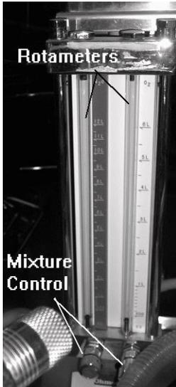
Rotameters are calibrated in cubic centimeters (cc) or milliliters (ml) of gas per minute. The amount of each gas entering the mixing board is controlled by needle valves at the base of each rotameter.
