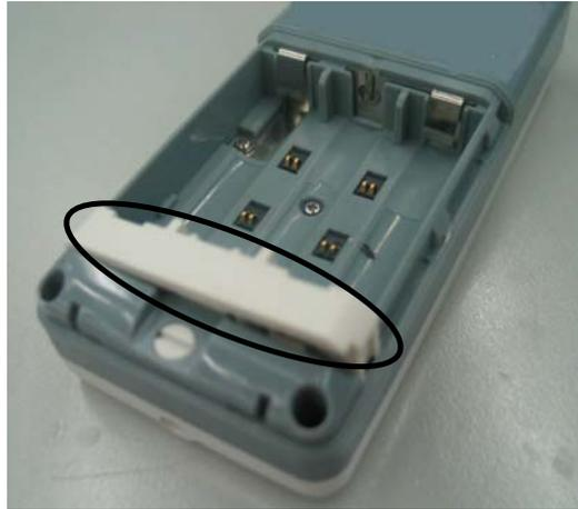
3. Unscrew 2 M2X6 crosshead screws and 3 PT2X8 tapping screws. Separate the front panel from the rear cover with your hands.
