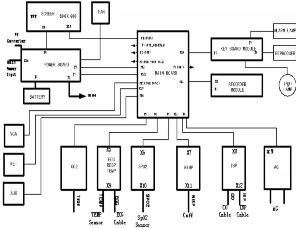
Figure 2-2 Functional structure of the DPM5
