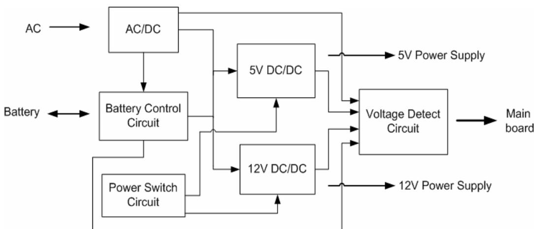
Figure 2-11 Working principle of the power PCB
