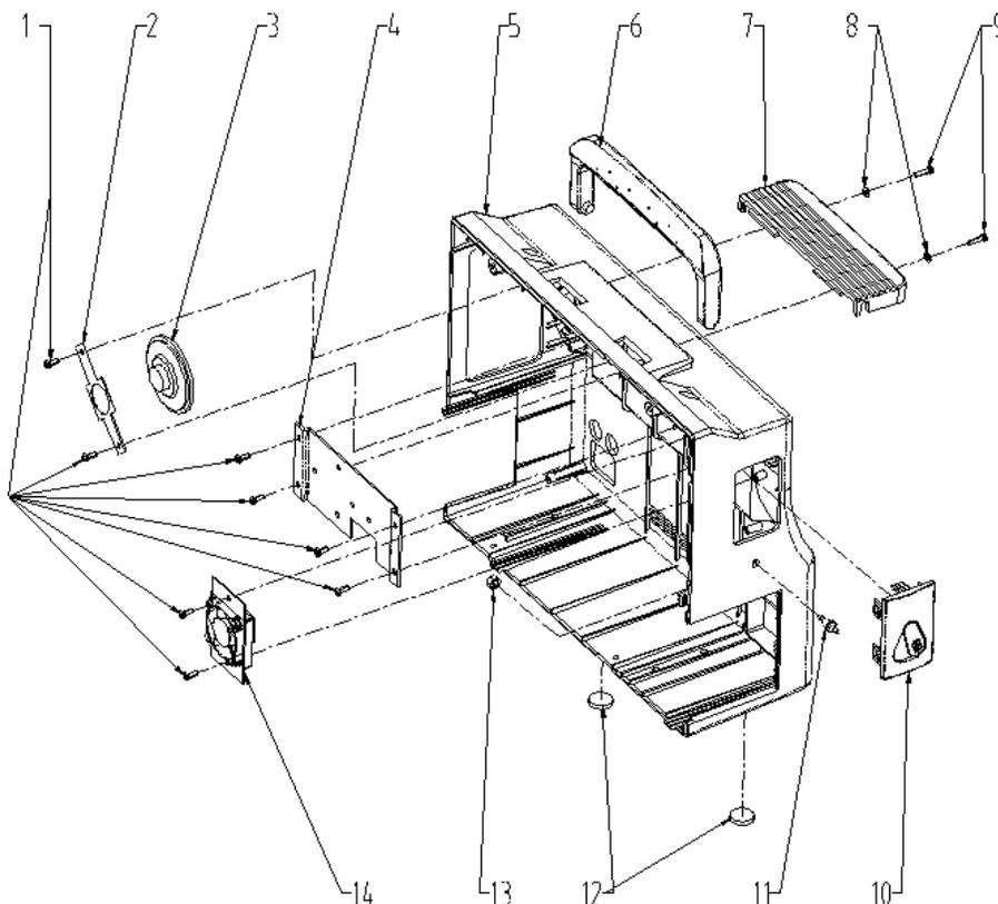
Figure 4-5 Back cover assembly (microstream CO<sub>2</sub>) (9201-30-35992)
