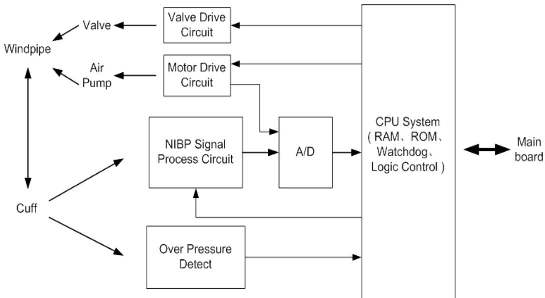
Figure 2-8 Working principle of the NIBP module
