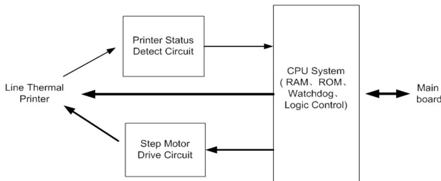
Figure 2-9 Working principle of the recorder module
