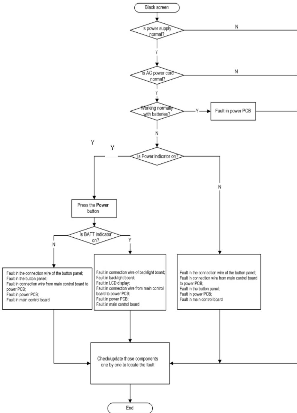
Figure 4-7 Location flow of faults causing black screen
