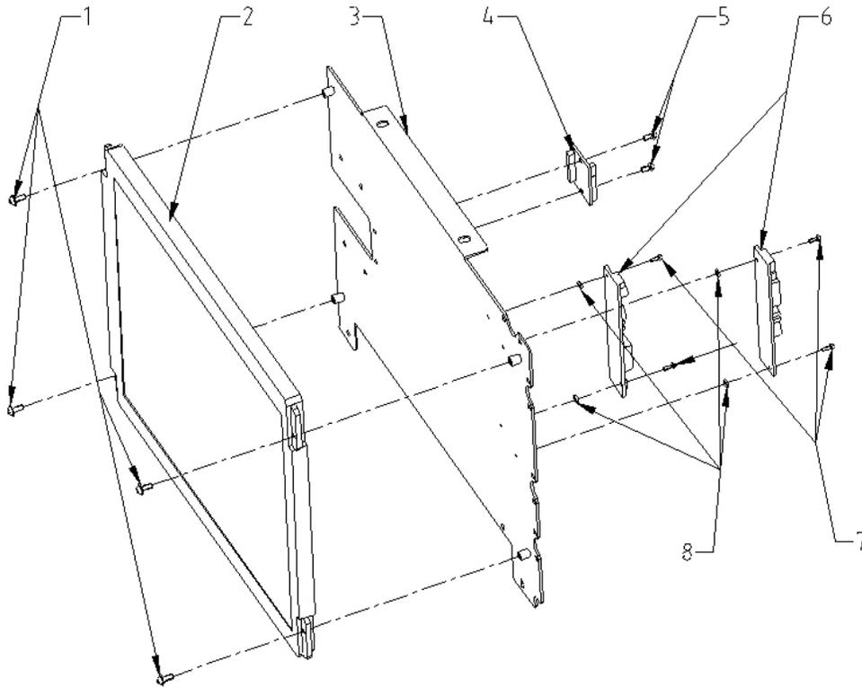
Figure 4-2 DPM5 display (TFT display) assembly
