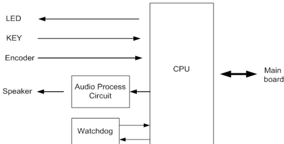
Figure 2-10 Working principle of the button panel
