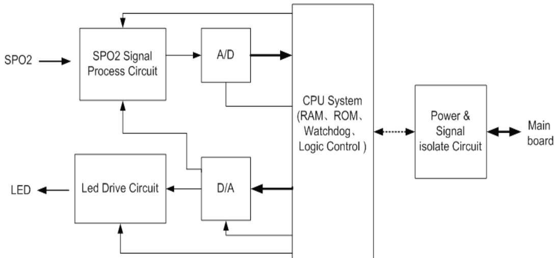
Figure2-7 Working principle of the SpO<sub>2</sub> module
