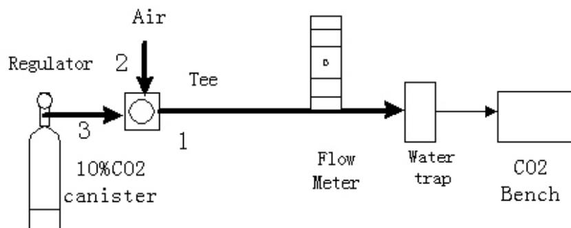
Figure 5-6 Sidestream test set up
