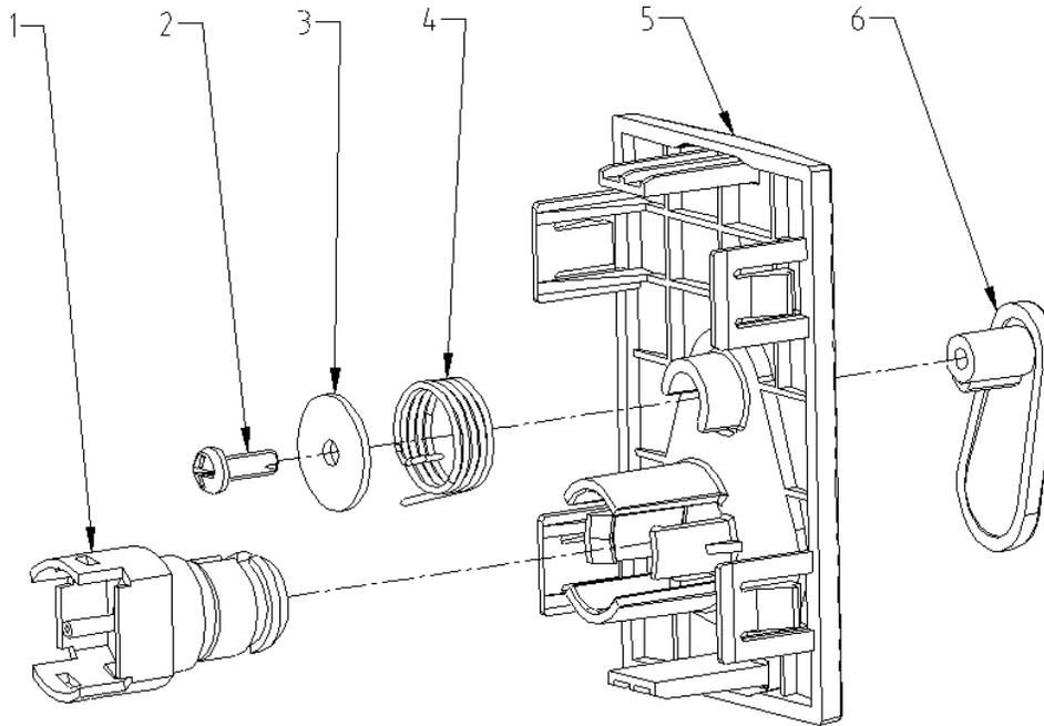
Figure 4-6 Microstream CO<sub>2</sub> assembly
