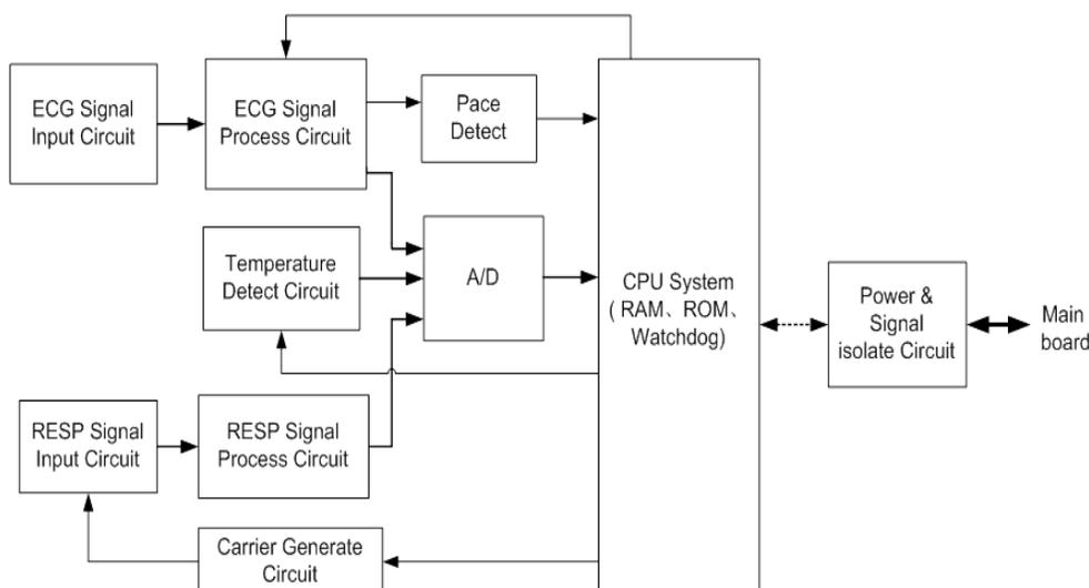
Figure 2-5 Working principle of the ECG/RESP/TEMP module
