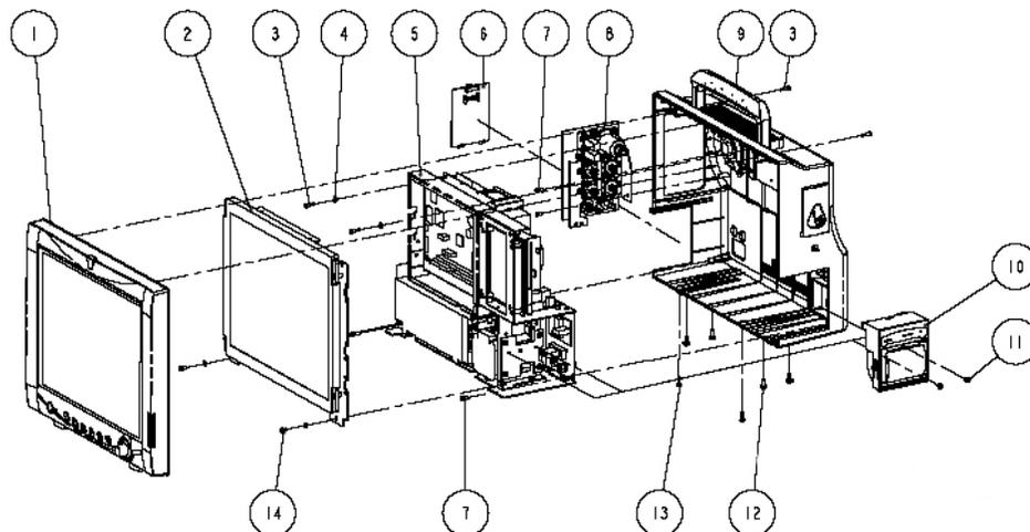
Figure 4-1 Exploded view of DPM5
