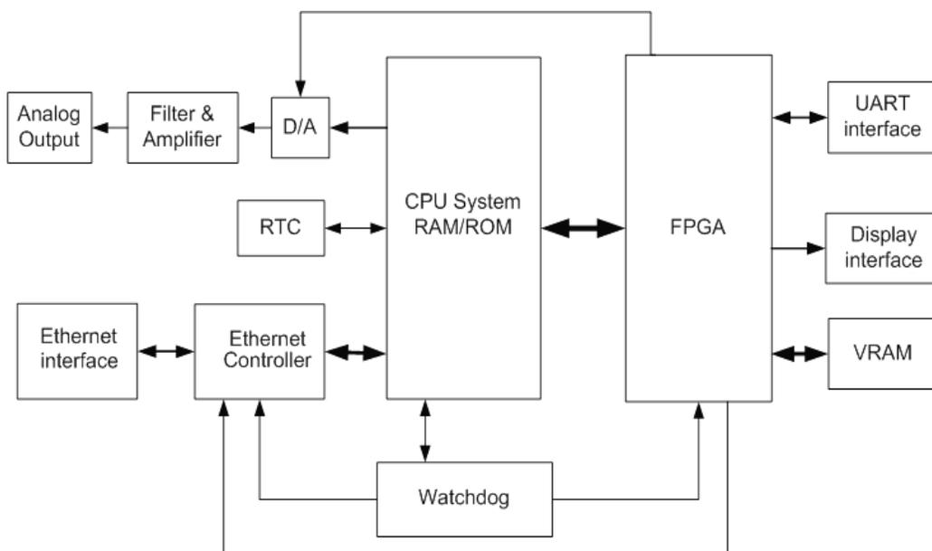
Figure 2-4 Working principle of the main board
