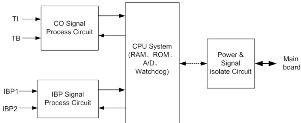
Figure 2-6 Working principle of the CO/IBP module
