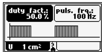
**Pulse [ms], period [ms]** – information about the length of the pulse and the period calculated for the set pulse frequency and duty factor.
