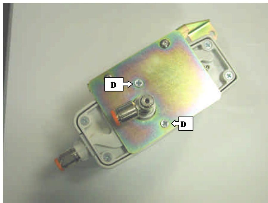
The suction controller can then be removed from its bracket by removing the two 'pozi-drive' screws (D).
