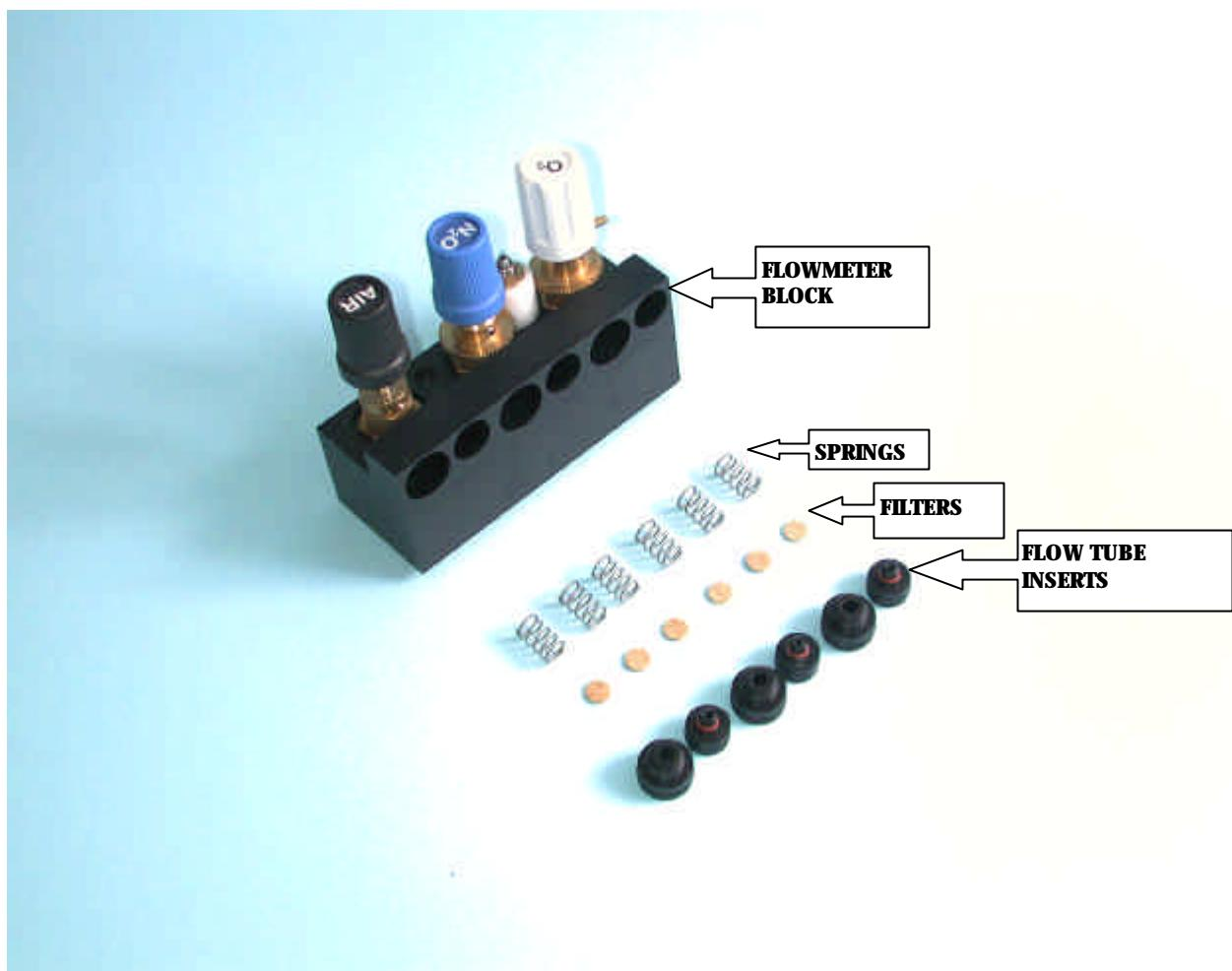
**Figure 15 Flow Block Showing Flow Tube Filters and Tube Lower inserts**
