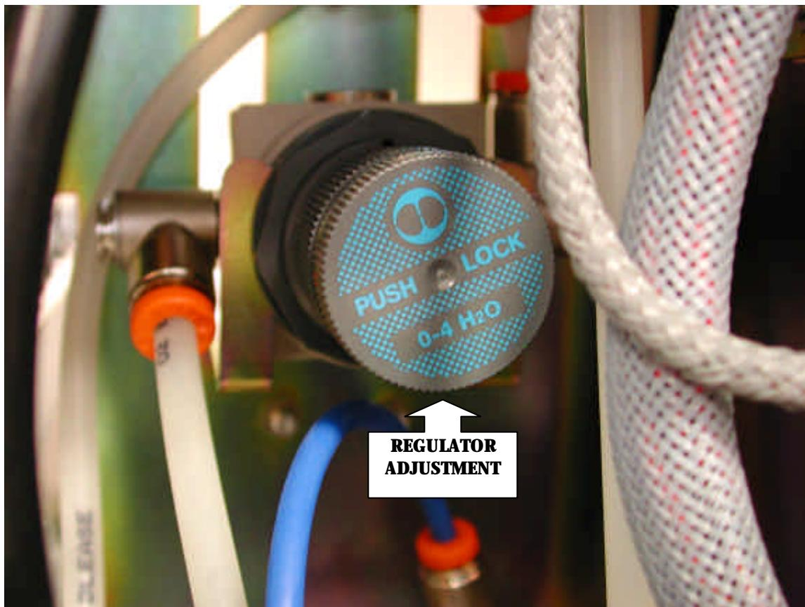
**Figure 19 Regulator Adjustment**
