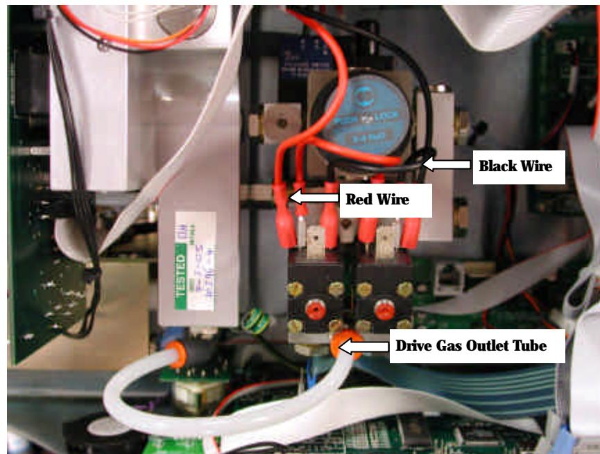
Disconnect the two wires (one red, one Black) from the flow control valves and the drive gas outlet tube.
