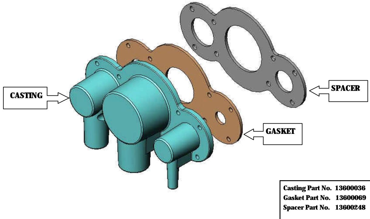
**Figure 30 Absorber Interface Manifold Assembly**
