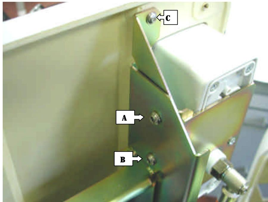
**Figure 36 Suction Controller Removal/ Replacement**
