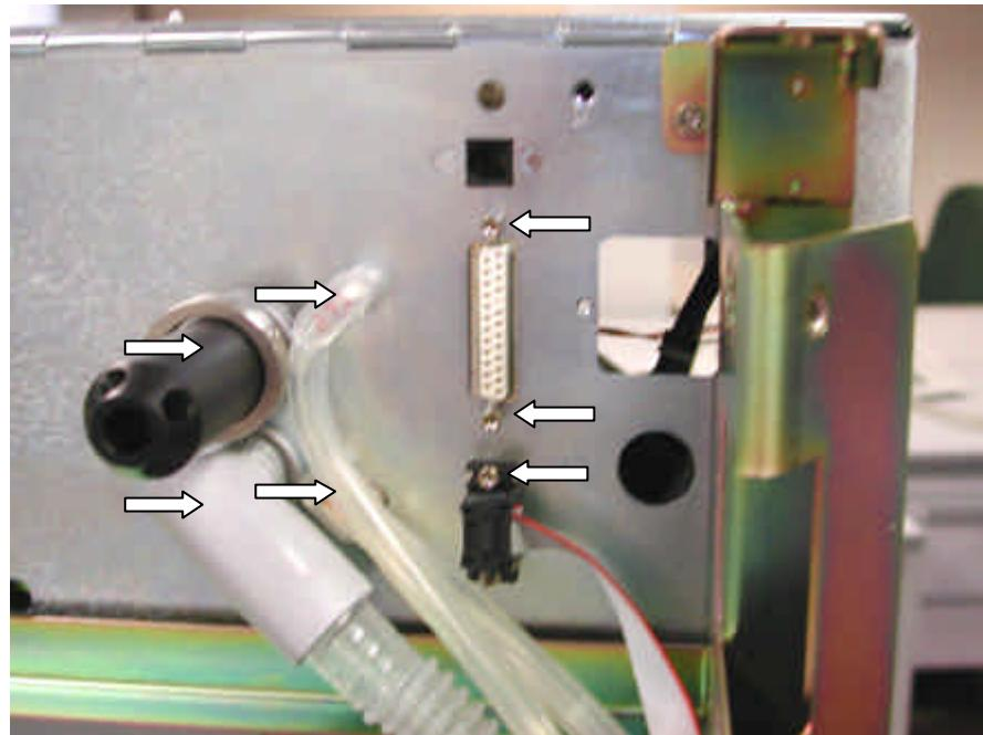
The Inspiratory block is now free to be removed. Fit the replacement Inspiratory block and then see section **3.3** for sensor calibration.
