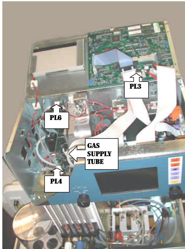
**Figure 39 Inside Ventilator**
