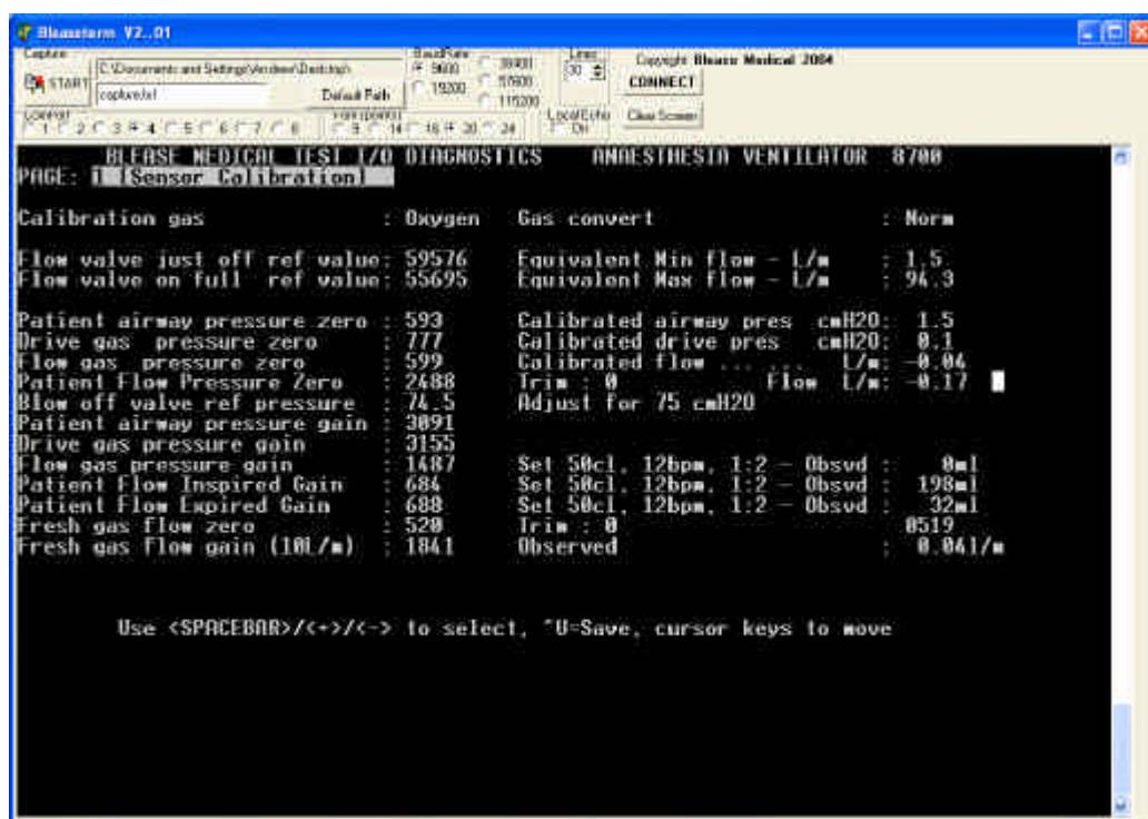
move the cursor down with the down arrow key on the keyboard to Patient airway pressure Zero
