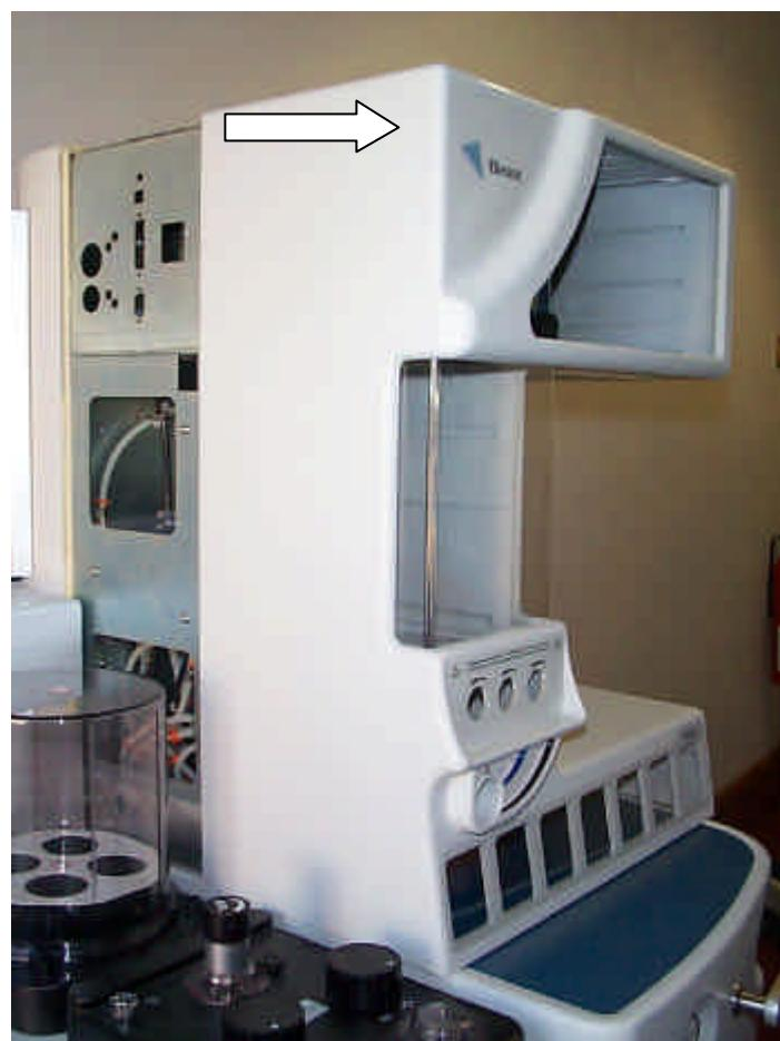
**Figure 6 Removal of Front Moulding**
