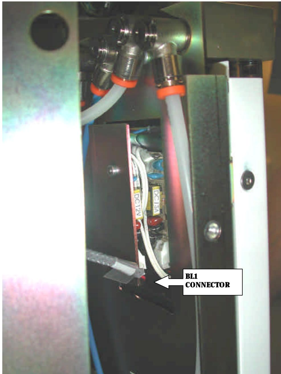
Mark the positions of the pipes entering the flow meter, and remove them from their fittings.
