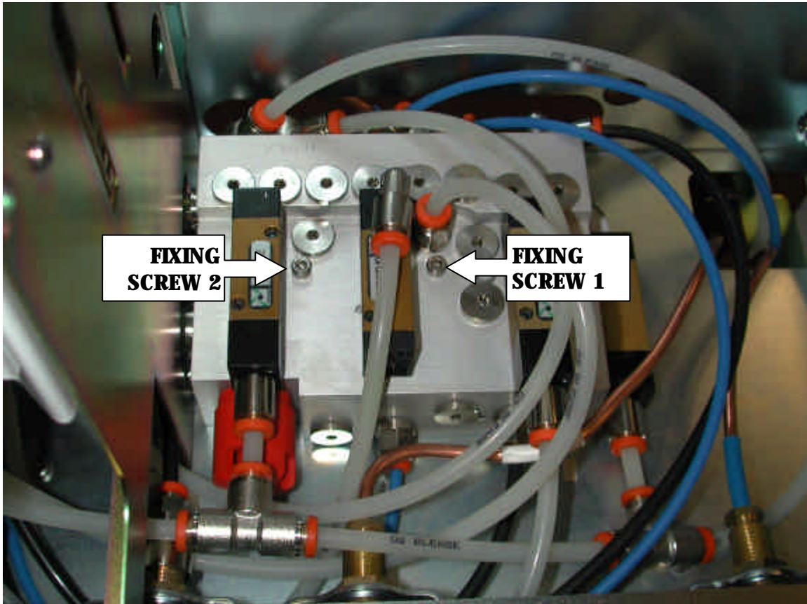
**Figure 25 Alarm Block Removal**
