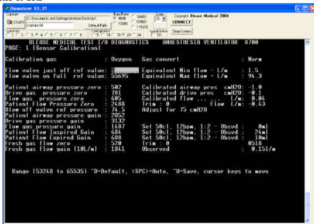
The valves will now be opening and closing. The system is attempting to find the lowest repeatable flow that it can deliver. Once this has been calculated the dots will be replaced with a new number.
