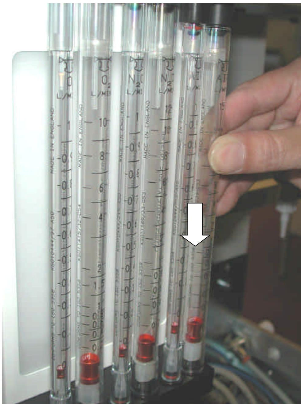
**Figure 17 Flow Tube Removal**
