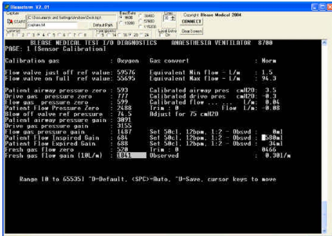
**Figure 48 Fresh Gas Flow Sensor Gain**
