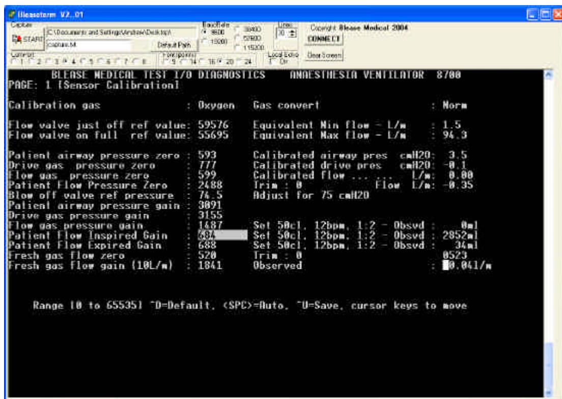
Check that the delivered volume on the volume measuring device is still 500+0/-30ml and press the space bar to record the value. (DO NOT MOVE THE CURSOR (8700 only)) The EtidalV value will go RED (on the third breath) and then back to BLACK. The cursor can now be moved to Patient Flow Expired Gain. (6700; does not measure inspired volume, therefore no setup procedure).
