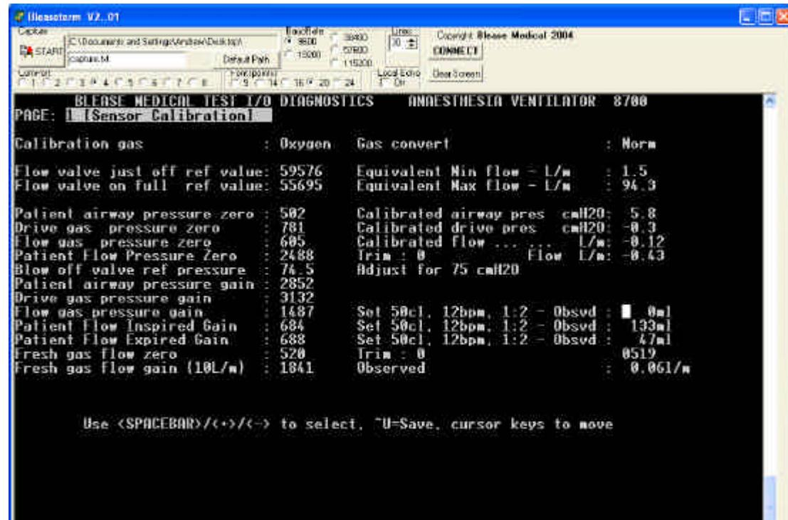
**Figure 41 BleasTerm Sensor Calibration**
