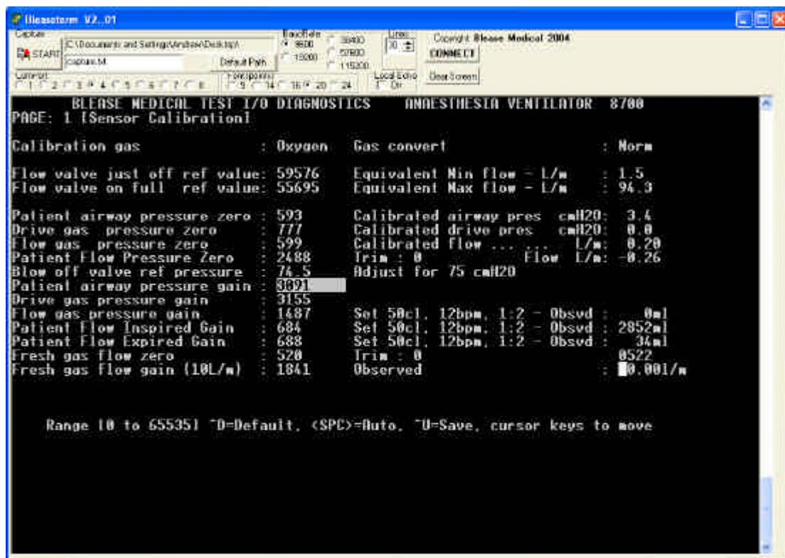
With the blow off pressure at 75 +/- 3 cmH2O press the space bar to record the value.
