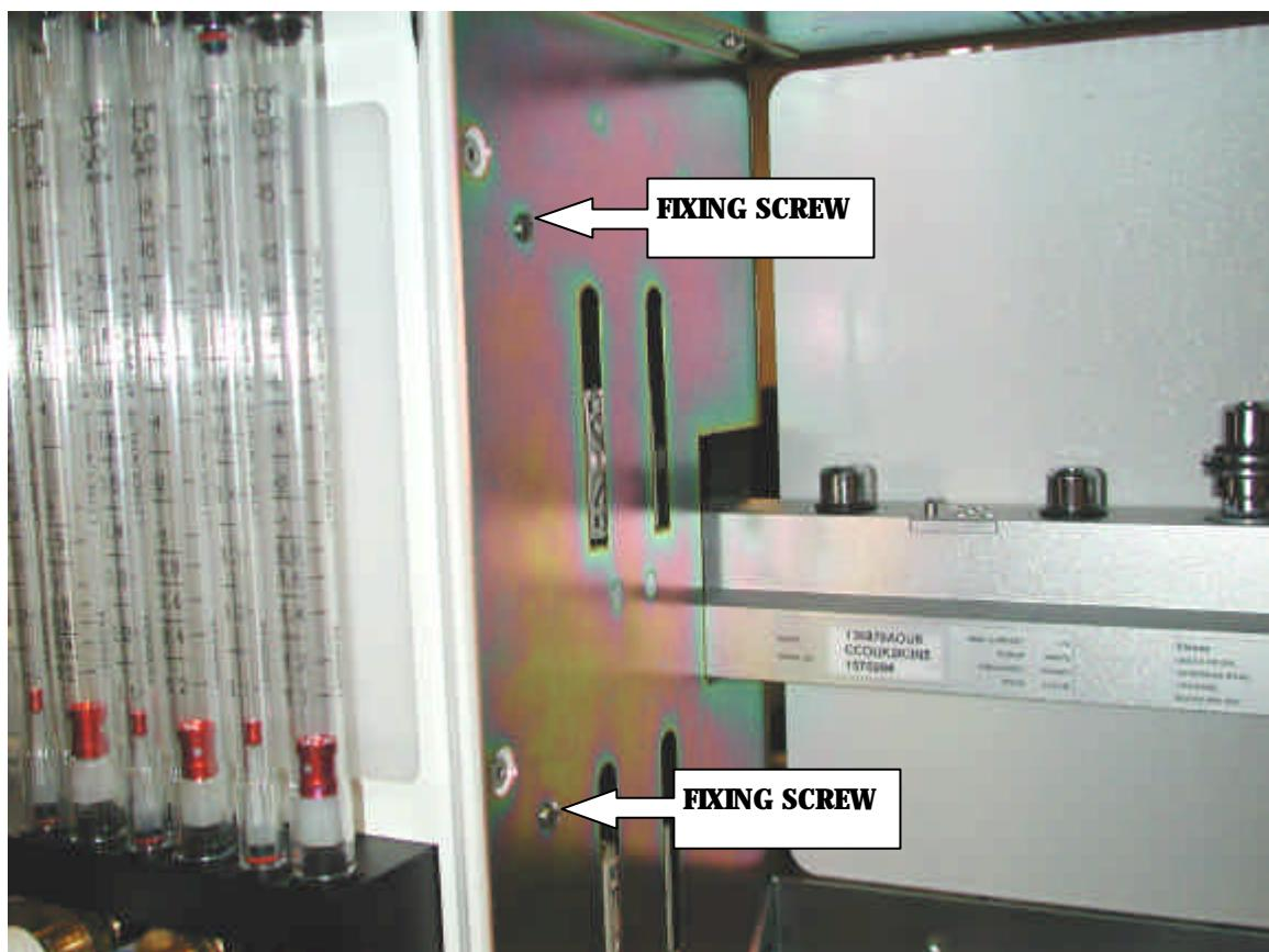
**Figure 28 Flow Meter Removal**
