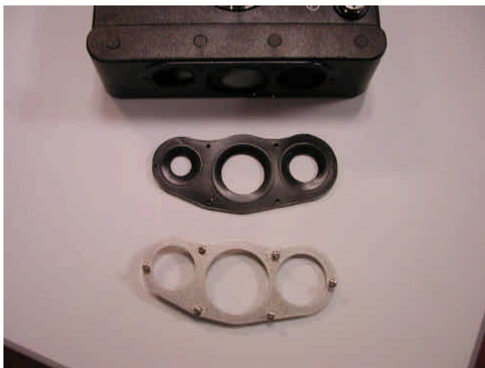
Gasket can them be removed, do not over tighten screws upon re-assembly.
