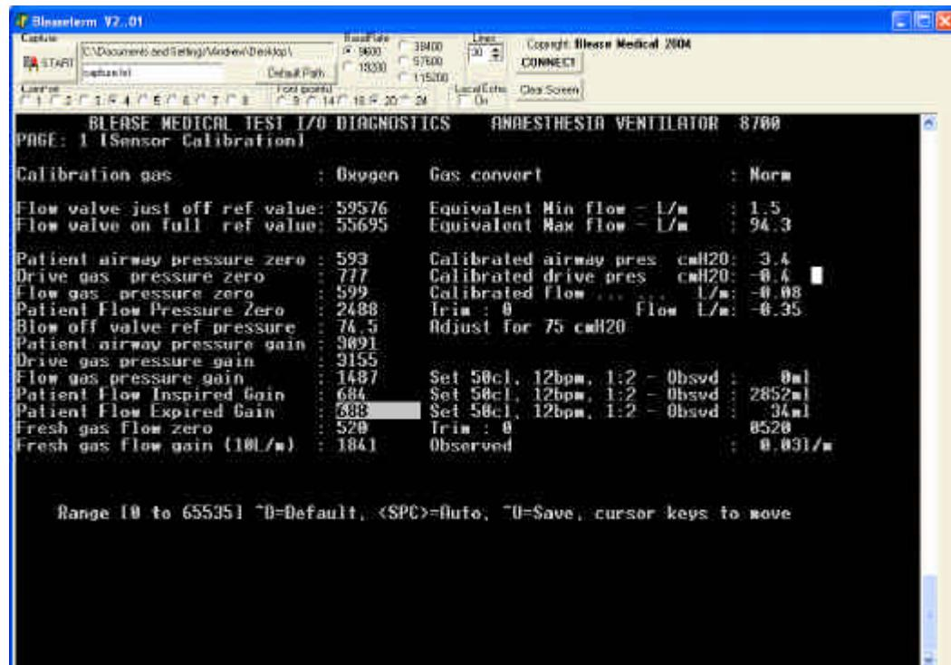
Check that the delivered volume on the volume measuring device is still 500+0/-30ml and press the space bar to record the value. Press the Ctrl and U keys to save.
