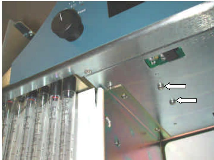
Move the assembly up and to the right so that access can be gained to the drive gas inlet tube. Remove this tube from the connector. The pressure switch is mounted on the back of the assembly remove the two wires that are connected to this. The assembly can now be removed from the ventilator.
