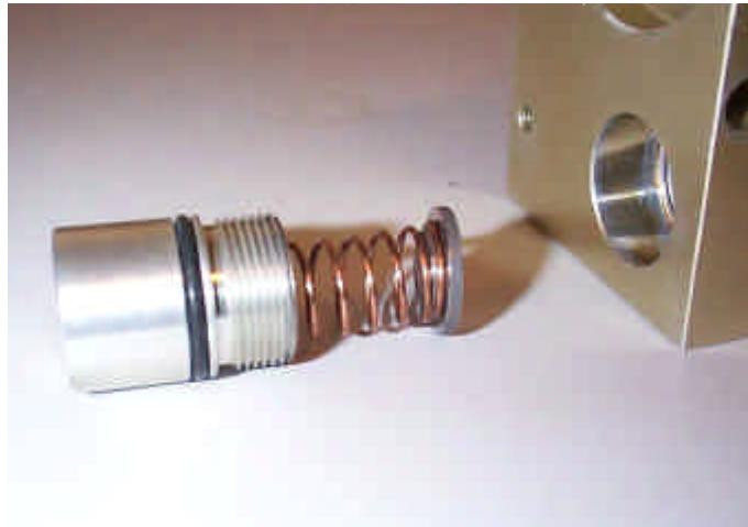
**Figure 27 Valve Adjuster and disc removed**
