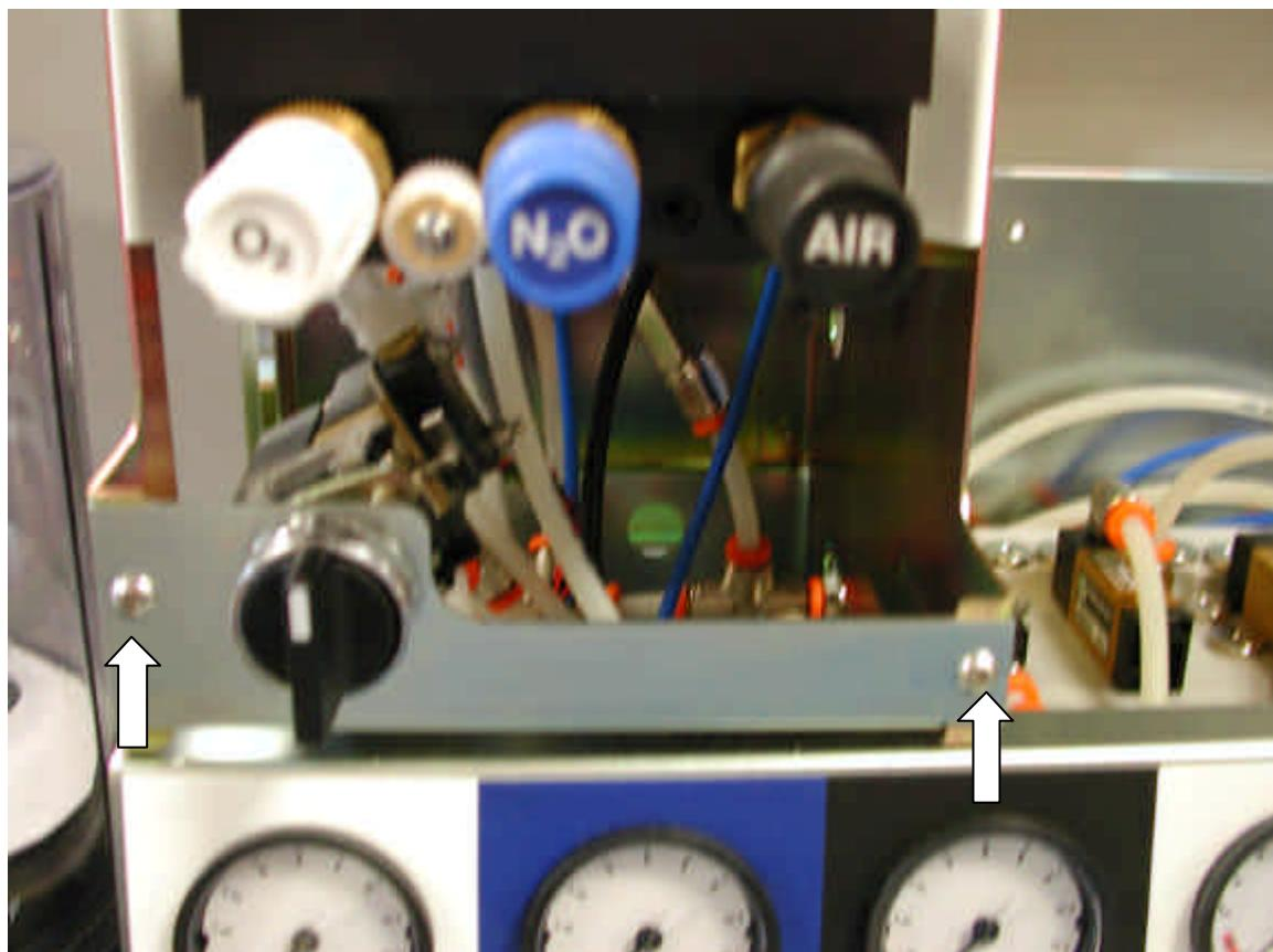
**Figure 29 On/Off Switch Removal**
