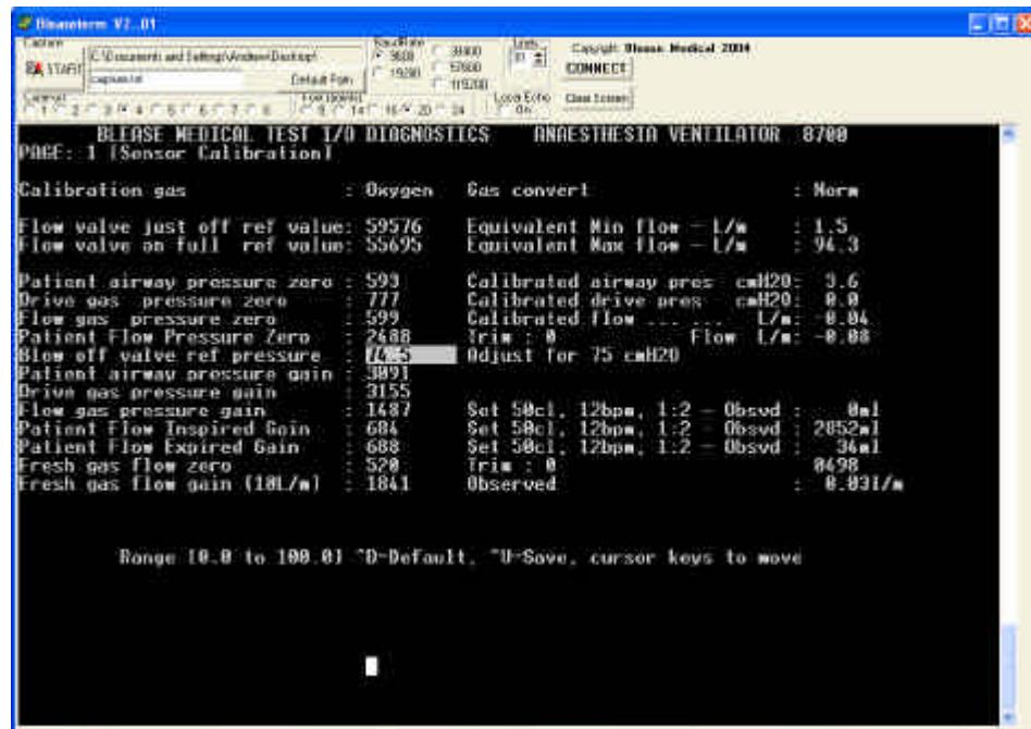
**Figure 46 Pressure Sensor Gain**
