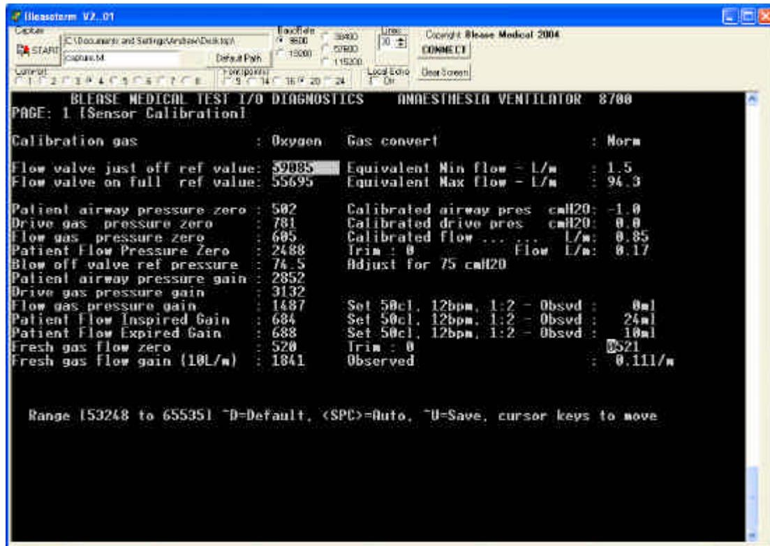
It is possible to move the cursor sideways to the Equivalent Min flow L/m and type the value recorded by the flow measuring device. (this information is not needed for the calibration. It is only a recording of the real world value).
