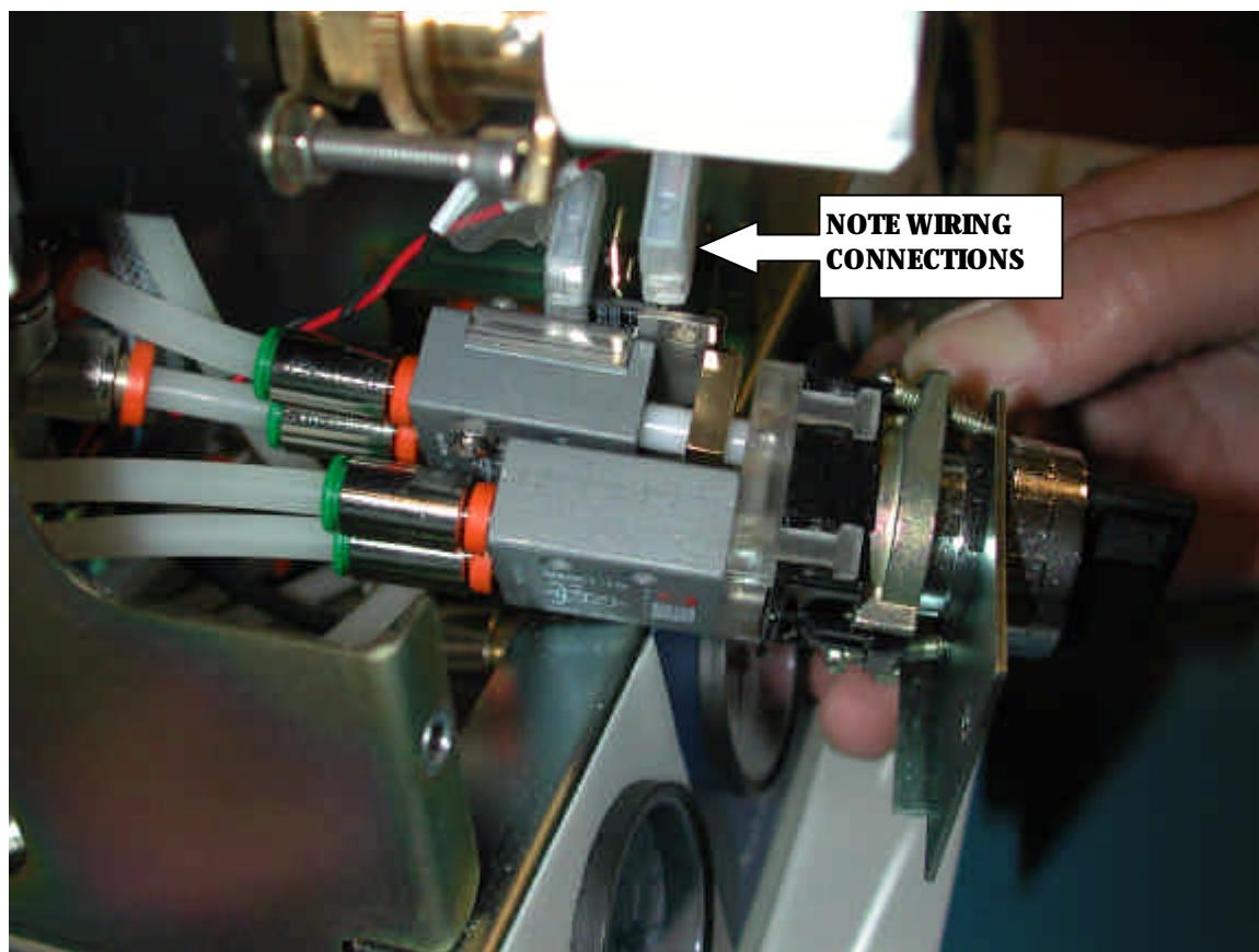
Carefully pull the switch assembly forward and disconnect the two wires from the switch noting their positions, then mark the relative positions of the four pipes entering the switch and remove them from their fittings.
