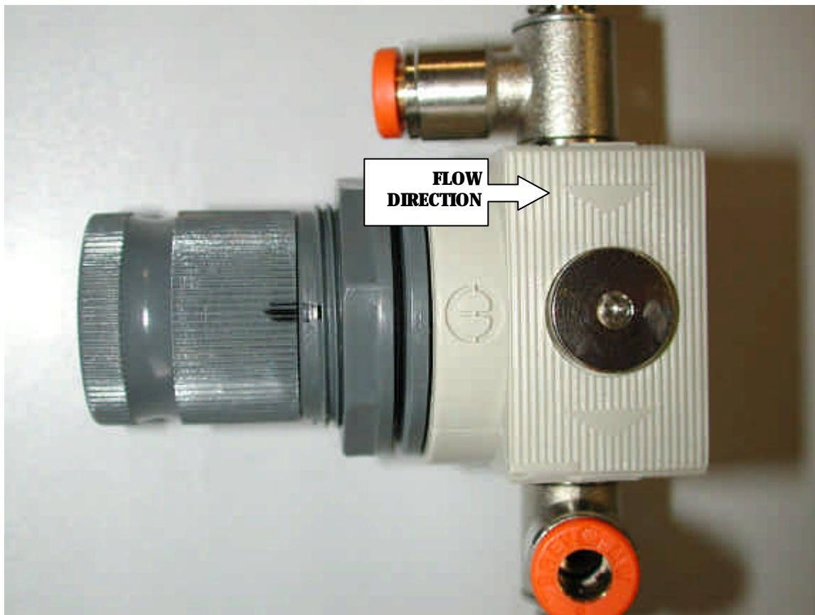
**Figure 21 Regulator Flow Direction**
