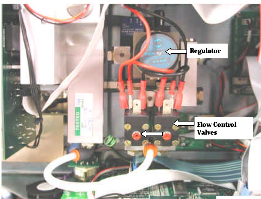
Gas Inlet Assembly Part No. 13700003
