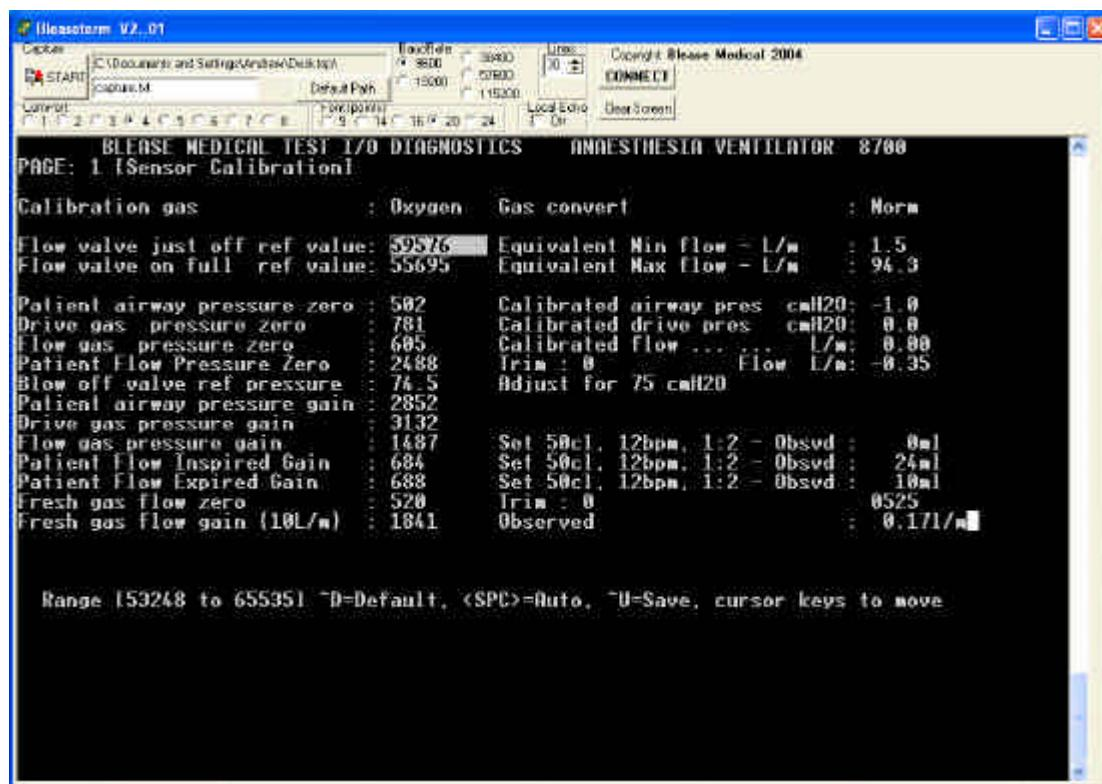
Press the space bar on the computer. The numbers in the cursor highlighted box will change to a series of dots
