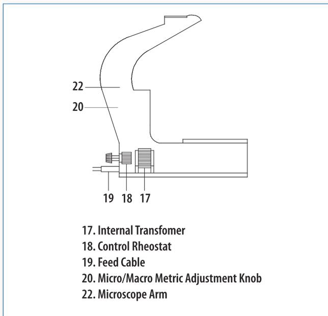
The microscope's body is designed to receive and support the components already described (binocular head, mechanical stage, condenser and revolving objective holder, other components such as the transformer and electrical/electronic elements of the microscope's lighting system).
