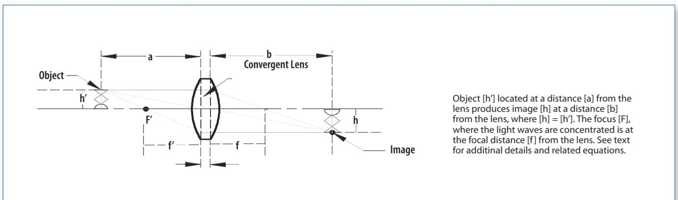
Object [ $h'$ ] located at a distance [ $a$ ] from the lens produces image [ $h$ ] at a distance [ $b$ ] from the lens, where [ $h$ ] = [ $h'$ ]. The focus [F], where the light waves are concentrated is at the focal distance [ $f$ ] from the lens. See text for additional details and related equations.
