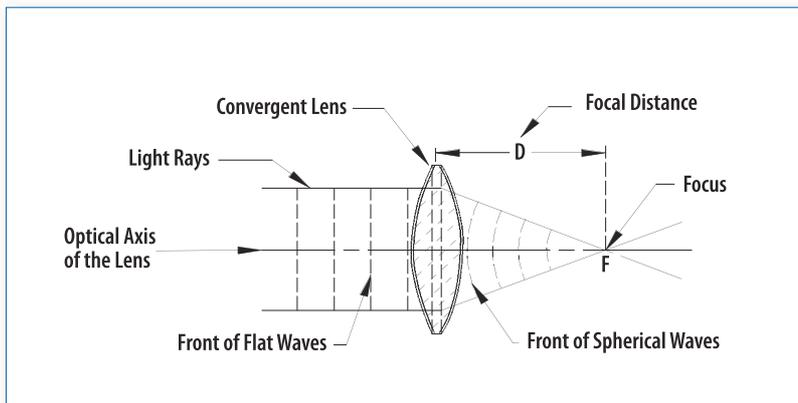
**Figure 42. Optics of the convergent lens**
