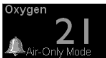
Figure 2-3. Air-Only Mode Message in Oxygen Parameter Box
