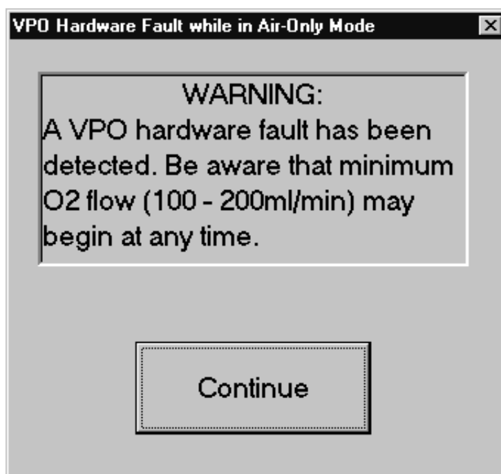
Figure 4-7. VPO Hardware Fault in Air-Only Mode
