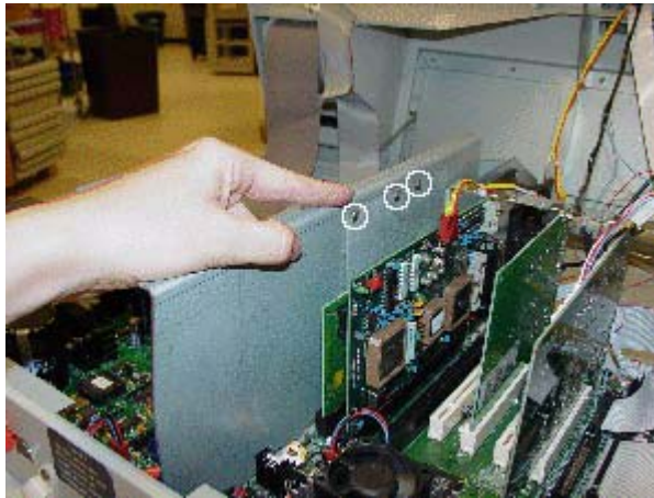
Figure 1-4. Slots for fan assembly screws
