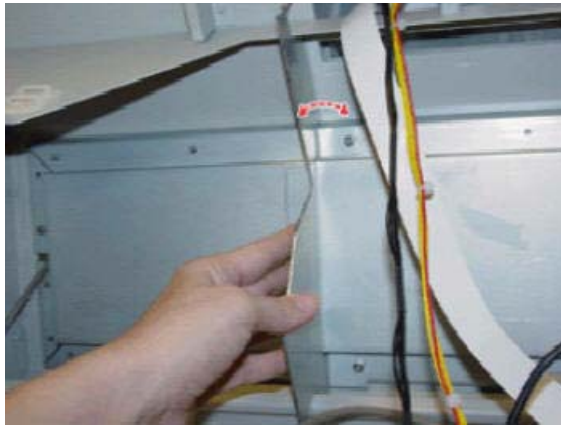
Figure 1-3. Installing the pressure plate
