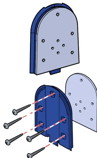
**8. Optional:** Attach the Cover plate to the Wall mount using the 5 M6x6 4 mm hexagon screws. And attach the pole clamp to the Cover plate using the 4 M5 screws which were removed during step 3 using a 4 mm hexagon key.
