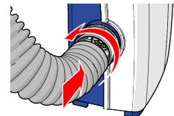
6. Pierce the hose with a sharp object at the location where the screw must be attached. Apply and tighten the screw that fixes the hose.
