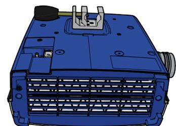
3. Remove the 4 M5 screws of the pole clamp using a 4 mm hexagon key and remove the pole clamp.
