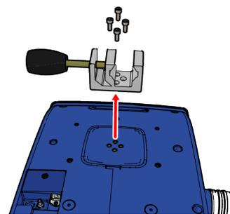
4. Attach the Cover at the 3 indicated locations using the first 3 of the 5 M4x16 3 mm hexagon screws with a maximum torque of  $1.5 \pm 0.2$  Nm or  $13.3 \pm 1.3$  in-lb.
