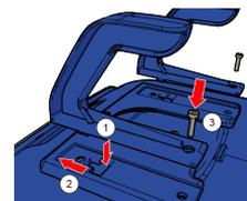
5. Optional: Click the Handles into the sliders of the Cover and tighten them at the 2 indicated locations using the last 2 of the 5 M4x16 3 mm hexagon screws.
