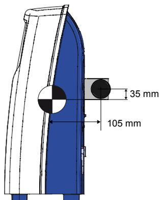
In the standard configuration, the device can be mounted to an IV pole or ISO rail using the universal clamp on the back of the device (see figures below). It is also possible to place the device on a table without reducing the air flow rate.
