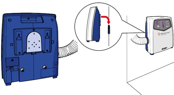
Mounting on a wall using the Wall mount.
