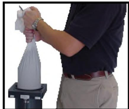
5. Slowly pull the exhausted resin pack over the side of the column while sliding it out of the column and into the plastic bag that it was shipped in. Return the exhausted resin pack to AmeriWater for regeneration.
