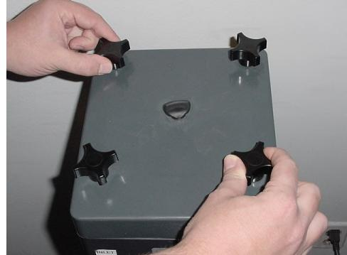
**CAUTION:** Failure to tighten the knobs completely may cause the cover plate to separate from the system when pressurized.
