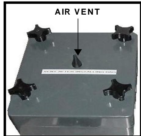
**NOTE:** Vent the system after every resin pack exchange to maximize the life and efficiency of the resin packs.
