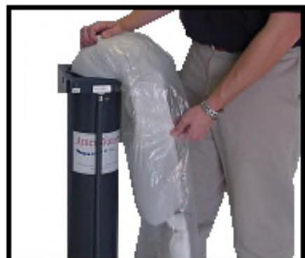
6. Remove the new resin pack from the shipping box and open the plastic bag being careful not to touch the resin pack. Stretch the resin pack over your arm to elongate the pack. Feed the pack into the column allowing it to slide out of the plastic bag. Save the plastic bag for the next resin pack exchange.
