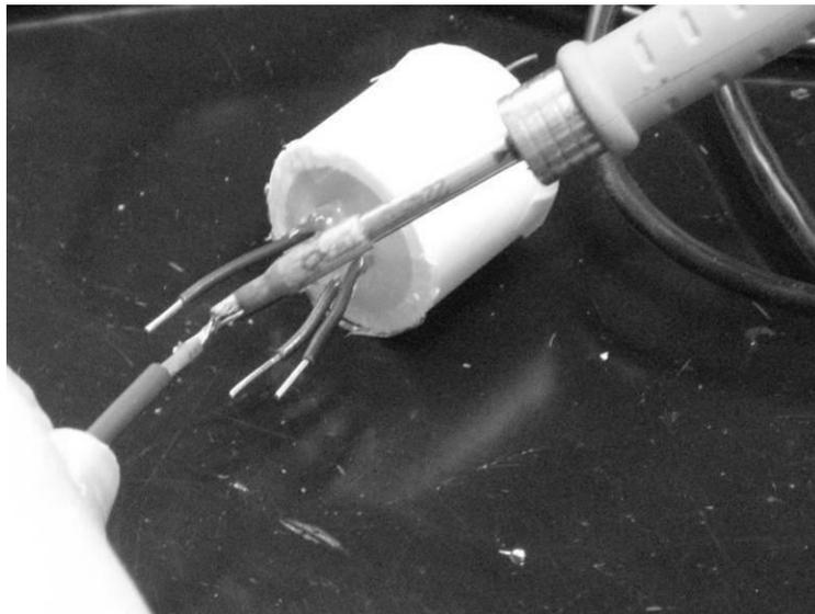
11. Insert new cable housing into the device. Insure that the fit is accurate.
