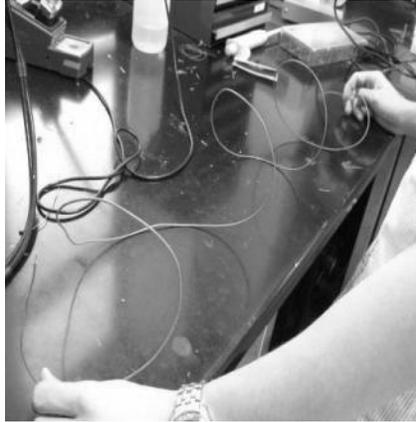
2. These wires will become the main cables of each lead. Strip both ends of each wire, and fit a piece of heat shrink tubing onto the wire.
