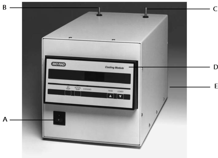
**Fig. 1: Cooling Module. A. Main power switch. B. FLOW IN port. C. FLOW OUT port. D. Control panel. E. Electrophoresis chamber internal temperature probe port and fuse (back of unit).**
