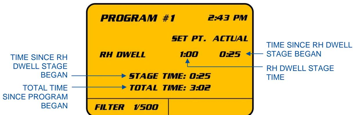
During the RH Dwell stage, the air is circulated inside the chamber. Additional humidity will not be added during this stage, so do **NOT** open the Main Door or the CA Chamber Door.
