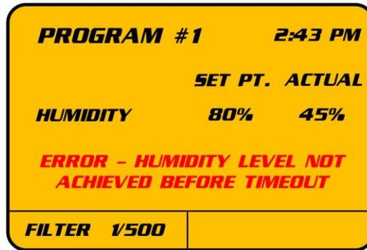
However, if the Fuming Chamber is used in an environment with very low humidity, the unit may require more time to reach the desired level of humidity. Before changing the default Humidify Timeout (35 min.), make sure no other problems exist within the unit. Contact Labconco Service Department at (800) 821-5525 or +1 (816) 333-8811 for troubleshooting assistance.
