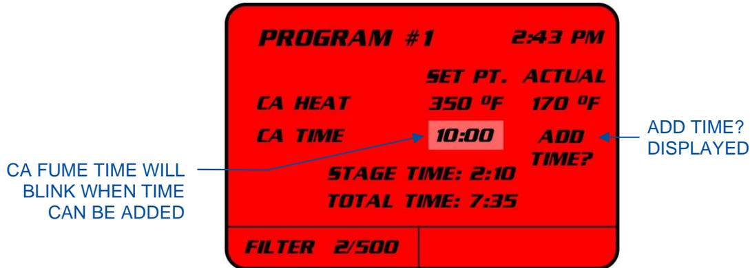
The **CA TIME** field will blink. If **[UP]** is not pressed within 5 seconds, the **ADD TIME?** text will disappear, and no change to the Fume Time will be made. Once the **ADD TIME?** text is displayed, each additional press of **[UP]** will add 30 seconds to the Fume Time.
