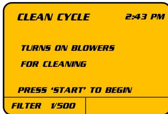
To start the Cleaning Cycle, press **[START]**. The blowers will turn on, even if the Main Door and/or CA Chamber Door are open. The blowers will stay on for 30 minutes, or until **[STOP]** is pressed.
