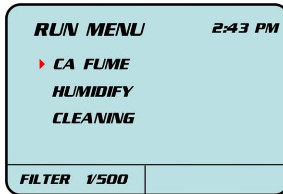
On the Run Menu screen (above), Select **CA FUME** by moving the red arrow to CA Fume menu option, and press **[OK]**. The Run > CA Fume Menu (see Fig. 6-8) displays all Program Parameters.
