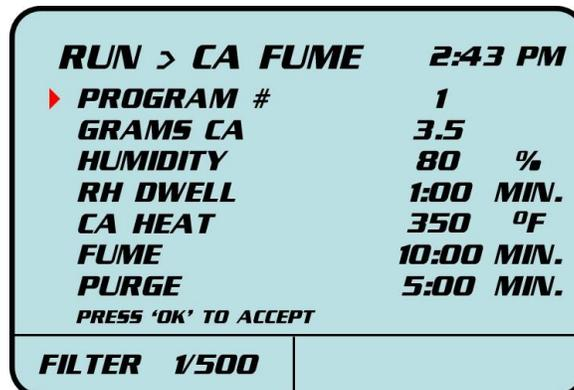
The Program Parameters (shown in Fig. 6-8) can be adjusted to desired levels within certain minimum and maximum values. Programs 1-3 are factory defaults for running common fuming cycles. The parameters can be modified in the first three programs, and a cycle ran; however, the modifications will not be saved, and will revert back to the factory default parameters. Programs 4-20 will save modifications to the program parameters. The modifications will be saved once a cycle has begun.
