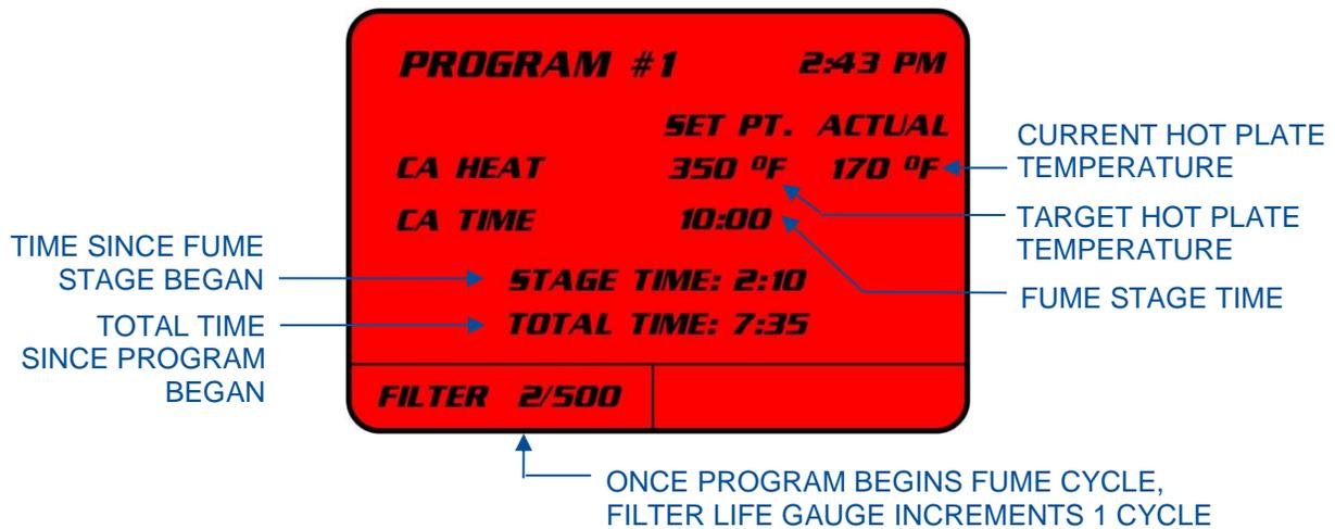
When the Fuming stage begins, both the Main Door and the CA Chamber Door will lock. They remain locked until the program is complete. This prevents opening the doors once CA fumes are present. If a power outage occurs while the doors are locked, they will remain locked. See [Section 10: Troubleshooting](#) for instructions to manually override the Main Door Lock so that evidence can be removed to protect it from over-fuming.
