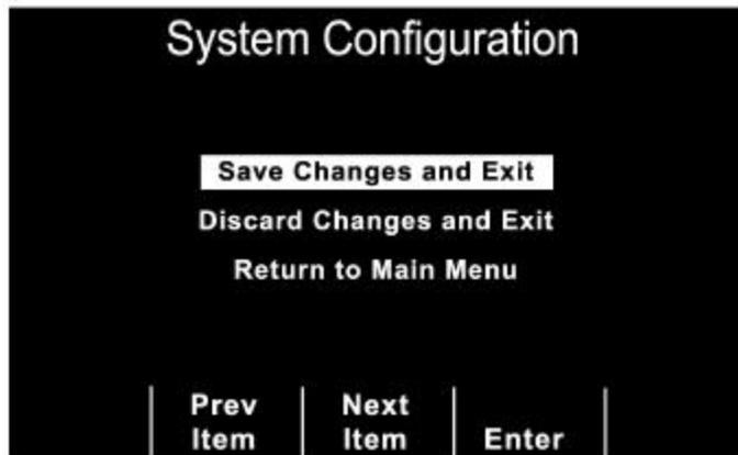
Press the **Prev Item** or **Next Item** softkey to scroll the highlight to the desired function. Press the **Enter** softkey to activate the selected function.
