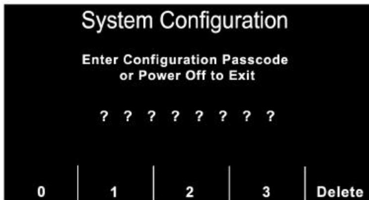
Users entering System Configuration for the first time must enter the default pass code (00000000) for System Configuration to continue.
