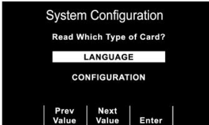
To move the highlighted area from LANGUAGE to CONFIGURATION and vice versa, press the **Prev Item** and **Next Item** softkeys. Press the **Enter** softkey to begin reading and storing the language settings or configuration settings from the user installed memory card.
