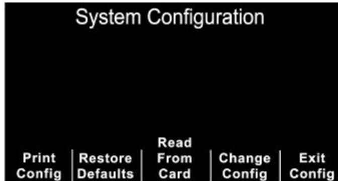
This menu provides the following five (5) softkey options: Print Config, Restore Defaults, Read From Card, Change Config, and Exit Config.
