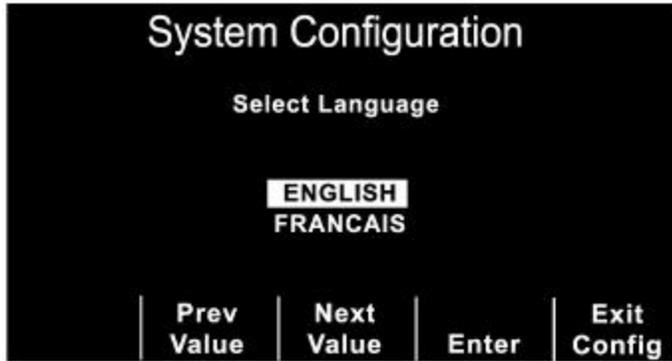
The first configurable option displayed after entering the correct pass code, is the Select Language menu. Press the **Prev Value** and **Next Value** softkeys to move the highlight from one language to the other.
