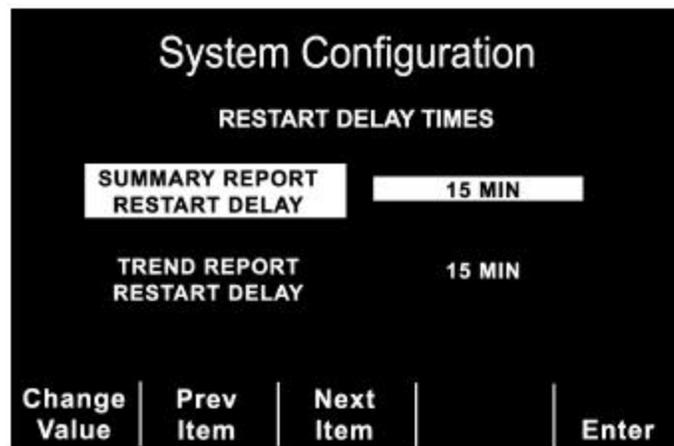
Pressing the **Change Value** softkey will scroll the highlight through the available delay times.
