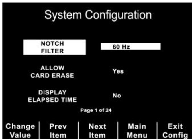
A description of each configurable feature is displayed in the left column of the option menu and that feature’s current setting is shown in the right column.
