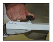
Position the adjustment knob of the Traction Unit Stand to the desired degree of the Pivot Plate.
