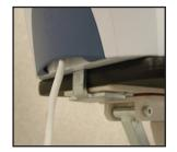
1. To secure the traction unit to the traction stand, loosen the clamp from the traction unit. Fit the traction unit to the stand and tighten the clamp up onto the stand.
