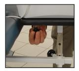
2. Attach the mounting screw onto the traction stand at the front of the unit. The mounting screw is provided with traction units only.
