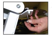
Place the two supplied 13 mm flat washers underneath the Pivot Plate.
