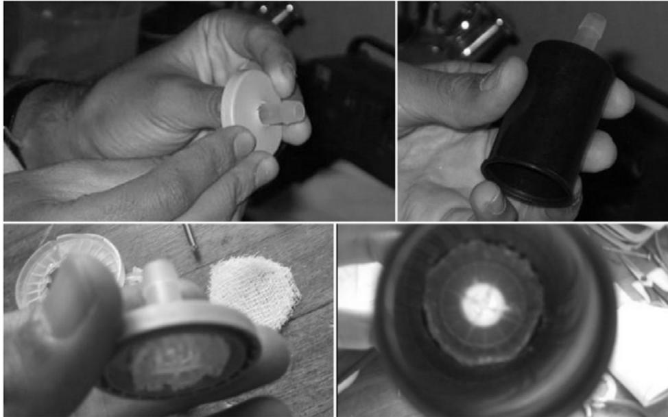
Using the gauze circles you cut out, make a stack of gauze, cotton, and gauze. Put the stack inside the film canister. Fill the entire canister. Use multiple stacks if needed.
