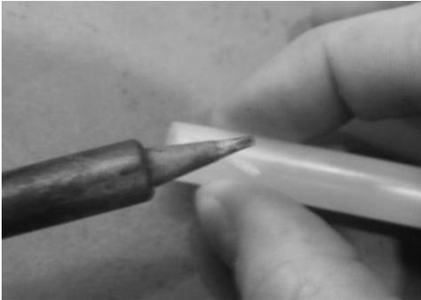
NEVER touch the heat source to the tube. Hold heat source safely near the tube.
