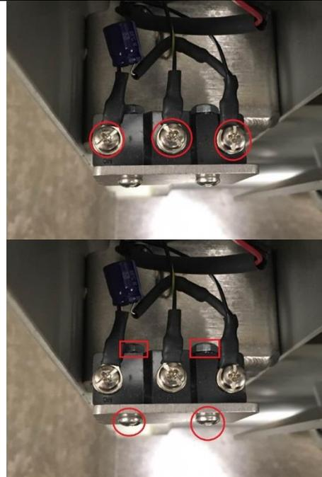
Use a 3/8" wrench to remove the nuts
