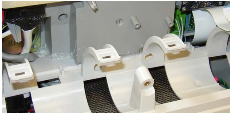
Figure 38: Front Body and Lower Frame Joint (with Correctly Applied Silicone)
