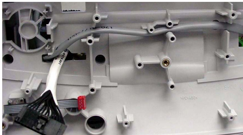
Figure 22: ECG Cable Route through Lower Frame
