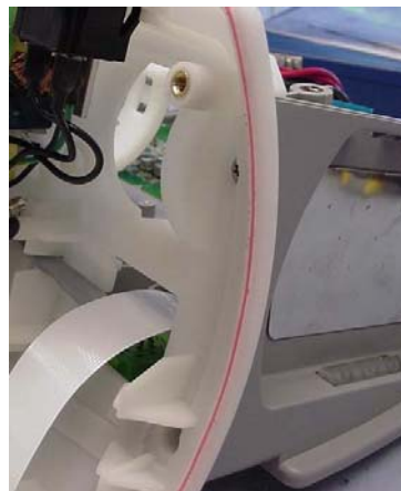
Figure 33: Tubing Properly Installed
