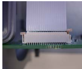
Figure 7: Bad: Jack Latch not Fully Engaged
