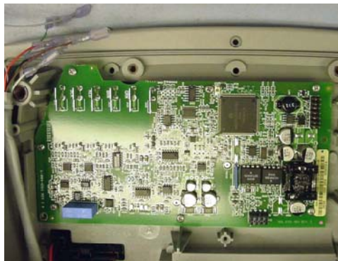
Figure 40: ECG Board Installed
