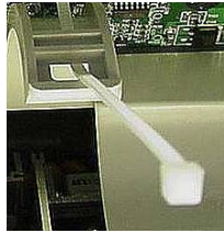
Figure 57: Tie Wrap Installation Detail
