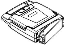
2. Push the latched end of the battery firmly into the AED, as shown in the drawing, until the battery snaps into place. The exposed side of the battery should be flush with the outside of the AED case.
