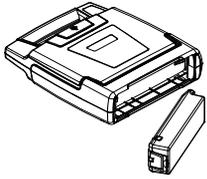
1. With the label on the battery facing the AED battery compartment, insert the battery as shown in the drawing.
