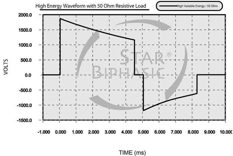
The Biphasic Truncated Exponential (BTE) waveform uses variable energy. The actual energy delivered will vary with the patient's impedance and the device will deliver a shock when impedance is between 25-180 Ohms. Energy will be delivered at up to three different levels referred to as ultra-low variable energy, low variable energy, and high variable energy as shown in the waveform tables on the following pages.
