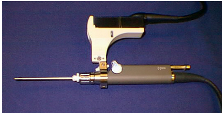
Figure 4-39. Debrider Attachment to Linvatec High Speed Shaver Handpiece
