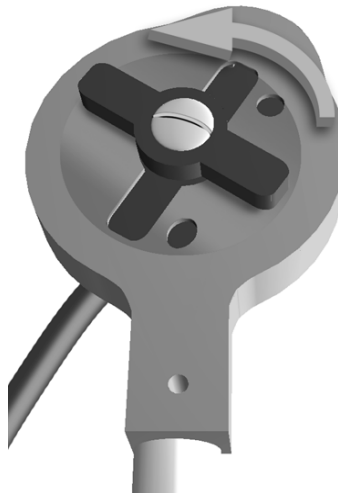
Figure 4-29. Rotate Transmitter Latch to Secure Transmitter
