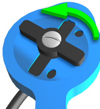
Figure 6-2. Removing Transmitter from Attachment Arm
