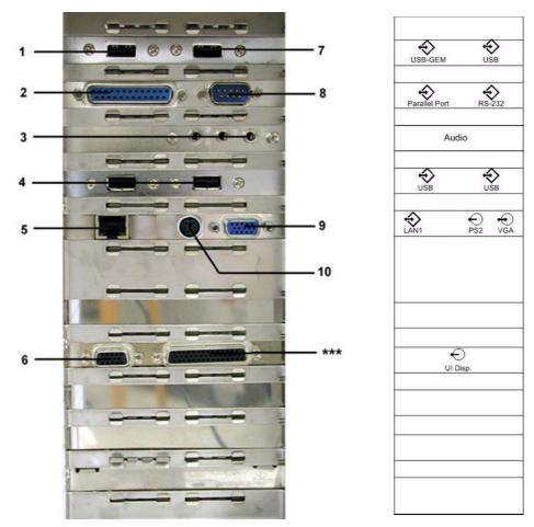
Figure 5-18 Connectors on PC-part of the GEF
