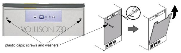
Figure 3-5 Remove rear cover plate
