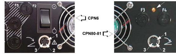
Figure 7-2 Diagnostic LED's and corresponding voltage check points
