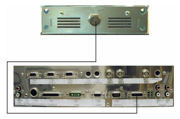
Figure 3-8 ECG Connection Scheme
