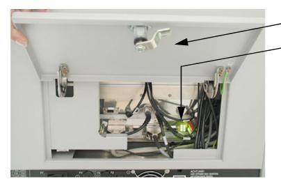
Open the locking, flap the service lid on the back of theVoluson® 730Expert upwards, and check the status of the Diagnostic LED's.
