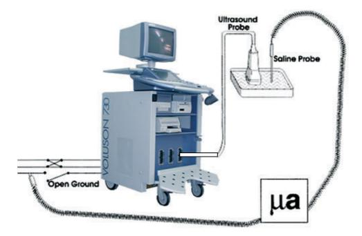
Figure 10-6 Check Without Probe Adapter
