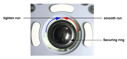
Figure 6-5 Trackball - Securing Ring
