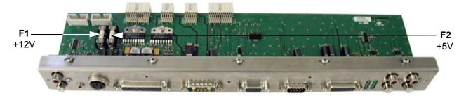
Figure 5-28 fuses for disk drives
