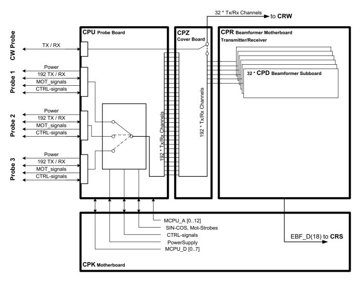
Figure 5-11 CPU + Beamformer (CPR)
