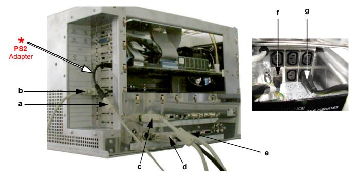
Figure 7-11 cable- minimum configuration (e.g., IBASE PC-Board installed)
