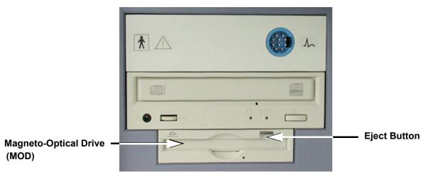
Figure 4-16 Magneto-Optical Drive
