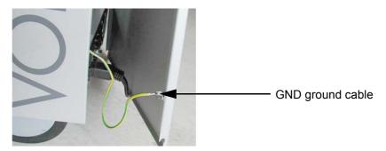
Figure 3-6 GND ground-cable
