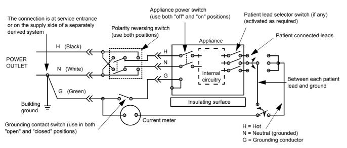
Figure 10-4 Test Circuit for Measuring Non-Isolated Patient Leads
