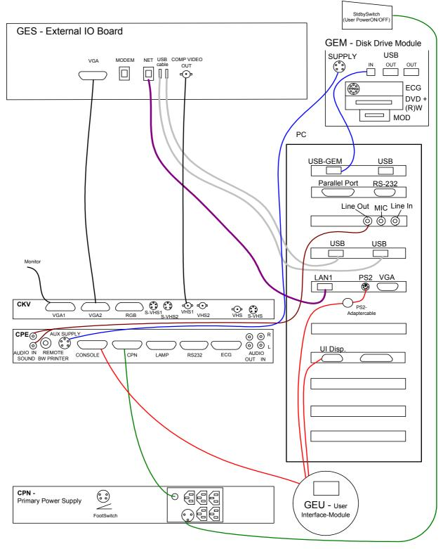
Figure 5-16 Internal I/O
