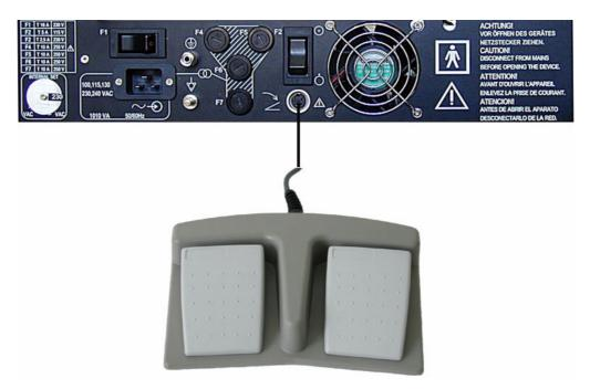
Figure 3-7 Foot Switch Connection Scheme
