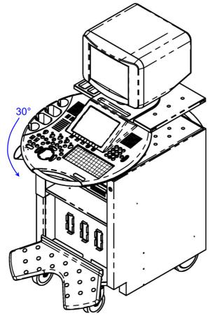
Figure 5-30 Top Console Positioning
