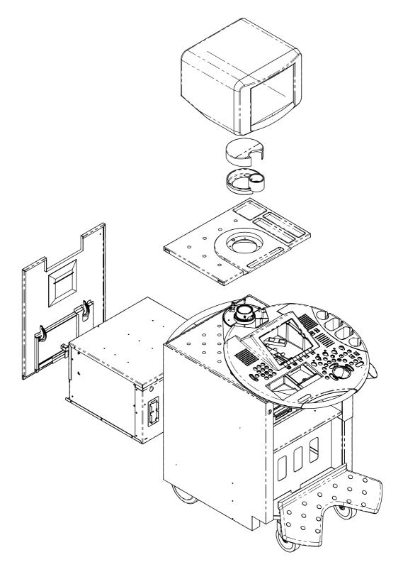
Figure 5-32 Assembly Drawing Voluson® 730Expert
