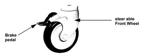
Figure 4-38 Front Wheel with Brake
