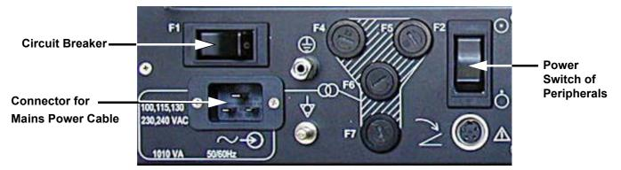
Figure 3-22 Circuit Breaker at rear of system with CPN6 installed
