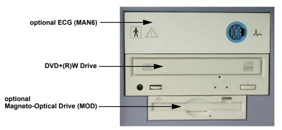
Figure 5-23 GEM incl. optional MOD and ECG
