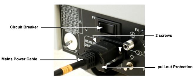
Figure 4-1 Circuit Breaker, Protection and Power Cable on back of Voluson® 730Expert
