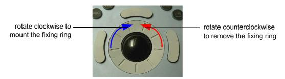
Figure 8-29 Trackball with top fixation ring
