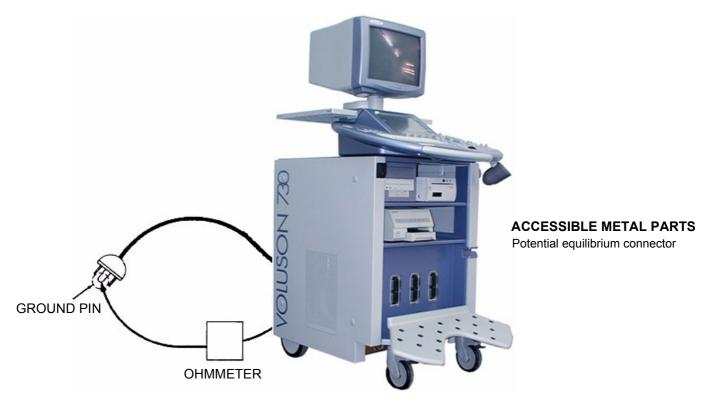
Figure 10-2 Ground Continuity Test
