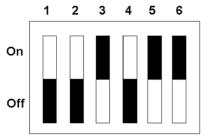
Set DIP Switches on back of the VCR as shown:
