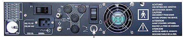
Footswitch connected to Power Supply-Box (below Main Electronic-Box)
