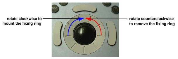
Figure 6-4 Trackball with fixing ring
