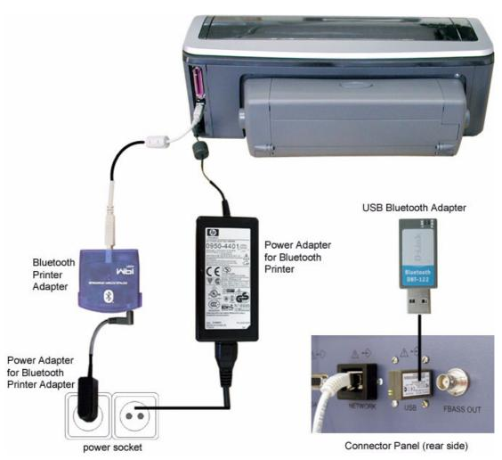
Figure 3-16 HP Bluetooth Printer - Connection Scheme
