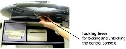
Figure 6-3 Locking Lever under Control Console
