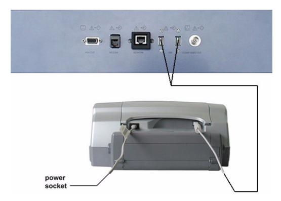
Figure 3-14 Line Printer Connection Scheme
