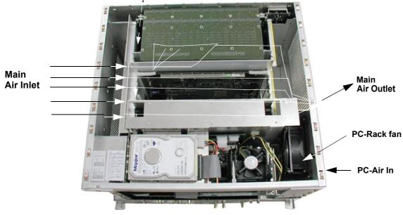
Figure 5-34 Air Flow Control
