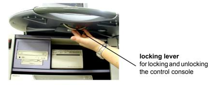
Figure 4-37 locking lever under Control Console
