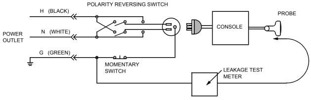
Figure 10-5 Set Up for Probe Leakage Current
