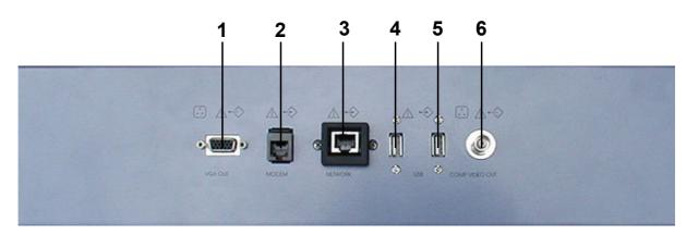
Figure 5-22 External I/O Panel Connectors
