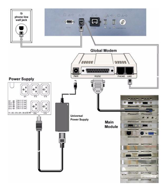
Figure 3-9 Global Modem Connection Scheme
