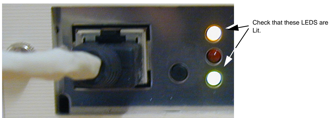
Figure 4-18 Link LED and 100 Megabit Detector LEDs at the rear of the Networks Printer
