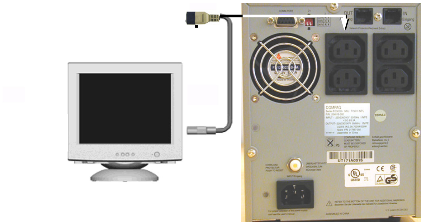
Figure 3-17 Monitor power connection at UPS rear (International version shown)
