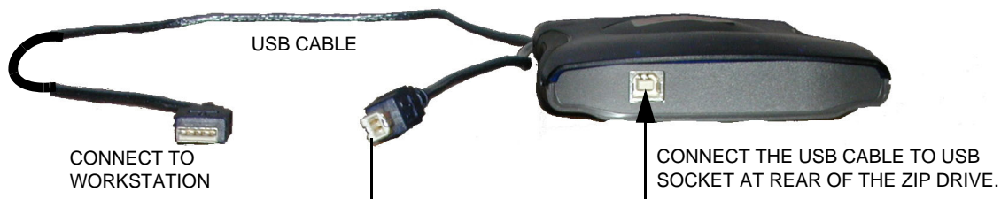
Figure 3-49 USB Connection between workstation and ZIP
