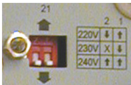
Figure 3-21 Voltage configuration DIP switches
