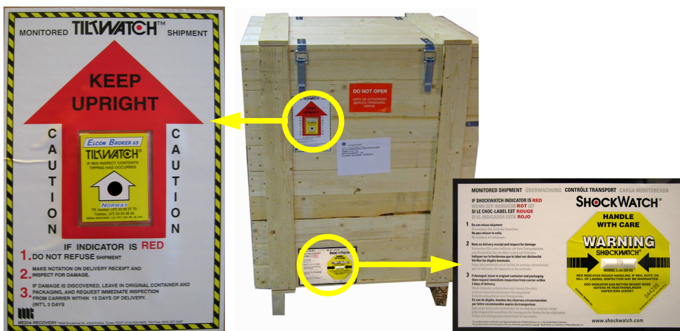
Figure 3-2 Tilt & Shock indicators's position on one side of transportation box
