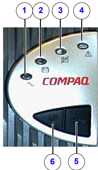
Figure 4-14 UPS front panel LED display and controls
