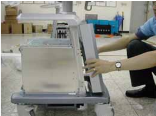
Figure 8-90 Removal of front cover
