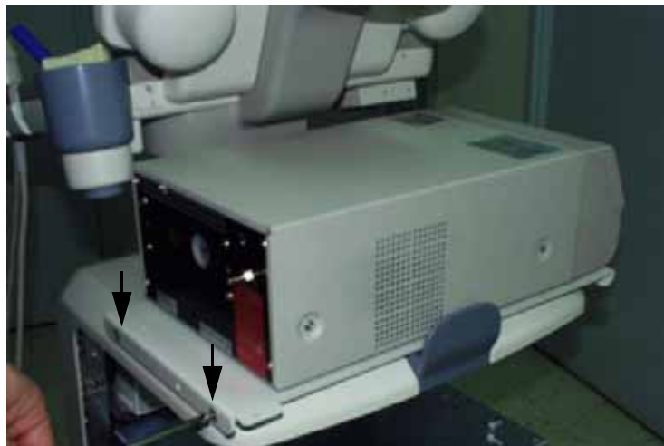
Figure 8-303 Printer VCR DVD Fixture installation top
