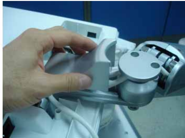
Figure 8-234 Removing the Fold cover
