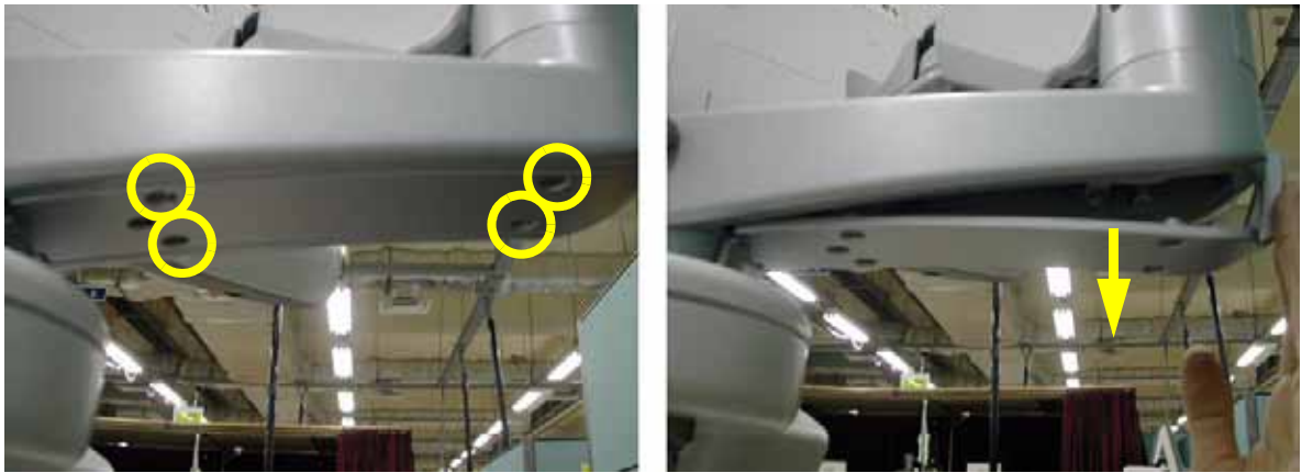
Figure 8-25 Removing the Arm bottom cover
