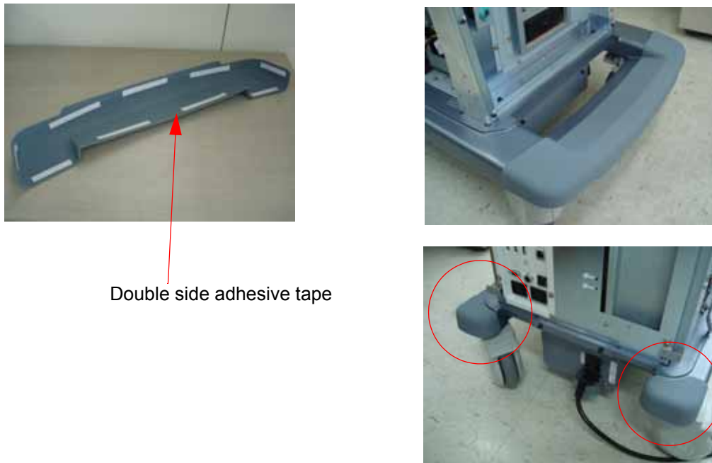
Figure 8-337 Protect Cover Installation
