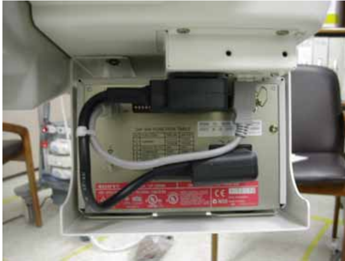
Figure 8-288 BW Printer Fixture Keyboard installation
