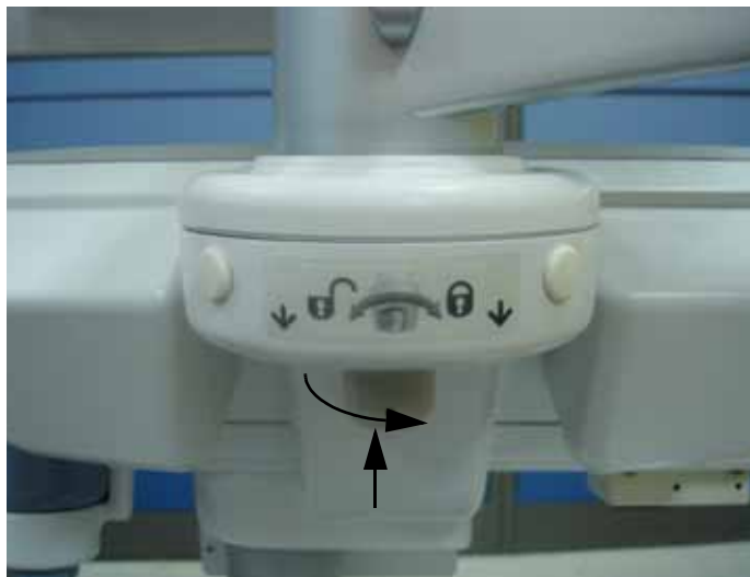
Figure 6-3 Locking the Flexible LCD arm
