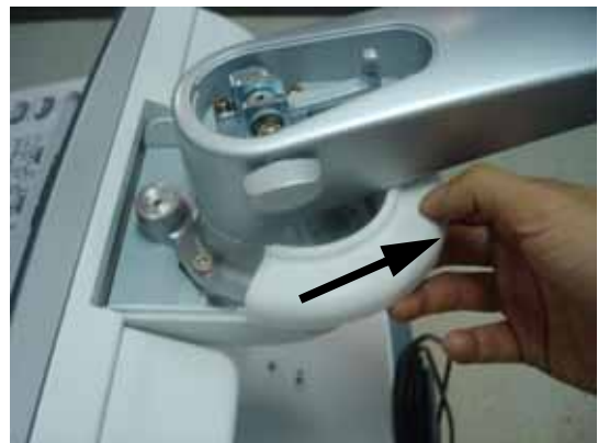
Figure 8-31 Unscrewing 3 screws and removing the neck front cover & neck rear cover
