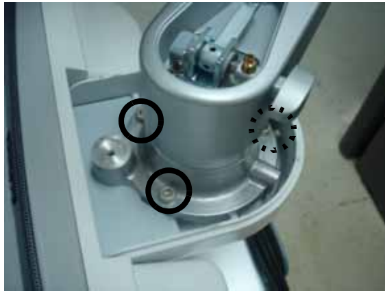
Figure 8-246 Separating the neck pipe
