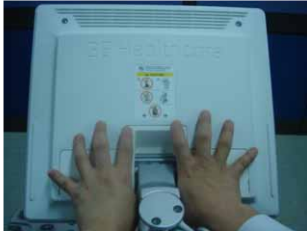
Figure 8-1 Removing the 17" LCD cable cover
