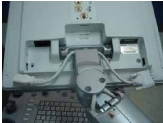
Figure 8-14 Removing the LCD Cable Cover
