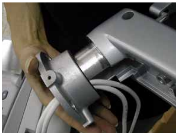
Figure 8-252 Inserting the flexible arm
