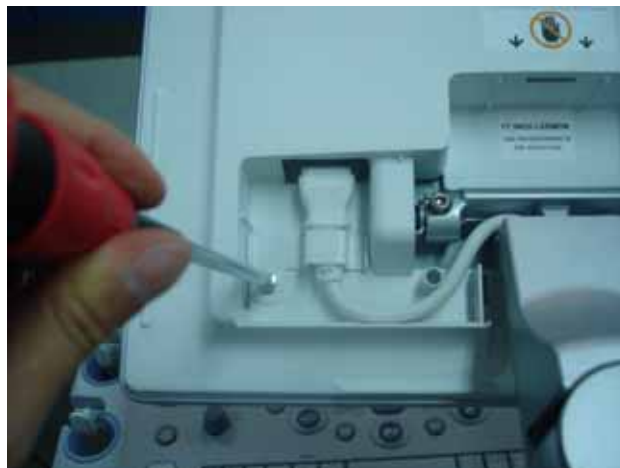
Figure 8-18 Removing the power cord bracket
