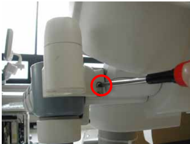
Figure 8-283 Cable Arm Hook installation
