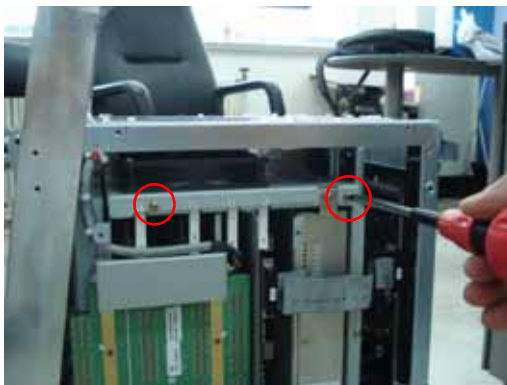
Figure 8-132 Pull out the nest fan
