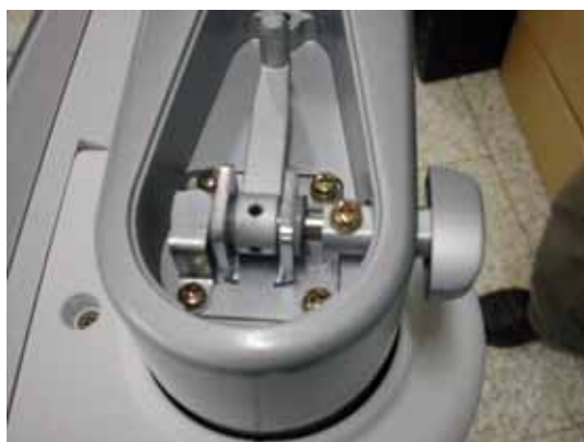
Figure 8-55 Assembling the Lock Knob
