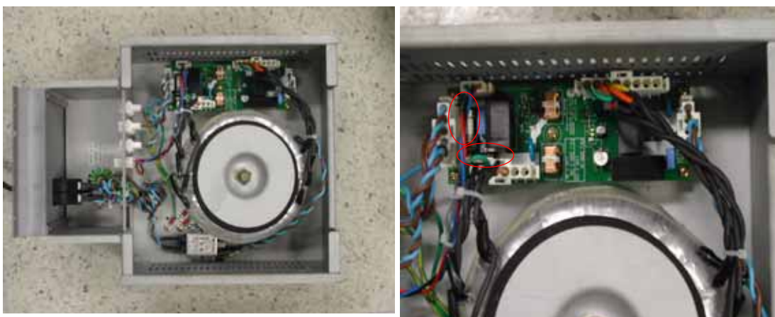
Figure 8-146 FUSE in Transbox(AP950) assy
