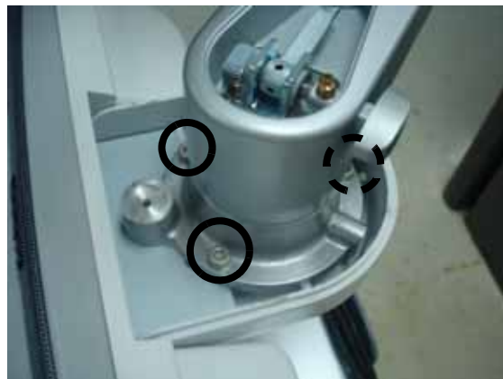
Figure 8-32 Separating the neck pipe
