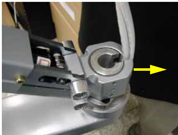
Figure 8-29 Pulling out power cable & DVI cable
