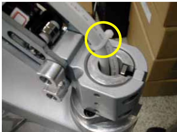
Figure 8-261 Tying the cables
