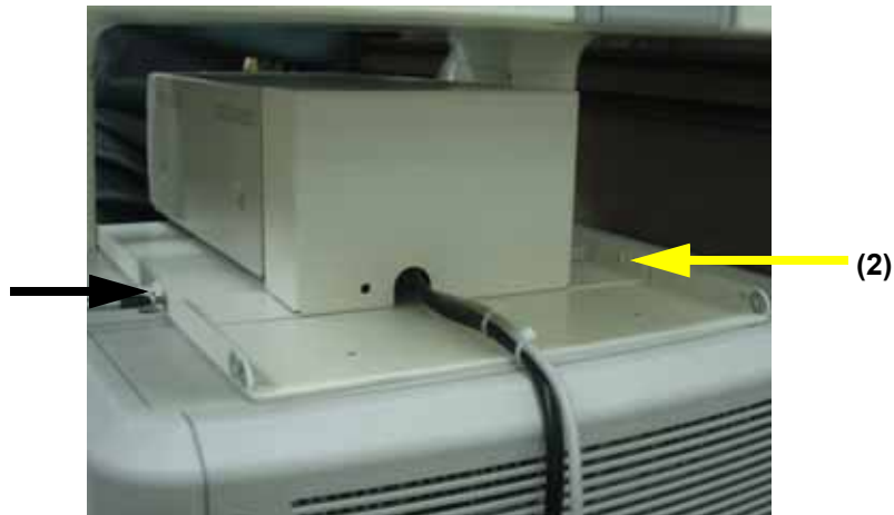
Figure 8-293 BW Printer Fixture Middle installation
