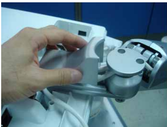
Figure 8-58 Assembling the Fold Cover
