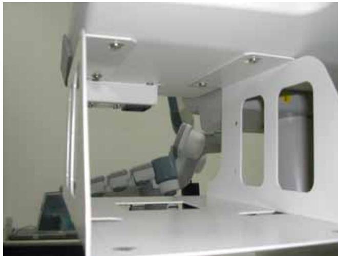
Figure 8-285 BW Printer Fixture Keyboard installation
