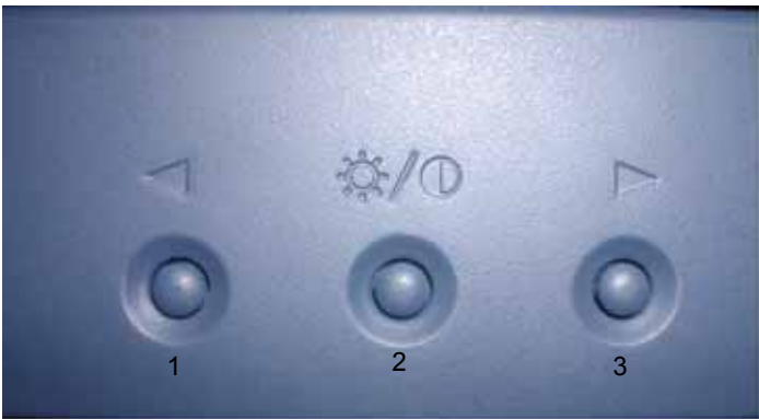
Figure 5-14 LCDMON control buttons
