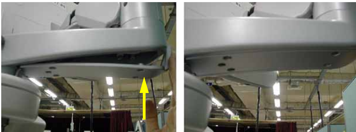
Figure 8-274 Assembling the Arm bottom cover
