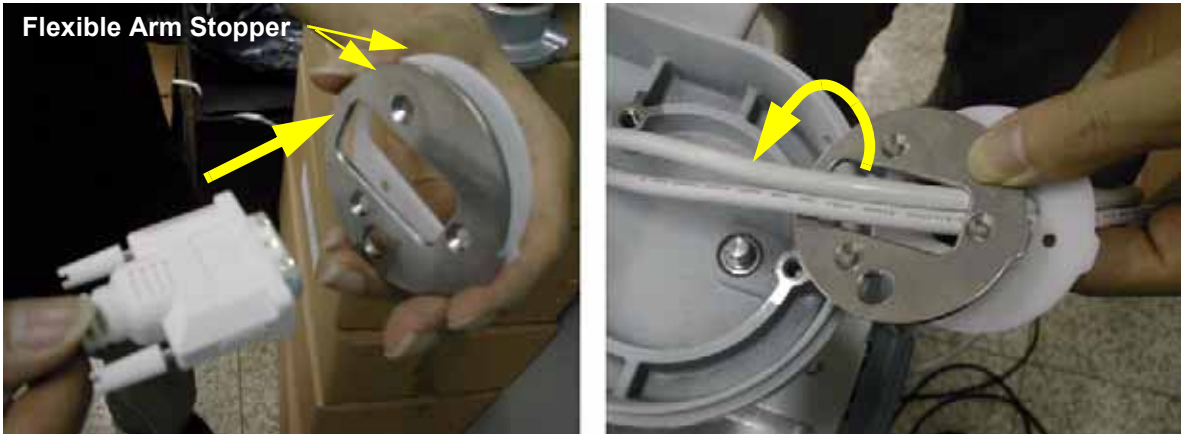
Figure 8-36 Inserting cables to the flexible arm stopper
