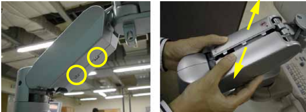
Figure 8-23 Removing the Arm cover L & Arm cover R
