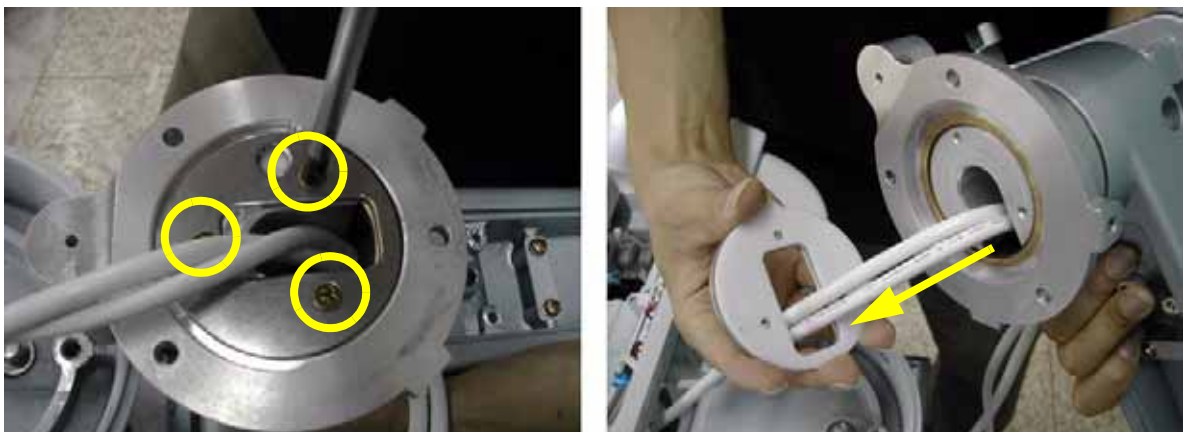
Figure 8-248 Separating the flexible arm stopper Section 8-7 - Mechanical Option Installation instruction
