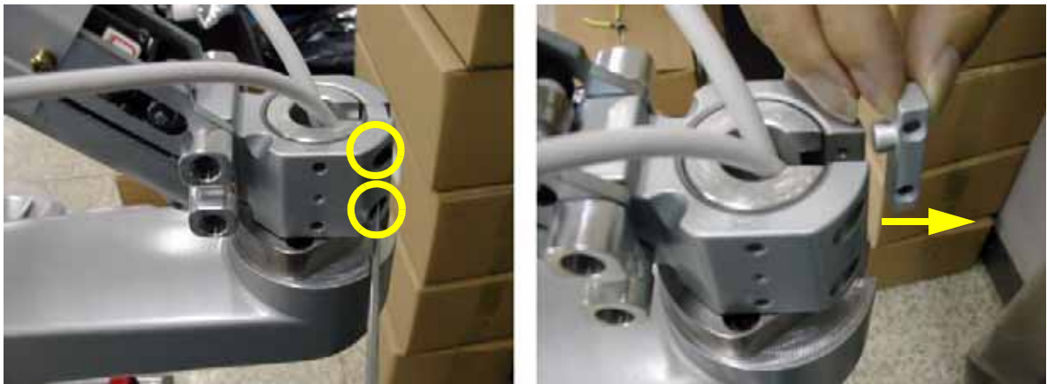
Figure 8-242 Removing the Arm stopper
