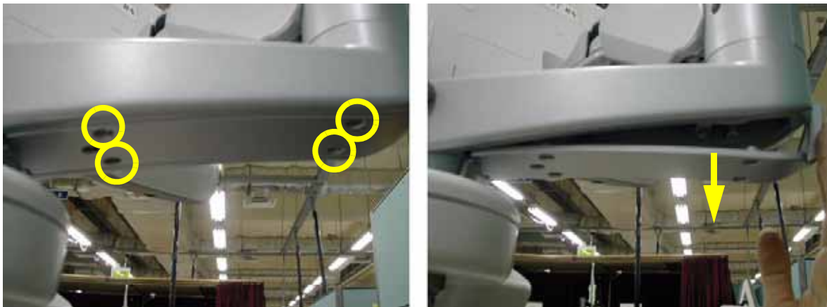
Figure 8-64 Removing the Arm bottom cover
