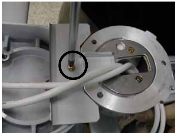
Figure 8-247 Removing OP bracket
