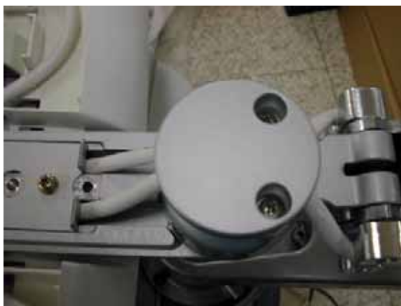
Figure 8-50 Assembling the Arm Cable Cover
