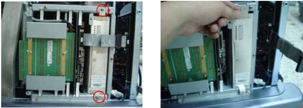
Figure 8-104 Pull out the APS Assy
