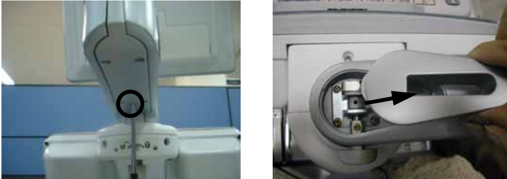
Figure 8-66 Removing the Arm lock cover
