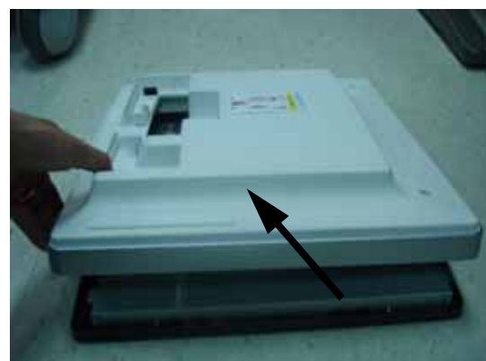
Figure 8-5 Removing the 17" LCD rear cover
