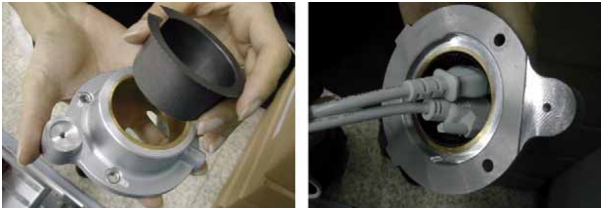
Figure 8-251 Inserting the oilless bush
