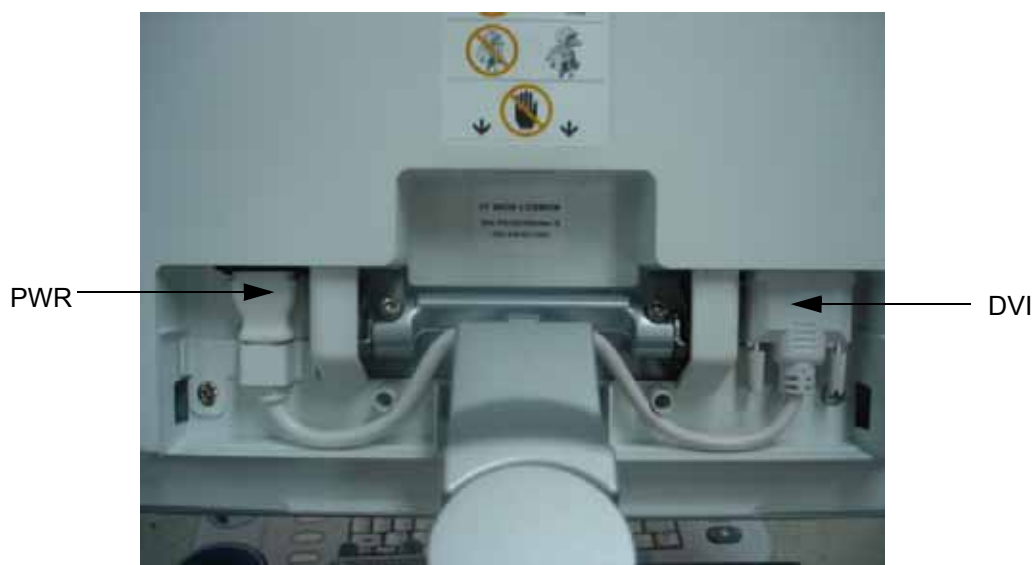
Figure 5-13 LP6 17" LCDMON Signal I/O
