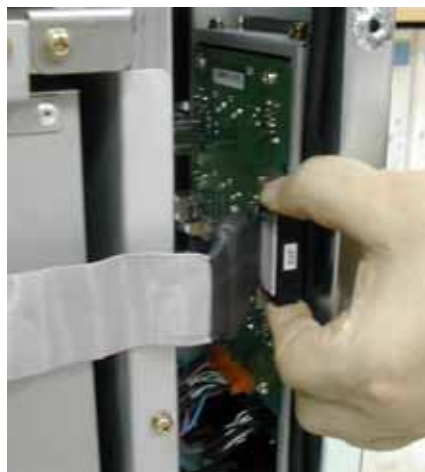
Figure 8-134 AEXP Cable of rear panel
