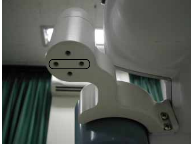
Figure 8-276 Endo Probe Holder Installation
