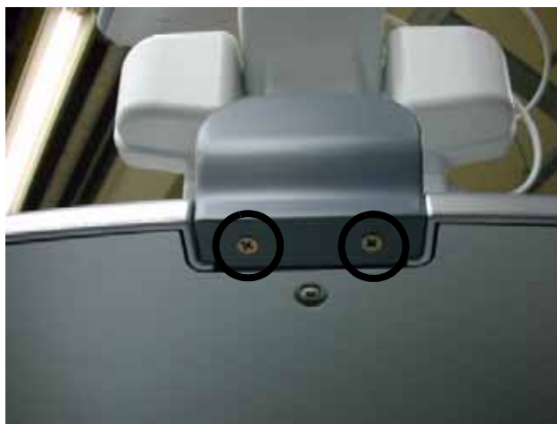
Figure 8-327 Rear Handle Installation
