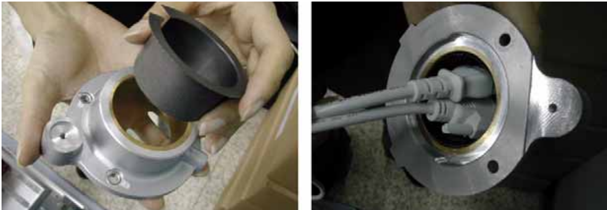
Figure 8-37 Inserting the oilless bush
