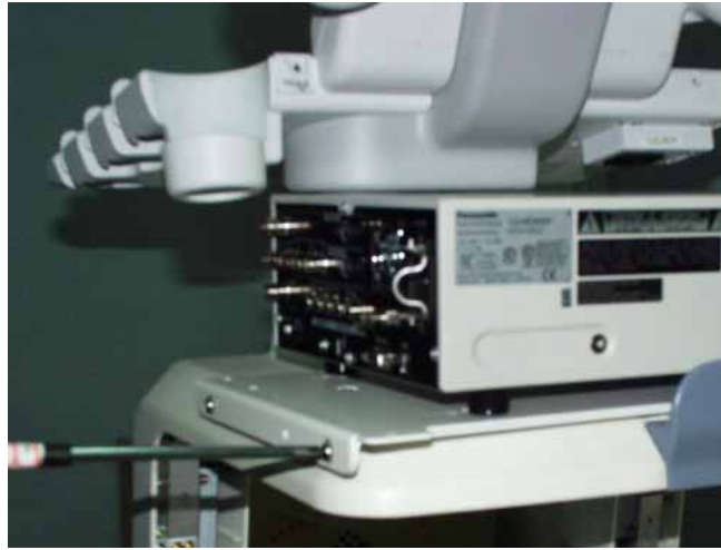
Figure 8-325 Printer VCR DVD Fixture Top installation (MD-800)
