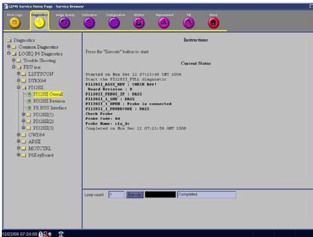
Figure 4-35 PI128II diagnostic test
