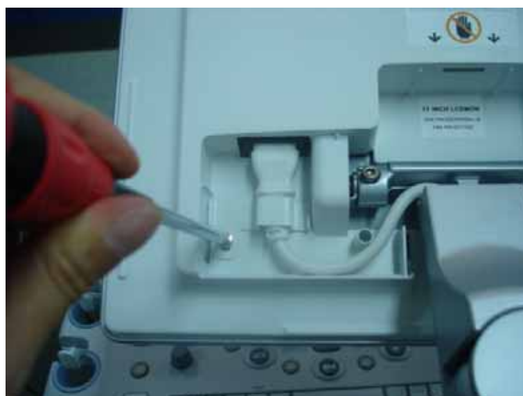
Figure 8-232 Removing the power cord bracket
