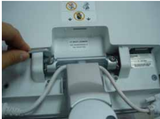
Figure 8-15 Removing the power code bracket
