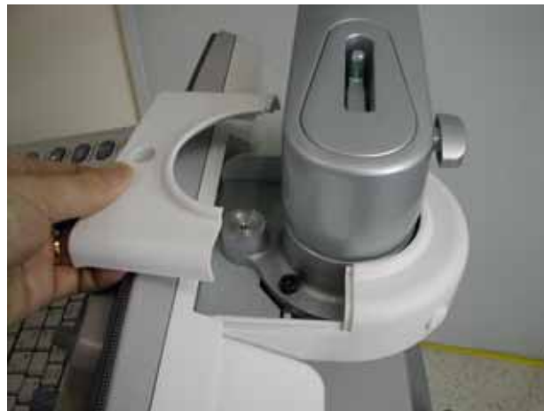
Figure 8-97 Open neck front cover
