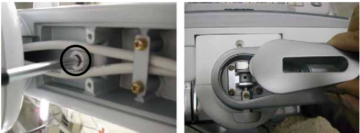
Figure 8-26 Removing the Lock cover
