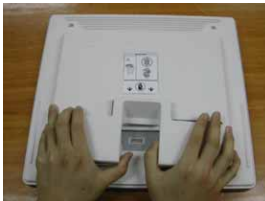
Figure 8-9 Removing the LCD Cable cover
