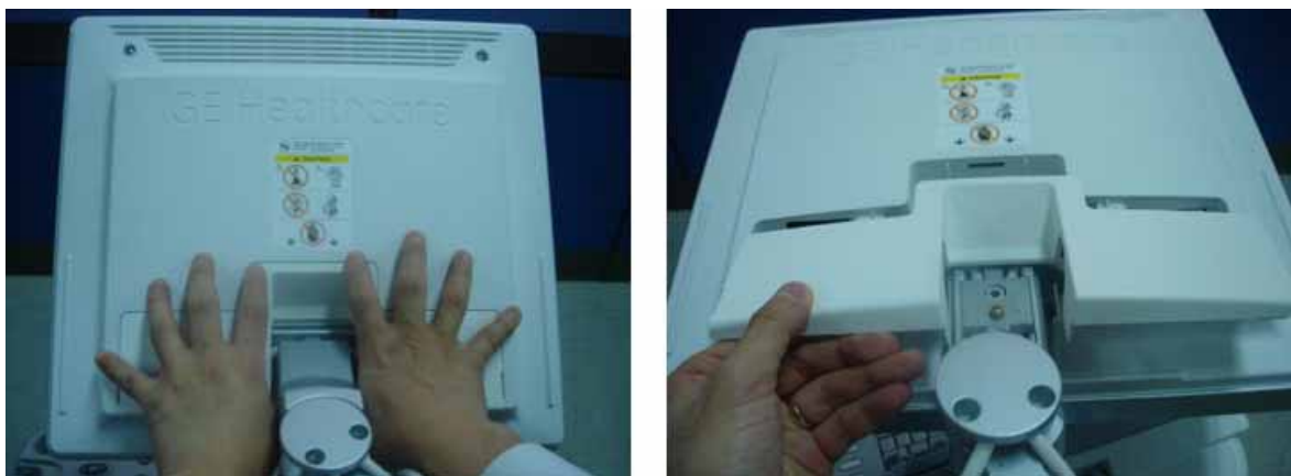
Figure 8-231 Removing the LCD cable cover
