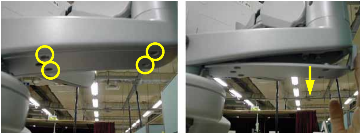
Figure 8-239 Removing the Arm bottom cover
