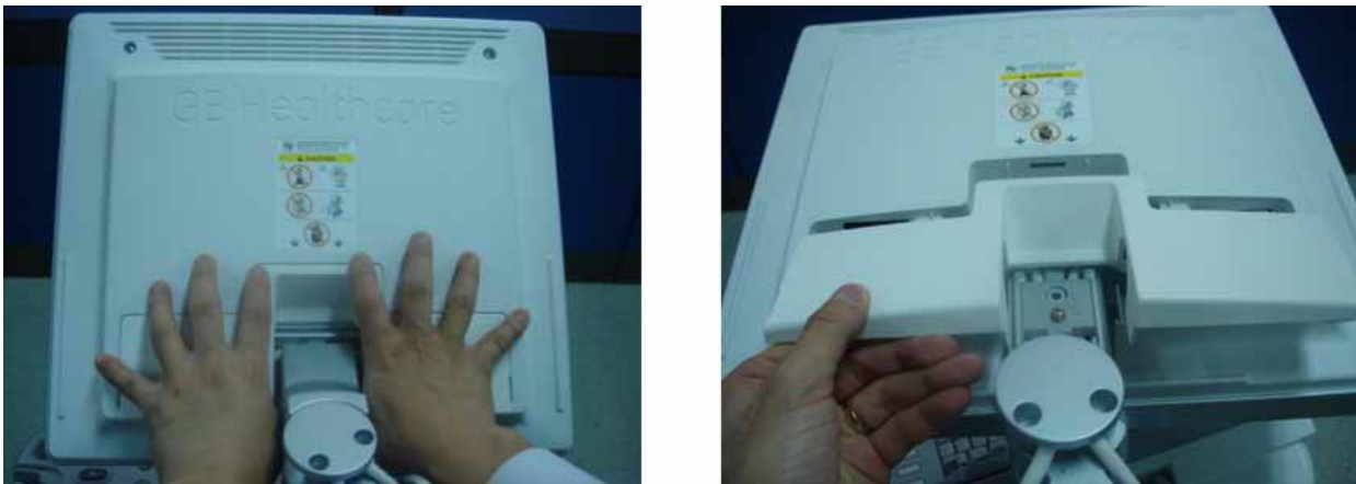
Figure 8-17 Removing the LCD cable cover
