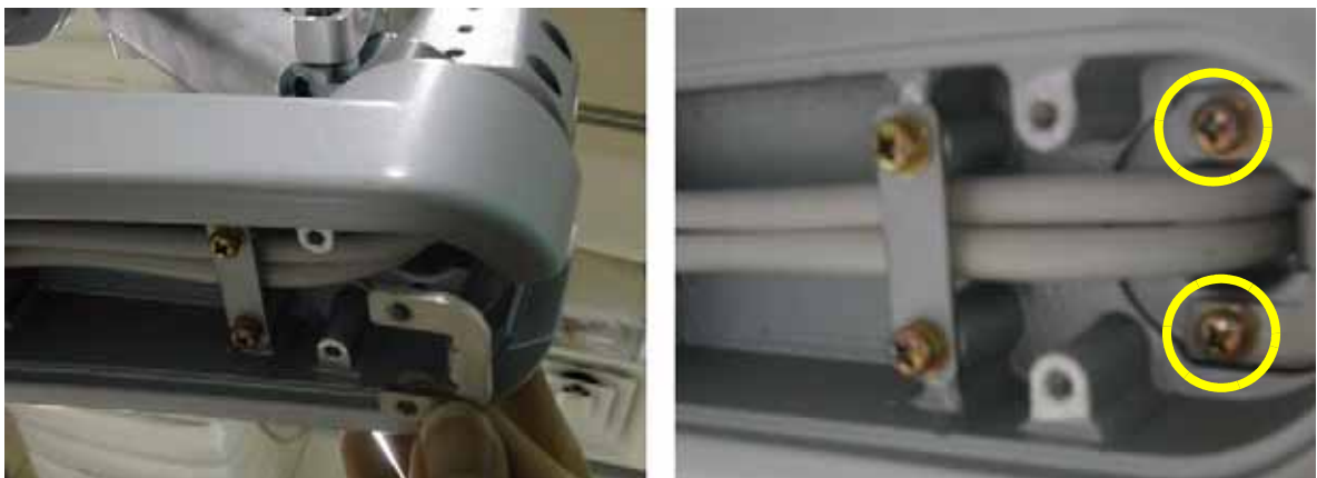
Figure 8-46 Assembling the Lower arm guide bracket
