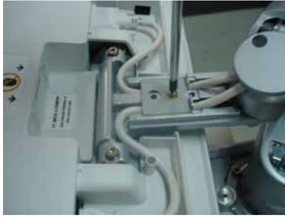
Figure 8-265 Placing the cables
