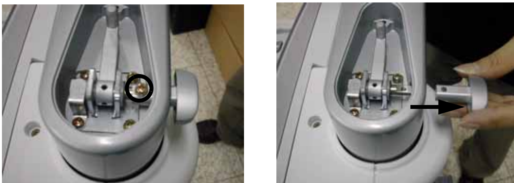
Figure 8-68 Removing the Arm lock Knob
