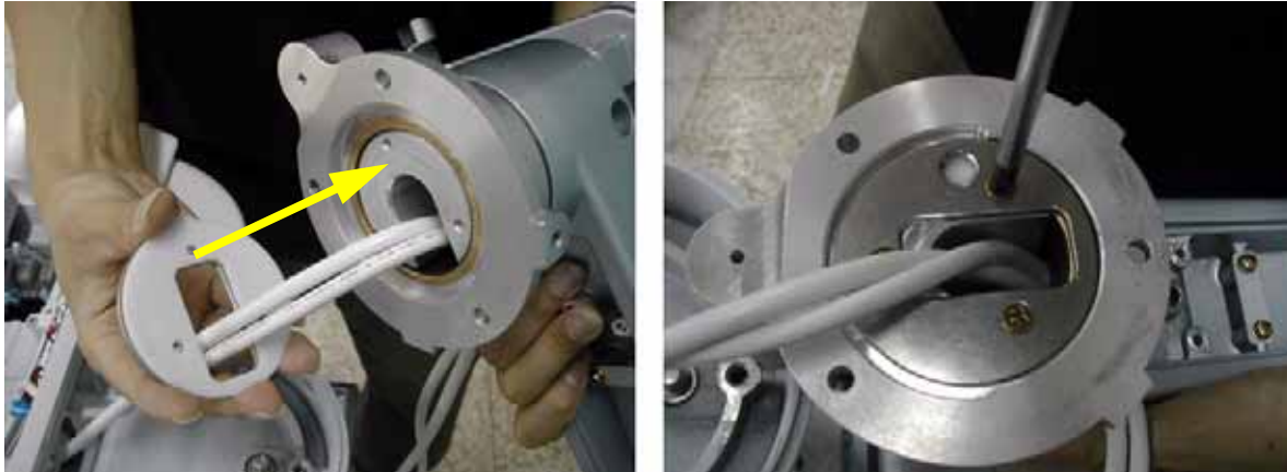
Figure 8-253 Fixing the flexible arm stopper
