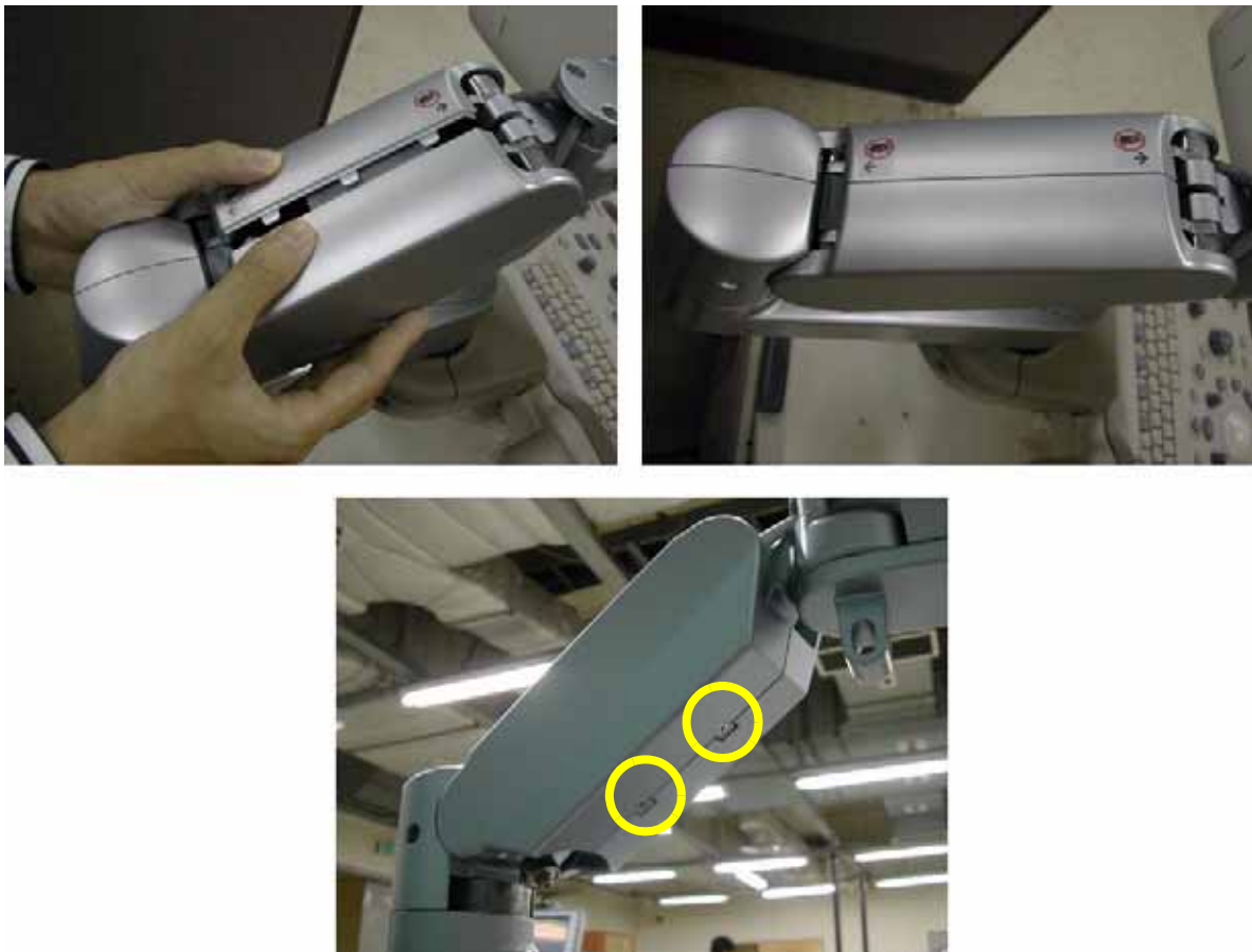
Figure 8-273 Assembling the Arm Cover L & R
