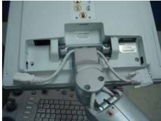
Figure 8-3 Disconnecting power cable and DVI cable
