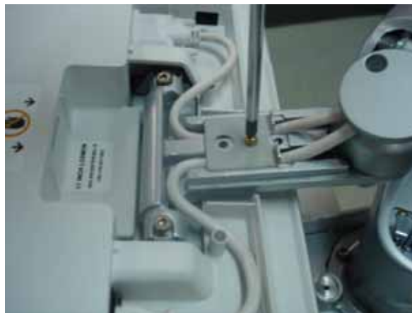
Figure 8-263 Assembling the Cable bracket
