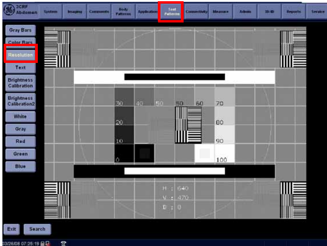
Figure 4-22 17" LCDMON II Assy Function Check
