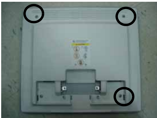
Figure 8-5 Removing the 17" LCD rear cover
