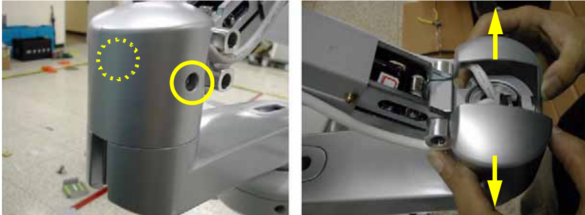
Figure 8-238 Removing the Cam cover L & Cam cover R
