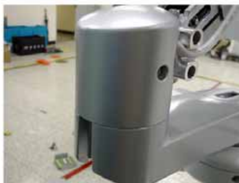
Figure 8-57 Assembling the Cam Cover L & R
