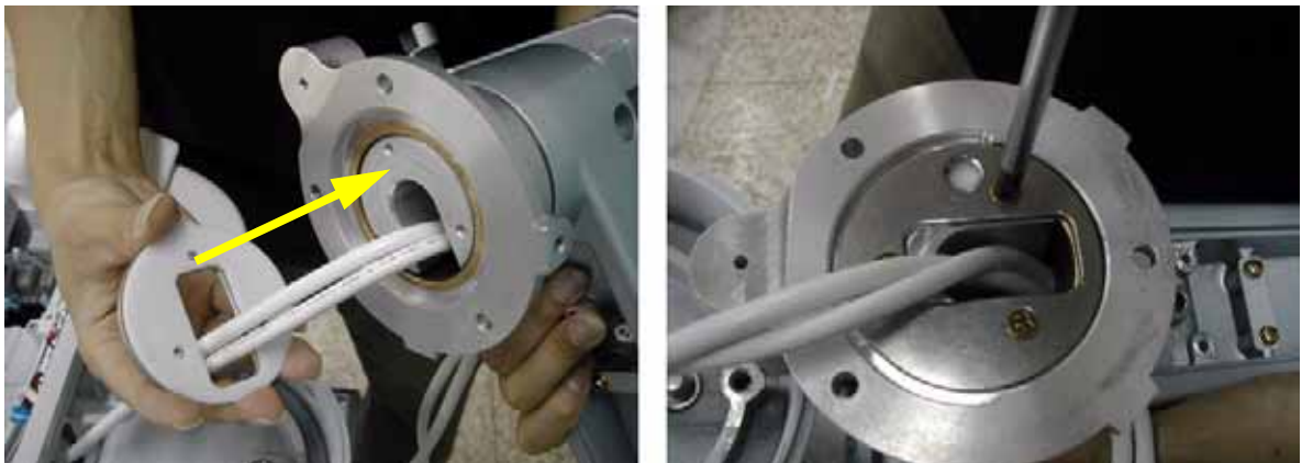
Figure 8-39 Fixing the flexible arm stopper
