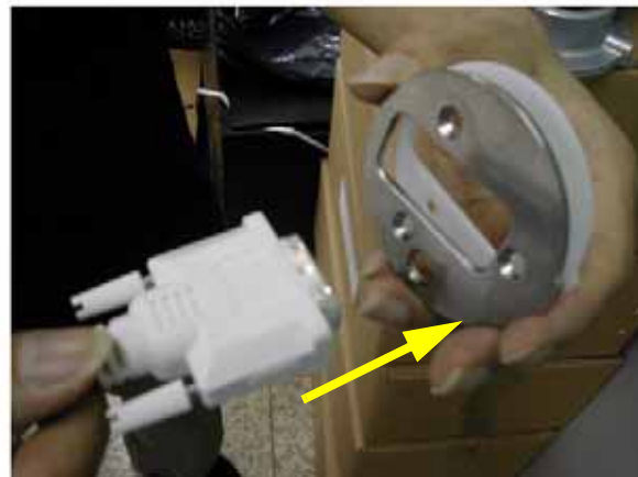
Figure 8-249 Pulling out power cable & DVI cable and removing the stopper
