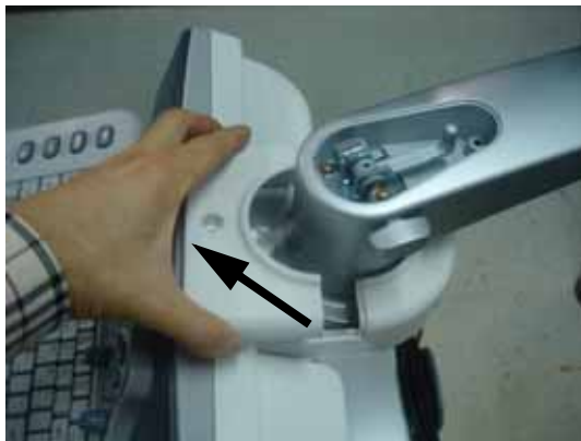
Figure 8-31 Unscrewing 3 screws and removing the neck front cover & neck rear cover
