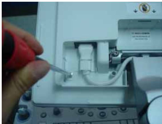
Figure 8-2 Removing the power cord bracket
