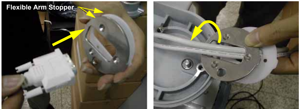
Figure 8-250 Changing the MON PWR CONN LONG cable
