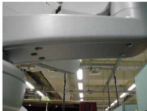
Figure 8-60 Assembling the Arm bottom cover
