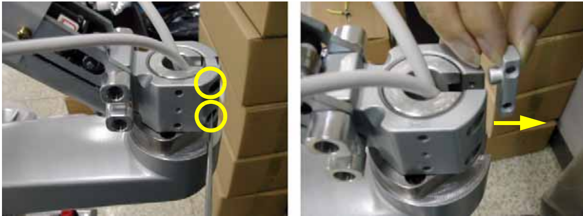
Figure 8-28 Removing the Arm stopper
