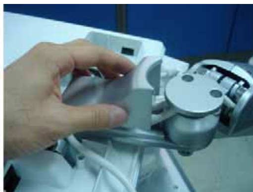
Figure 8-20 Removing the Fold cover
