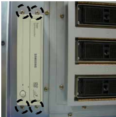
Figure 8-129 Unscrew 4screws and remove the DVD Assy
