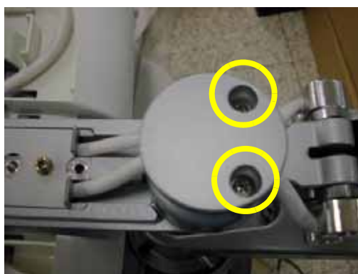
Figure 8-21 Removing the Arm cable cover
