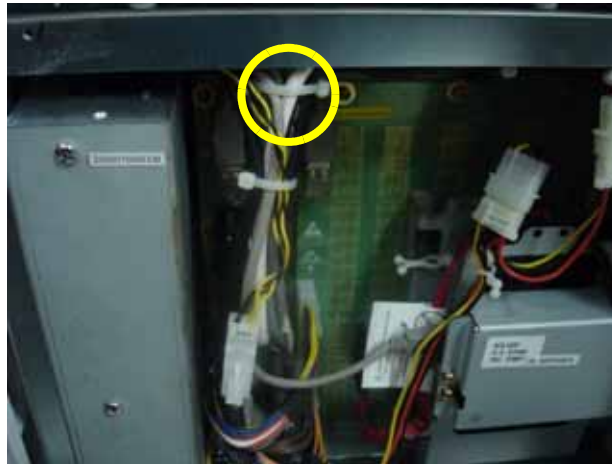
Figure 8-131 Connector and Screw2 screws on the Nest Fan
