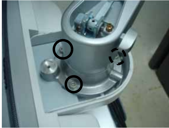
Figure 8-41 Assembling the arm neck pipe
