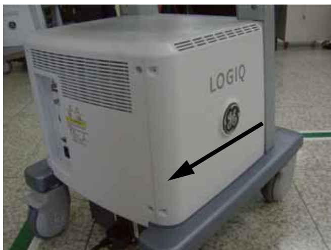
Figure 8-87 Open side cover
