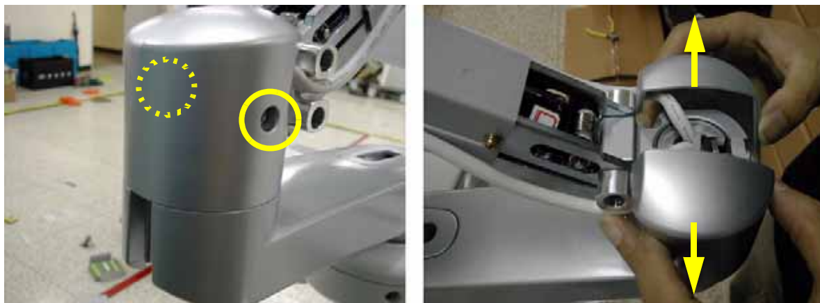
Figure 8-63 Removing the Arm cam cover L & Arm cam cover R
