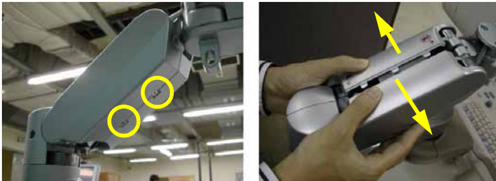
Figure 8-237 Removing the Arm cover L & Arm cover R
