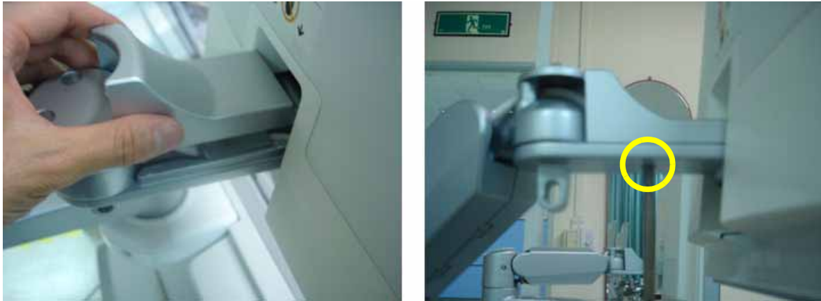
Figure 8-272 Assembling the Fold Cover
