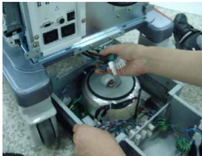
Figure 8-145 Insert the Transbox assy
