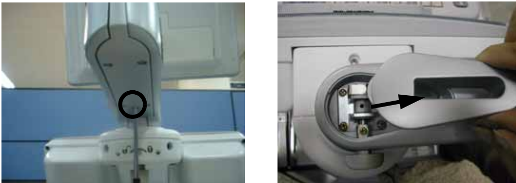
Figure 8-67 Removing the Arm lock cover
