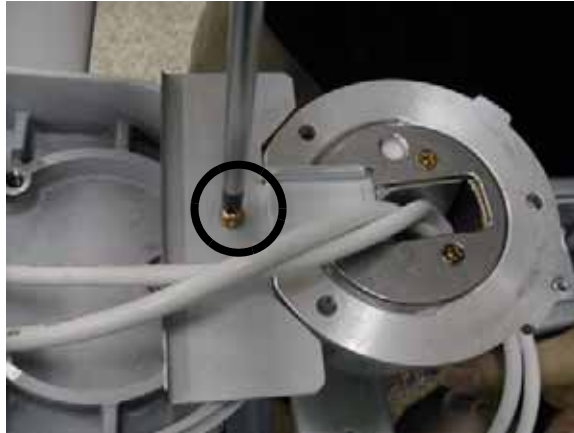
Figure 8-33 Removing OP bracket
