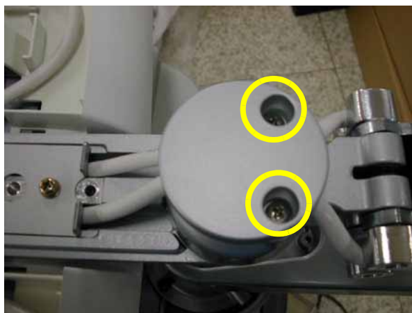
Figure 8-65 Removing the Arm cable cover
