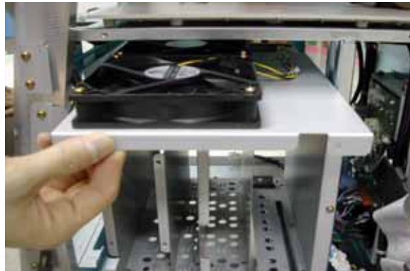
Figure 8-132 Pull out the nest fan
