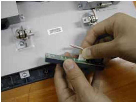
Figure 8-13 Disconnecting the cable
