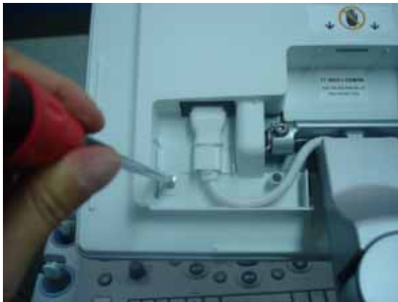
Figure 8-266 Assembling the power cord bracket
