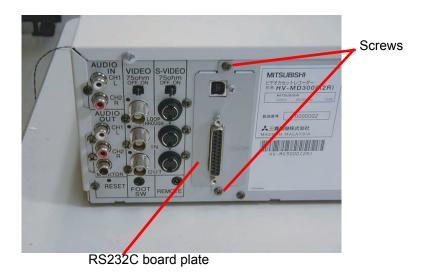
Figure 6-109 Opening Board Plate
