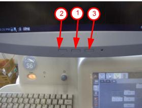
Figure 6-89 17 inch IPS-Pro Type LCD Monitor Adjustment buttons
