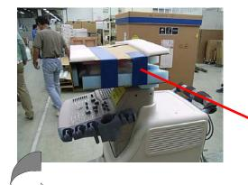
Secure the LCD Sleeve with adhesive tape after placing it to the proper location.
