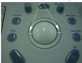
Figure 6-102 Rotating the Retainer Ring
