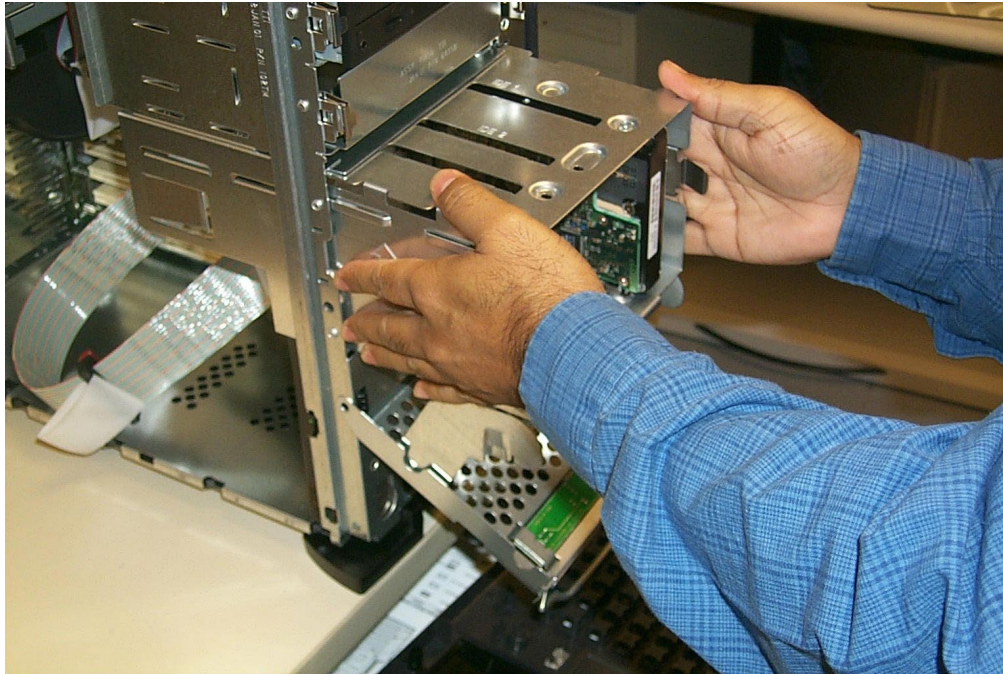
Illustration 3-16: Slide out hard drive cage
