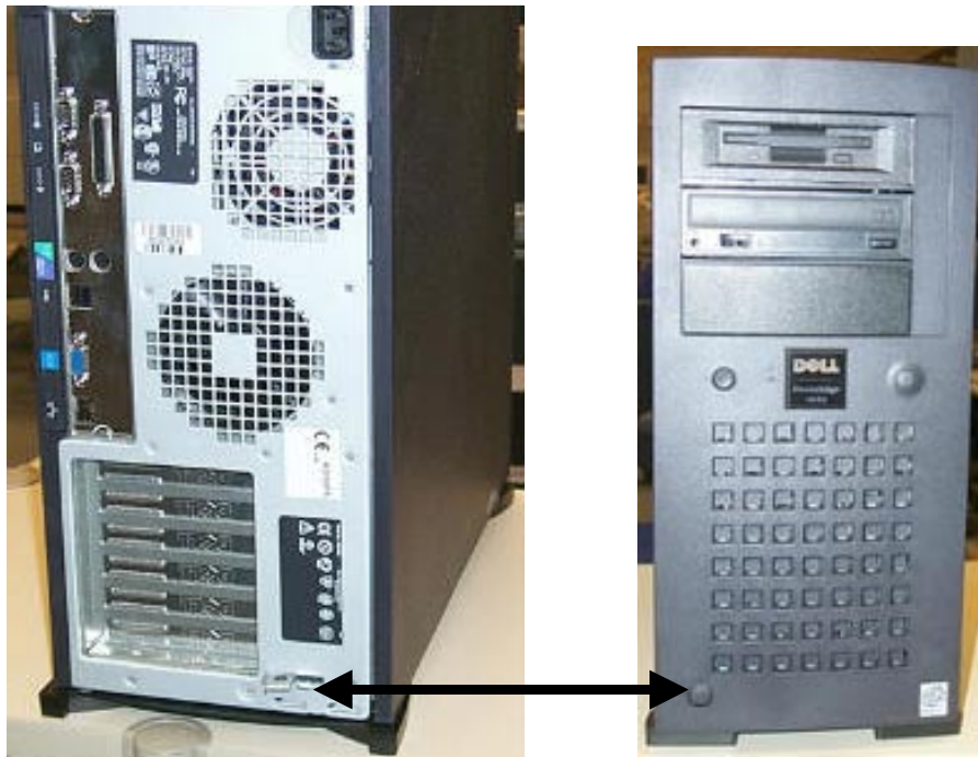
Illustration 3-35: Side Access Panel Release.
