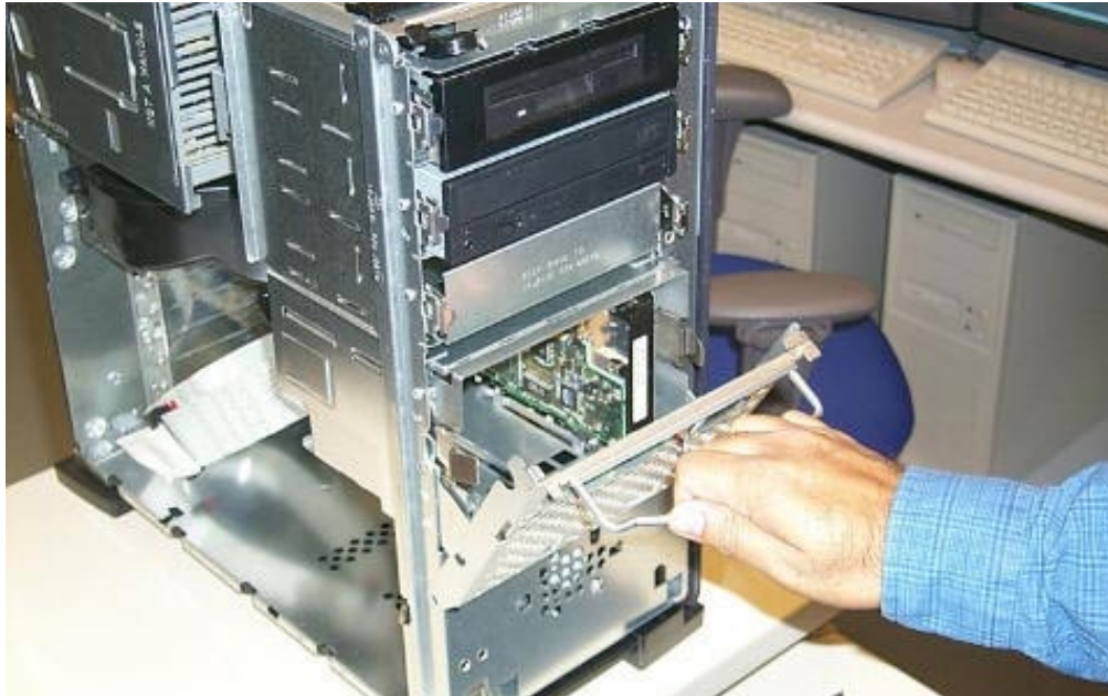
Illustration 3-15: Hard Drive Cage Access
