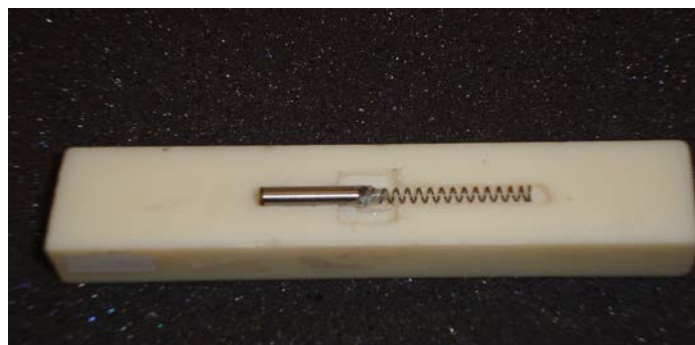
Figure 17.U. Spring - Dowel Pin Assembly and Alignment Tool
