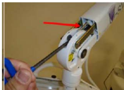
Figure 18-3. Insertion Point for Head Arm Adjustment
