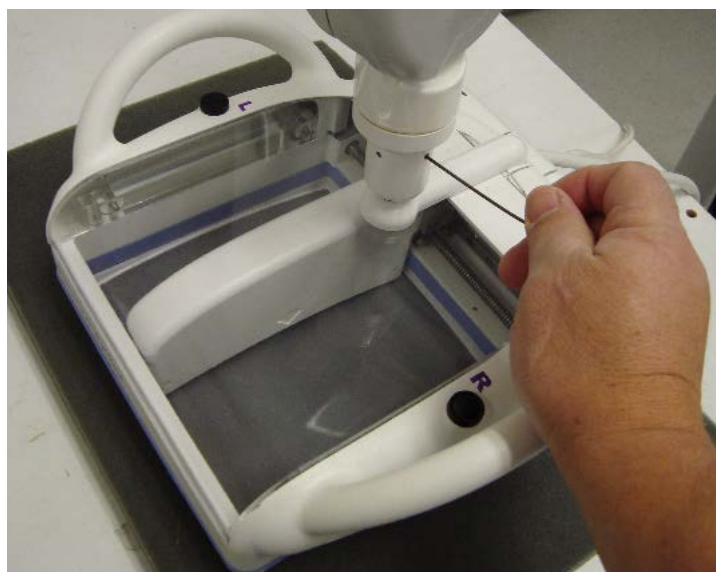
Figure 17.I. The 2 set screws on the scanner assembly retainer collar
