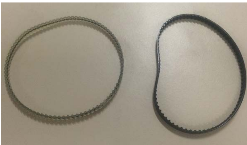
Figure 17.DD. Motor Belt: Gray (2102-0008-00) and Black (2012-0008-02)
