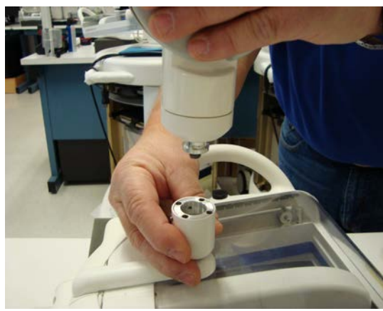
Figure 17.J. Must hold the arm while separating the Scanner assembly
