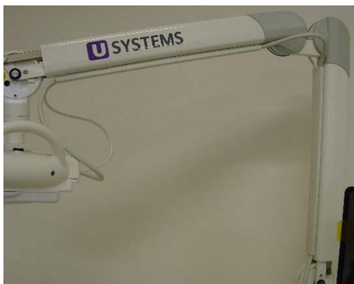
Figure 17.G. Plastic conduit raceways to enclose the Scanner cables
