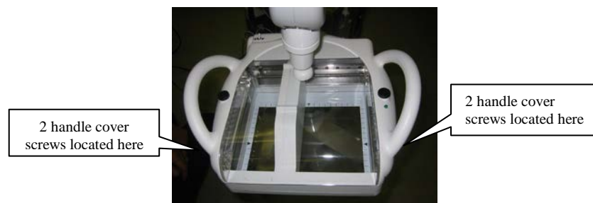
Figure 17.L. Locations of the screws to hold the handles
