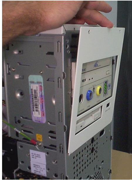
Figure 8-61 Front Cover Removal - BEP2
