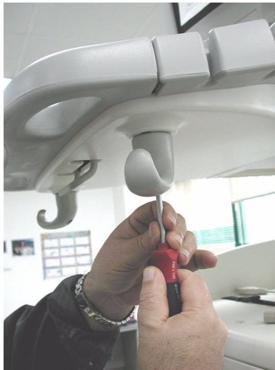
Figure 8-15 Removing Probe Cable Hooks under Keyboard Cover
