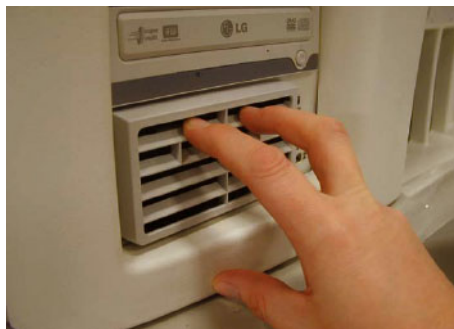
Figure 8-78 BEP Filter ASSY removal
