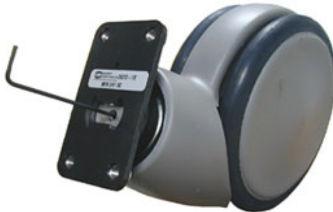
Figure 6-7 Rear Brakes adjustment
