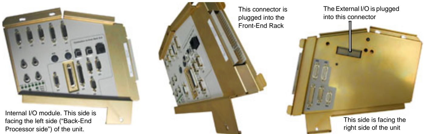
Figure 5-63 The Internal I/O module seen from different angles
