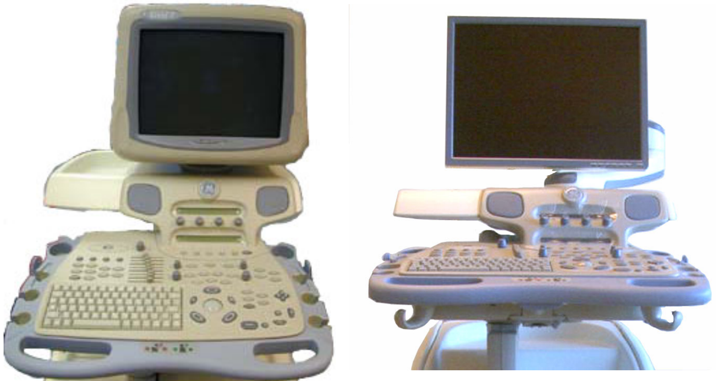
Figure 5-69 Top Console. CRT Monitor to the left, LCD Monitor to the right
