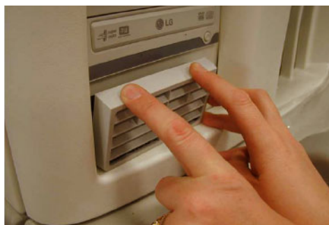
Figure 8-79 BEP Filter ASSY installation
