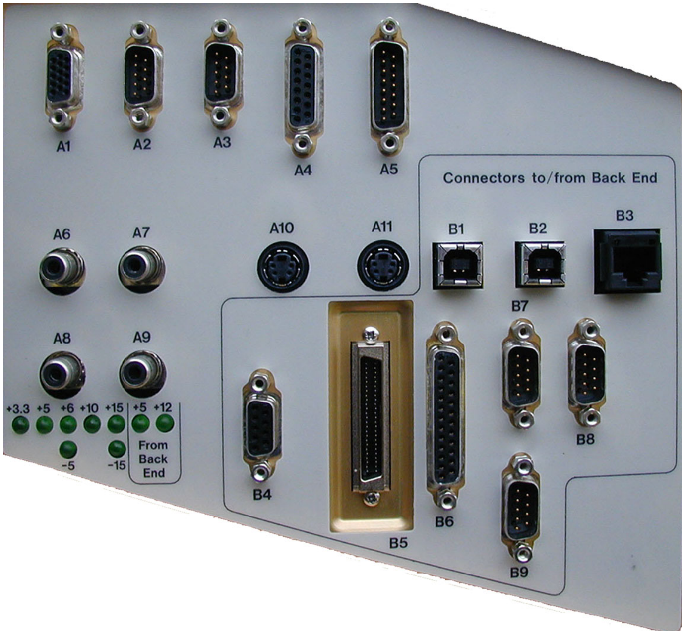
Figure 1-3 Labels on Internal I/O (Inside Scanner), Back-End Processor Side of Internal I/O
