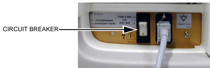
Figure 4-9 Circuit Breaker located on rear of the unit
