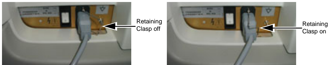
Figure 4-1 Female power plug with retaining clasp off (to the left) and on (to the right)
