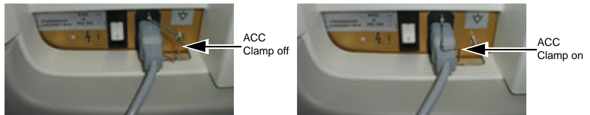
Figure 3-12 Female power plug with retaining clamp off (to the left) and on (to the right)
