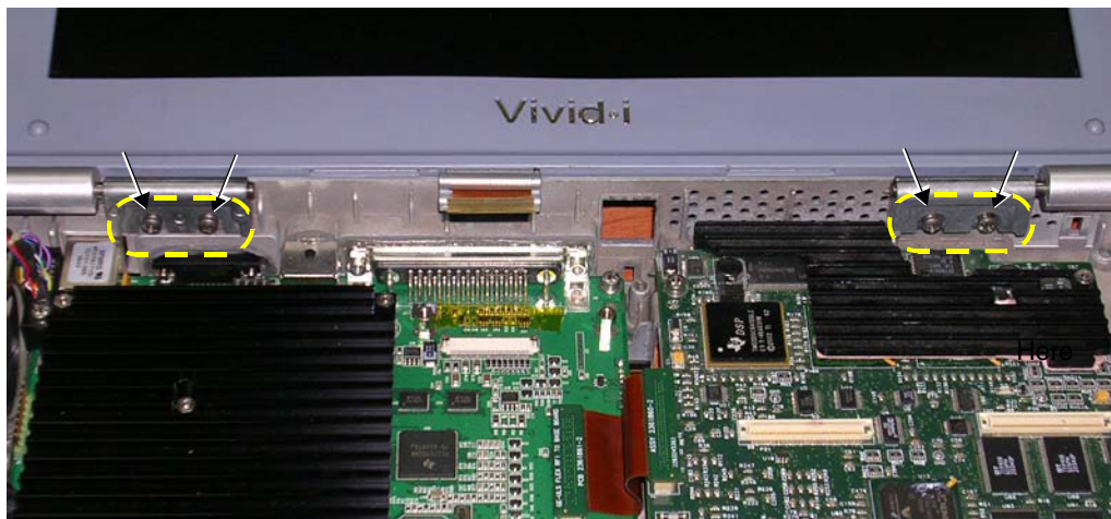
Figure 8-16 LCD Display Hinges Secured to Base Assembly - Location of Screws
