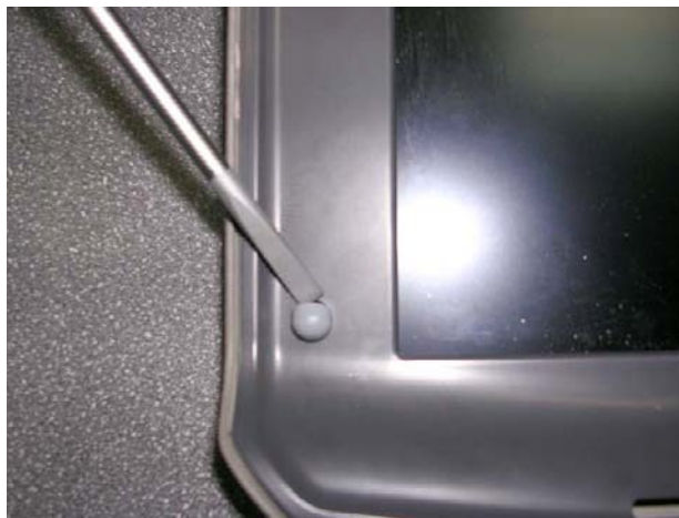
Figure 8-19 Removing the Screw Caps from the LCD Display Frame
