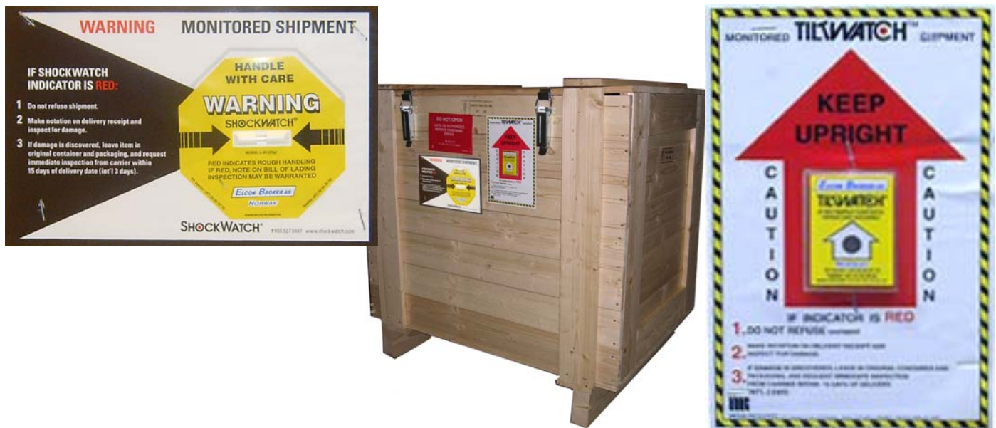
Figure 3-1 Tiltwatch and Shockwatch positions on Transportation Box
