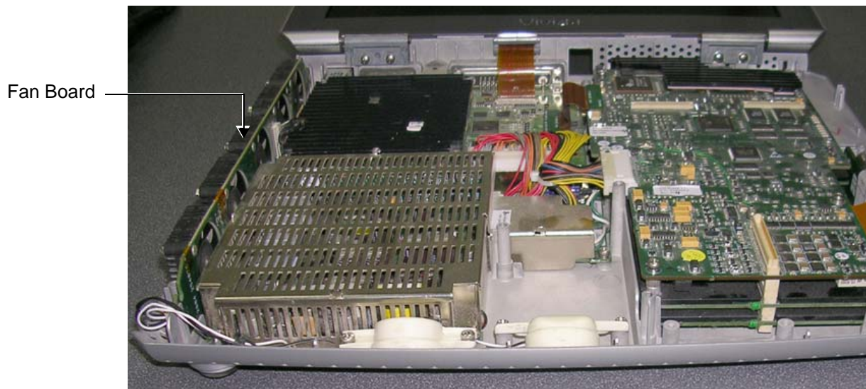
Figure 5-19 Location of Fan Board in the Bottom Assembly
