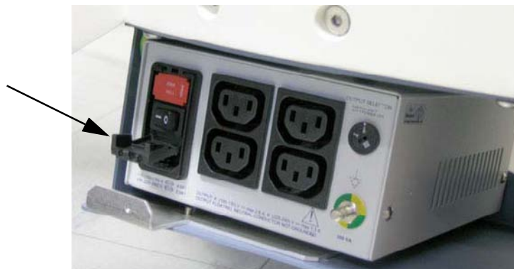
Figure 8-81 Open fuse protection on rear of transformer
