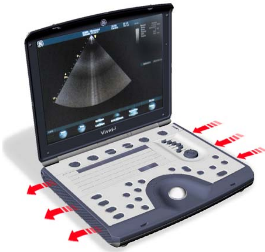
Figure 5-31 Air Flow through the Vivid i n Ultrasound Scanner
