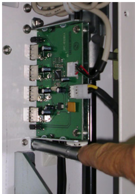
Figure 8-93 Removing the USB Box Cover
