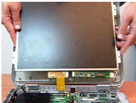
Figure 8-68 Removing the LCD Display
