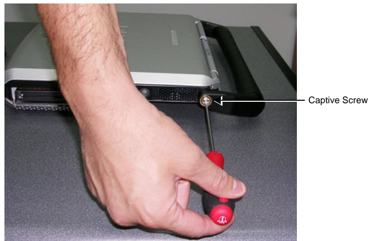
Figure 8-2 Releasing the Bearing Handle Captive Screw
