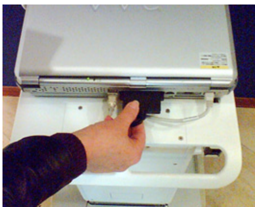
Figure 3-65 Connecting the Docking Connector to the Rear of Scanner
