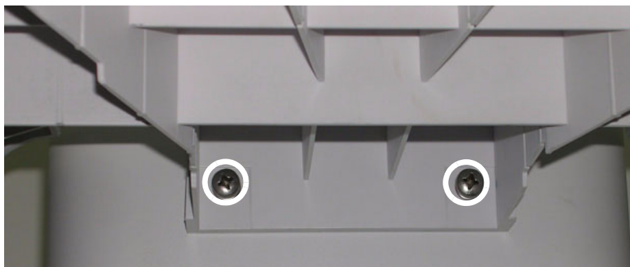
Figure 8-103 Probe Shelf Assembly - Lower Securing Screws
