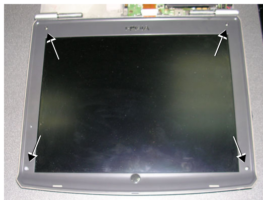
Figure 8-31 Removing the Securing Screws
