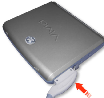
Figure 3-58 Connecting Probe to the Vivid i n/ Vivid q N
