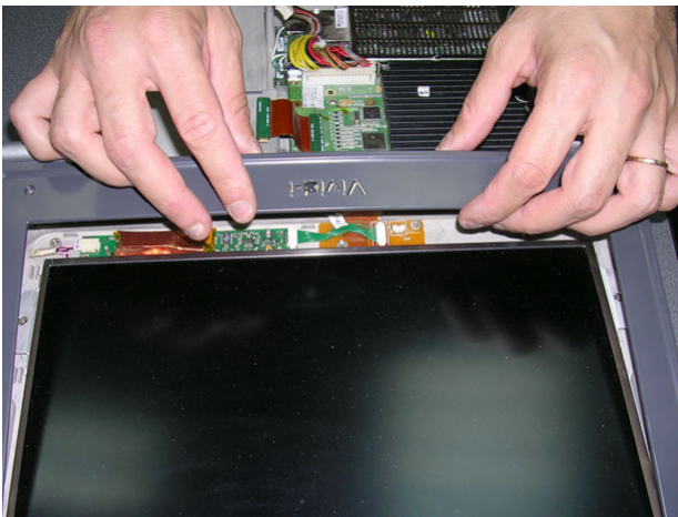
Figure 8-32 Removing the LCD Display Frame
