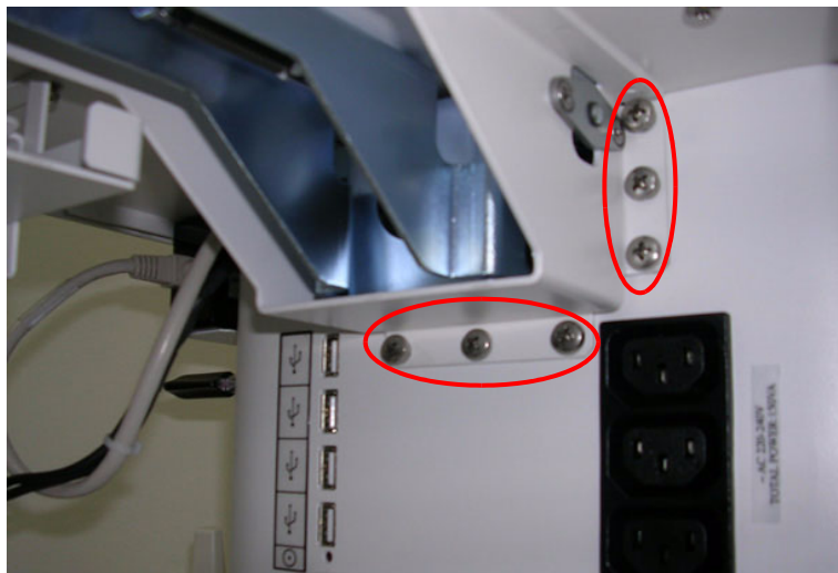
Figure 8-100 Top Shelf - Lower Retaining Screws
