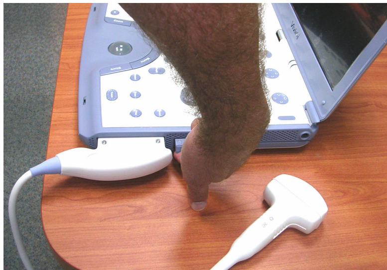
Figure 3-59 Securing Probe with Locking Lever
