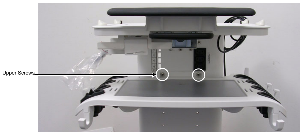
Figure 8-104 Probe Shelf Assembly - Upper Securing Screws
