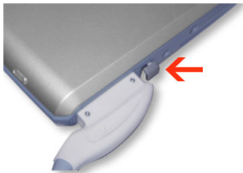
Figure 3-57 Probe Connection Locking Lever
