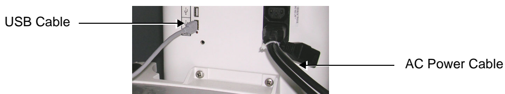
Figure 3-20 AC Power Cable and USB Cable Connected to SafeLock Cart
