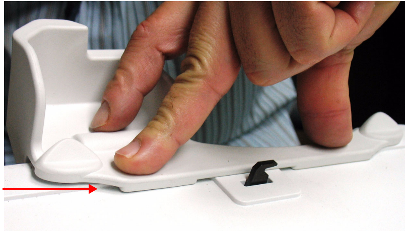
Figure 8-79 Placing the ECG Cable Protector in Position
