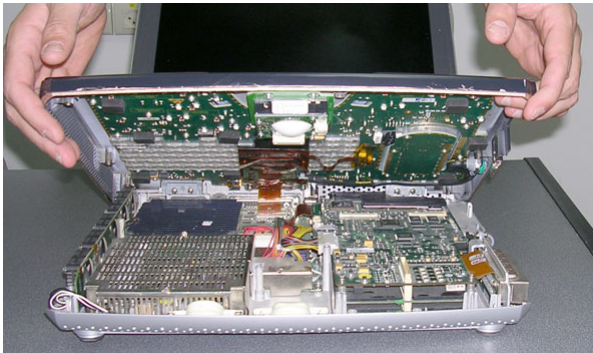
Figure 8-14 Removing the Control Panel and Keyboard
