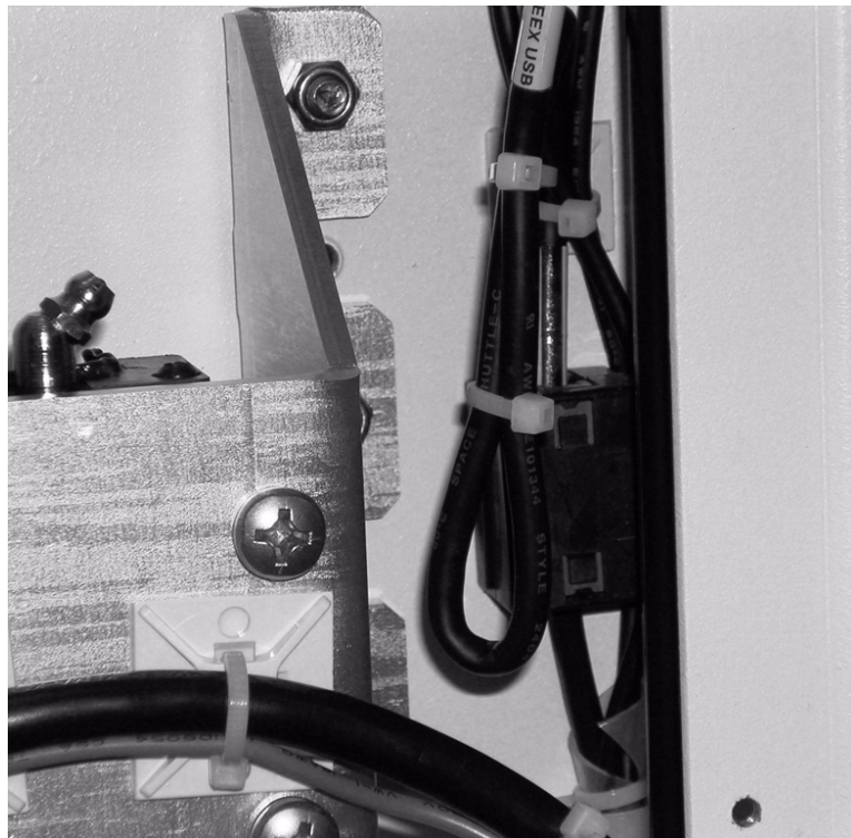
Figure 8-91 USB Power Cable Folded and Fastened with Tie-wraps
