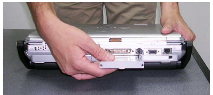
Figure 8-7 Removing the Hard Disk
