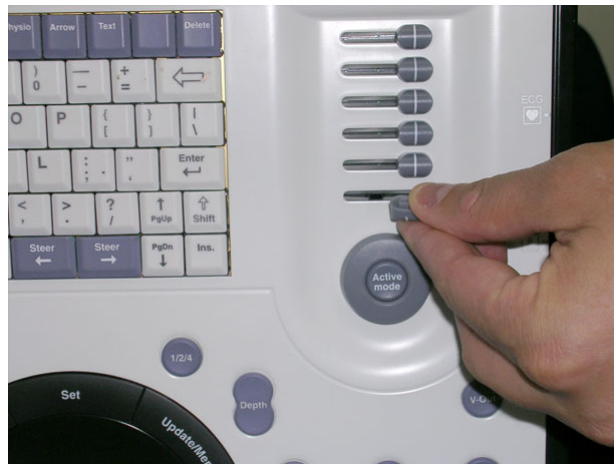
Figure 8-18 ATGC Slider Keycap Replacement
