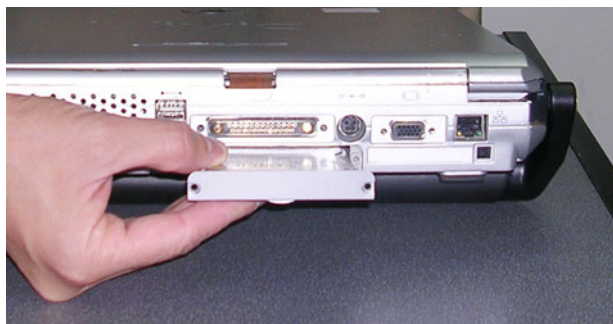
Figure 8-7 Removing the Hard Disk
