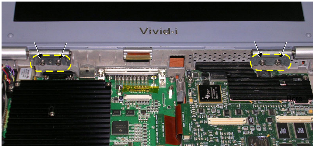
Figure 8-29 LCD Display Hinges Secured to Base Assembly - Location of Screws
