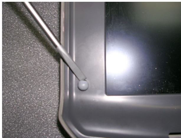
Figure 8-30 Removing the Screw Caps from the LCD Display Frame
