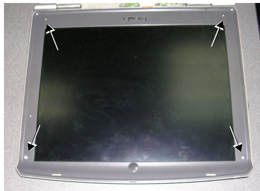
Figure 8-62 Removing the Screws from the LCD Display
