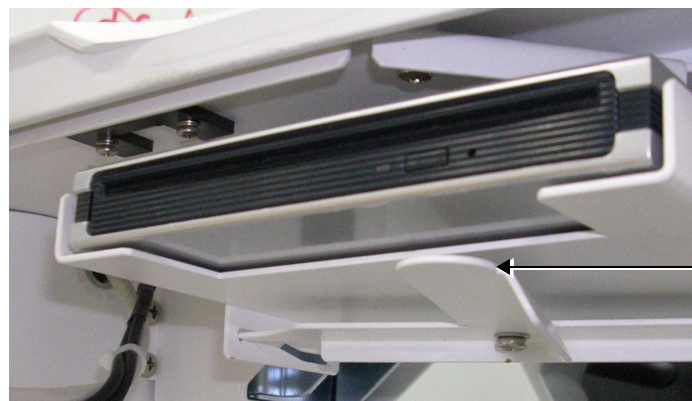
Figure 3-33 Retaining Clamp for DVD-R/RW Drive
