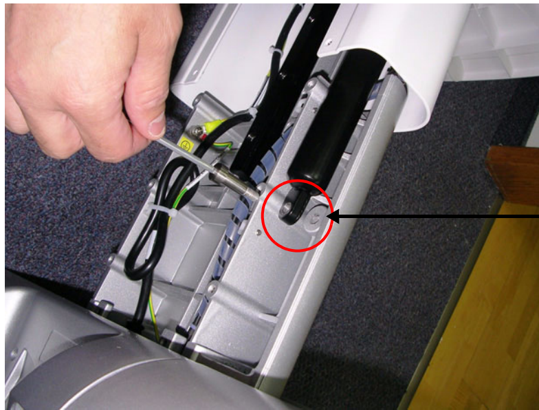
Figure 8-97 Lower Gas Spring Securing Bracket
