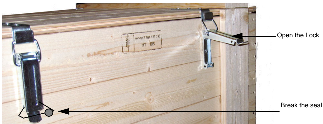
Figure 3-6 To remove the Lid of the Box
