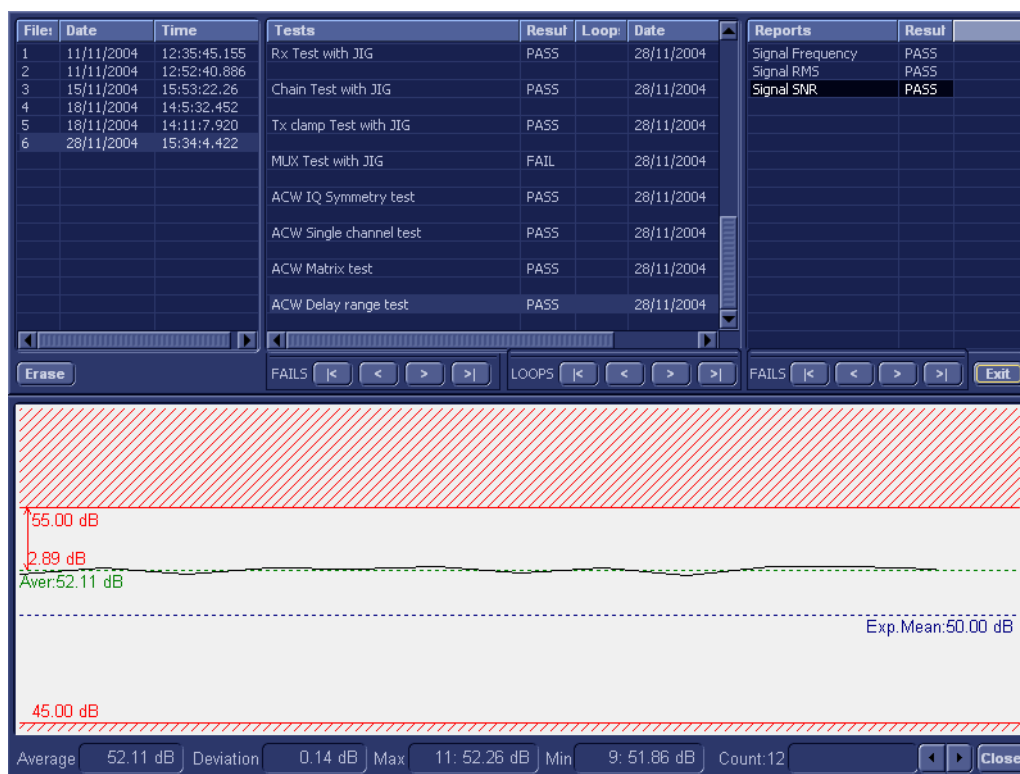
Figure 7-44 View Test Log - ACW Delay Range Test - Signal SNR
