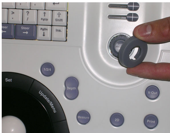
Figure 8-19 ATGC Rotary Knob Replacement
