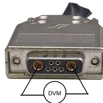
Figure 7-2 Connectors and corresponding voltage check points
