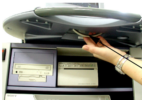
Figure 5-23 Locking lever under Control Console
