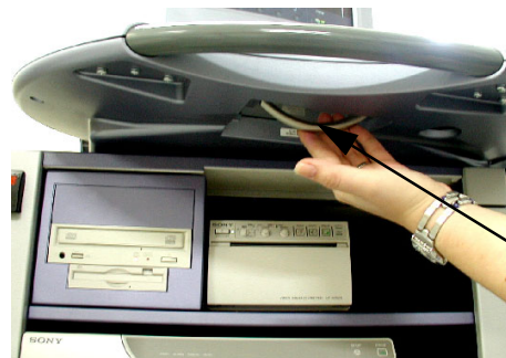
Figure 6-4 Locking Lever under Control Console
