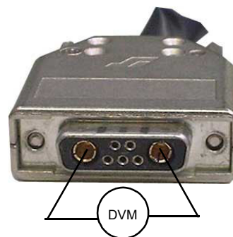
Figure 7-2 Connectors and corresponding voltage check points
