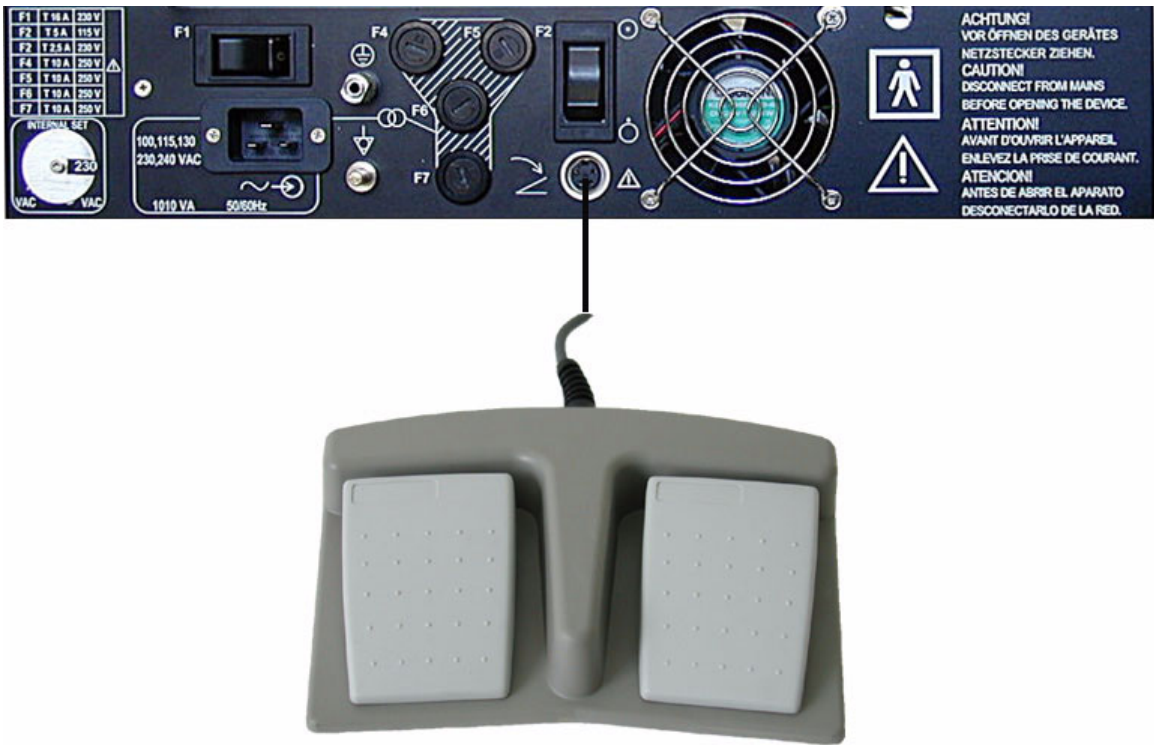
Figure 3-9 Foot Switch Connection Scheme
