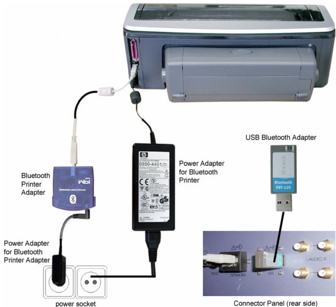
Figure 3-17 Bluetooth Printer Connection Scheme
