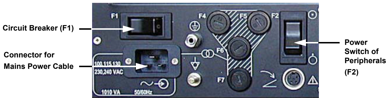
Figure 3-22 Circuit Breaker (F1) and Power Switch of Peripherals (F2)
