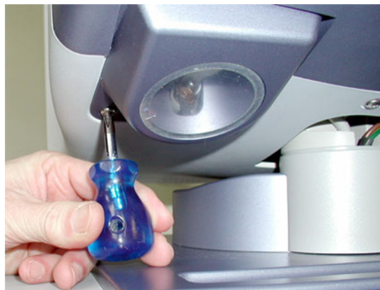
Figure 8-24 remove cover of the task lamp
