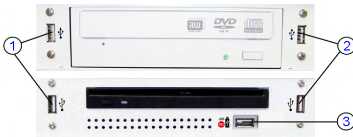
Figure 3-64 External I/O connectors - next to DVD or DVR drive
