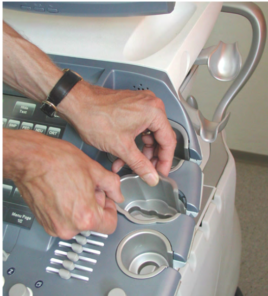
Figure 8-24 pull out the probe holder
