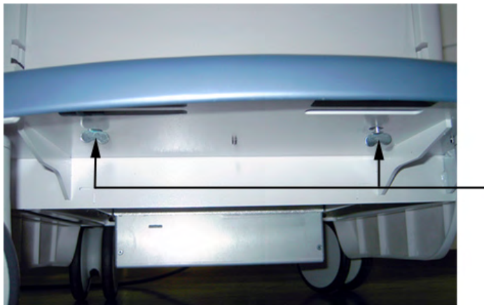
Figure 8-21 turn quick release devices 90° and remove the footrest cover
