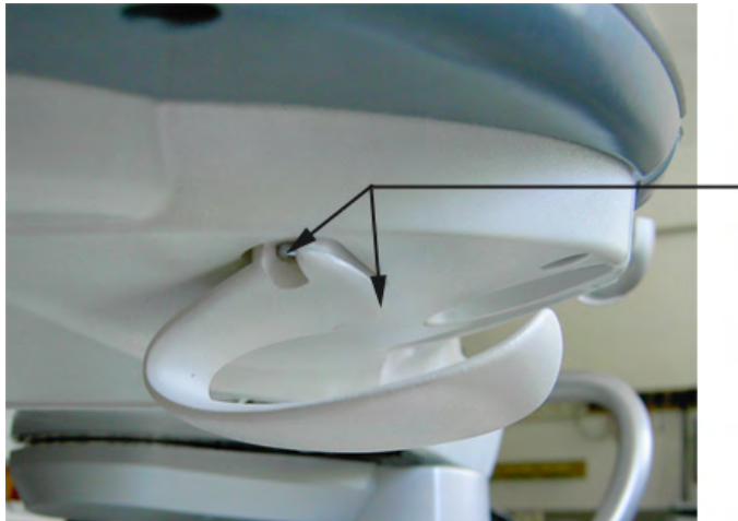
Figure 8-23 loosen 2 screws and remove cable holder
