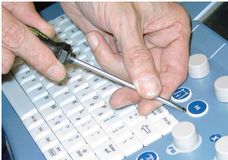
Figure 8-29 push against the circle cap and lift it
