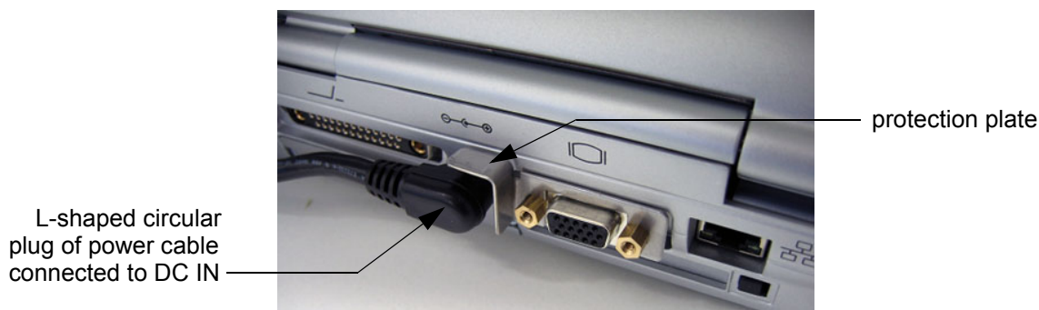
Figure 3-20 main power cable connected to Voluson i / Voluson e's power inlet (DC IN) connector
