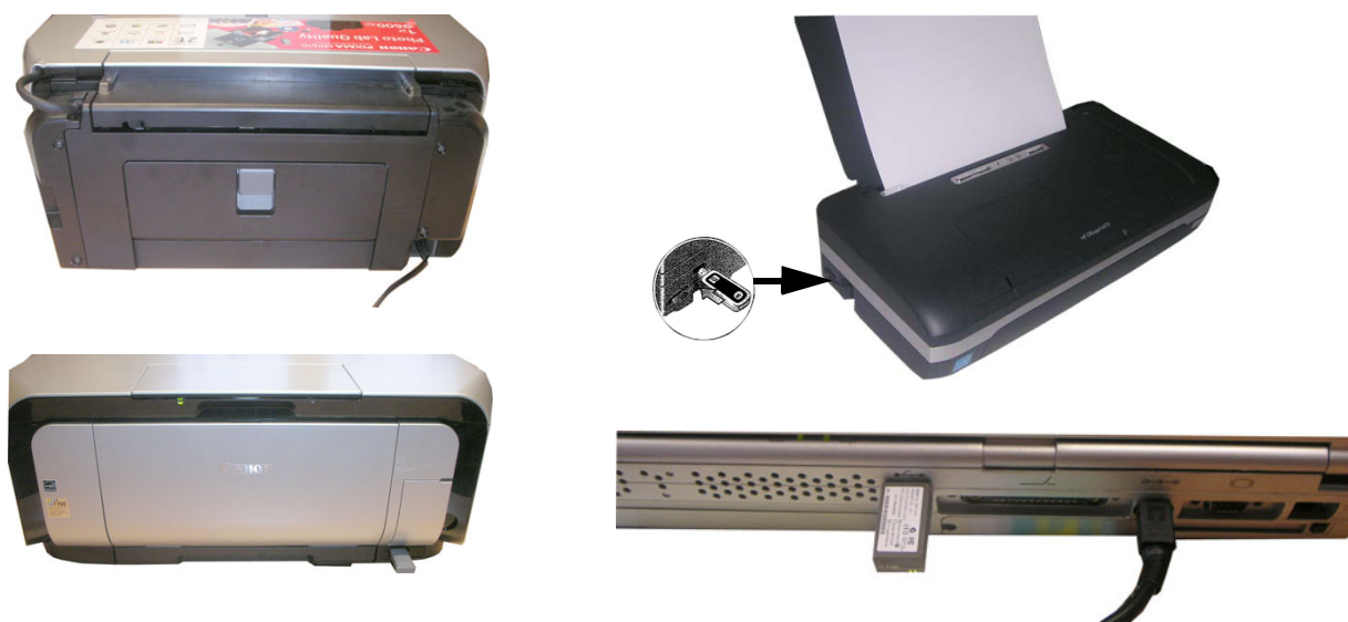
Figure 3-68 Canon Pixma MP600/MP610, MP550 and HP H470 Printer connection (via Bluetooth Adapter)
