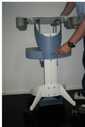
Figure 6-7 lower/raise the shelf assembly, then fasten screws
