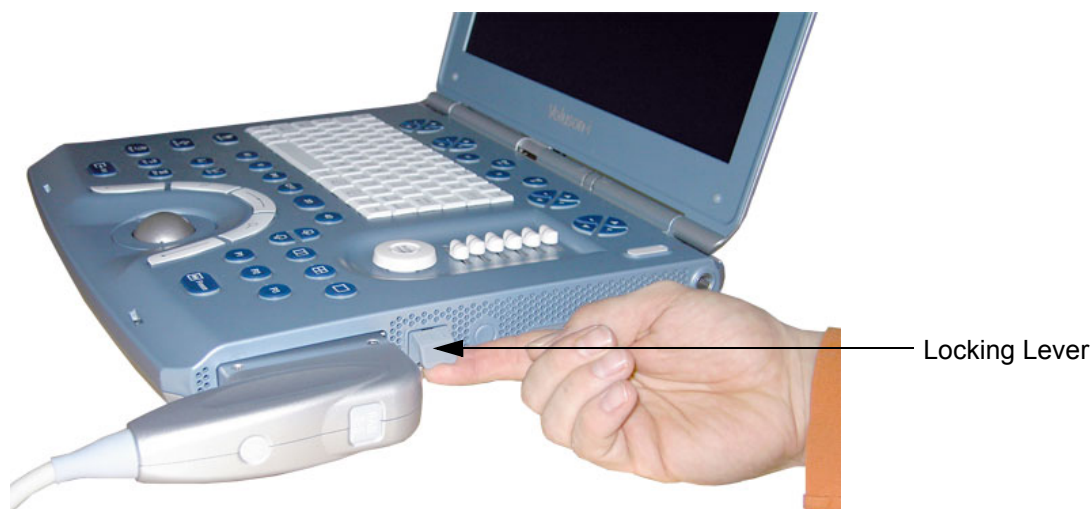
Figure 3-96 Securing probe with Locking Lever
