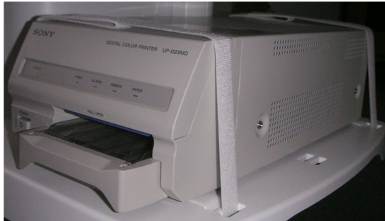
Figure 3-36 pull Velcro tape under shelf and printer and fasten it
