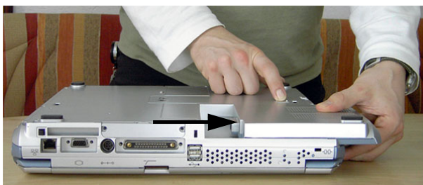
Figure 8-36 Sliding the Battery out of the Battery Compartment
