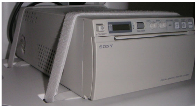
Figure 3-34 pull Velcro tape under shelf and printer and fasten it
