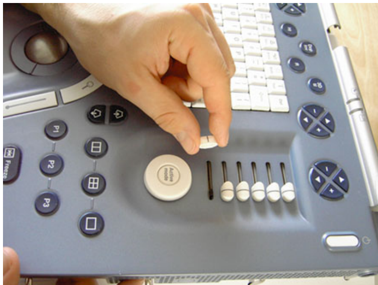
Figure 8-31 TGC Slider Replacement
