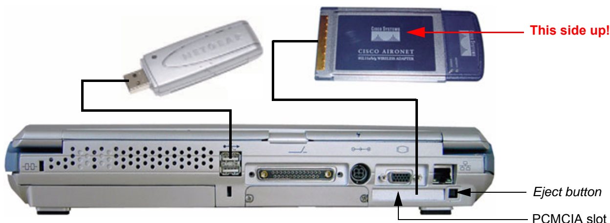
Figure 3-55 Connection Scheme - Wireless CardBus Network Adapter / Wireless Network Interface
