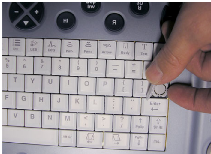
Figure 8-30 Key Cap Replacement
