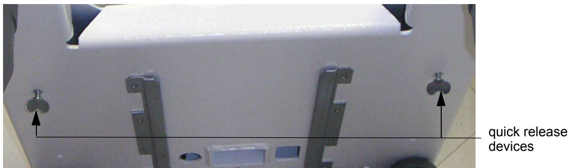
Figure 8-65 turn quick release devices 90°
