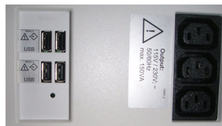
Figure 3-29 Peripherals mounted and secured / Power Supply of Dock Cart / USB-port on Dock Cart
