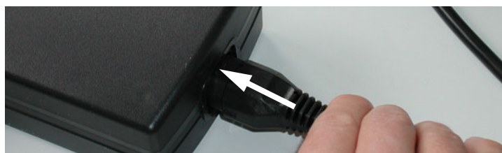
Figure 3-19 AC (main) Adapter connection
