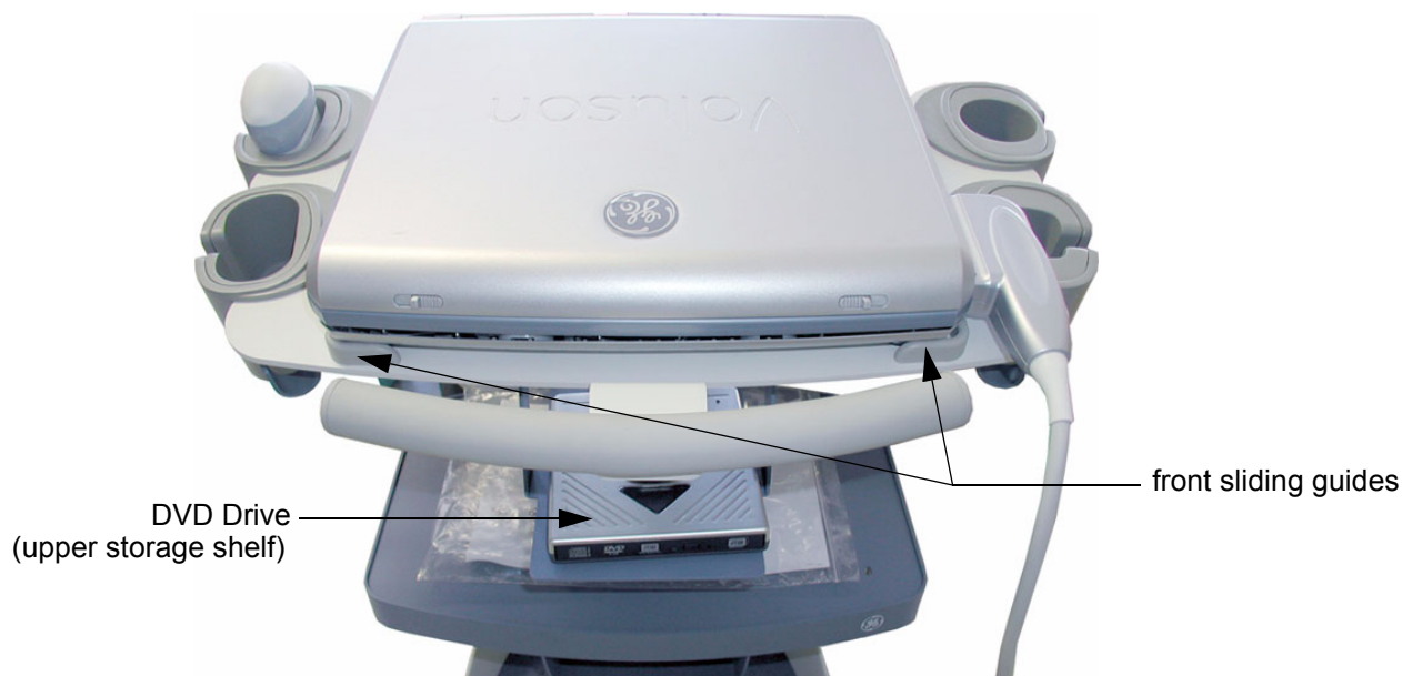
Figure 3-18 Voluson i / Voluson e attached to the Modo Cart
