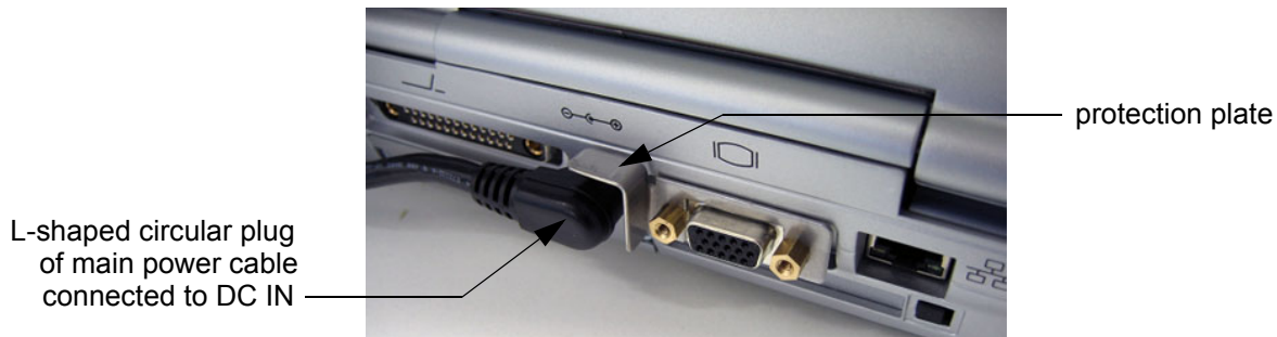
Figure 3-86 main power cable connected to Voluson i / Voluson e
