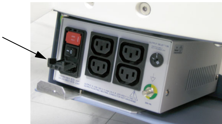
Figure 8-57 open fuse protection on rear of transformer
