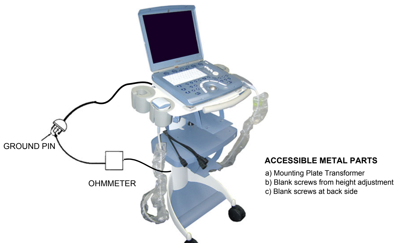
Figure 10-3 Ground Continuity Test
