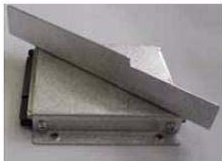
Figure 8-80 Removing the bracket
