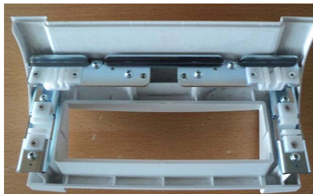
Figure 8-126 Assemble DVD front cover
