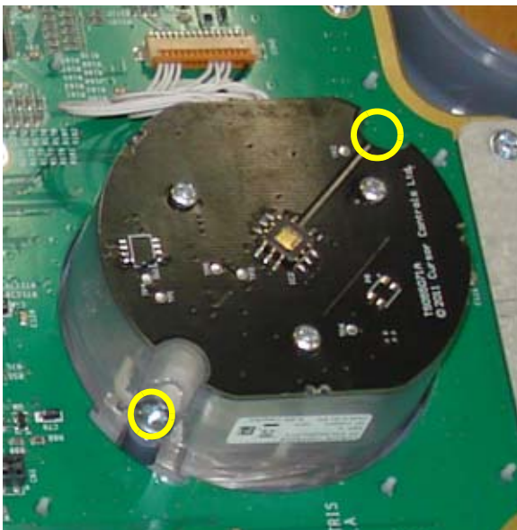
Figure 8-56 Unscrewing 2 screws and pulling out the TRACKBALL
