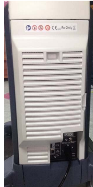
Assemble rear cover, power cord and power cord bracket
