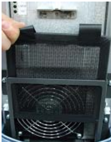
Figure 8-45 Removing the AIR FILTER
