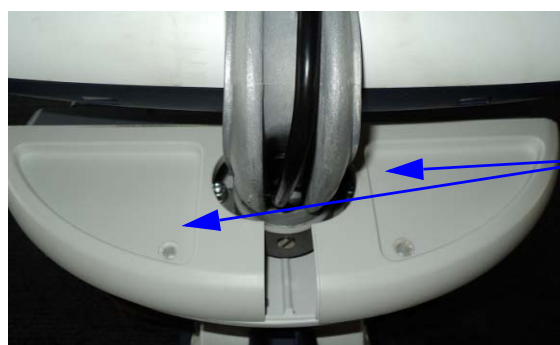
Figure 4-40 Left and right speaker covers
