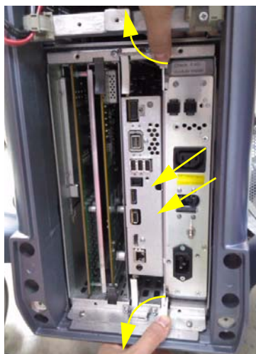
Figure 8-71 Drawing the CPS
