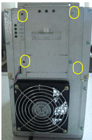
Figure 8-90 Opening the rear bracket
