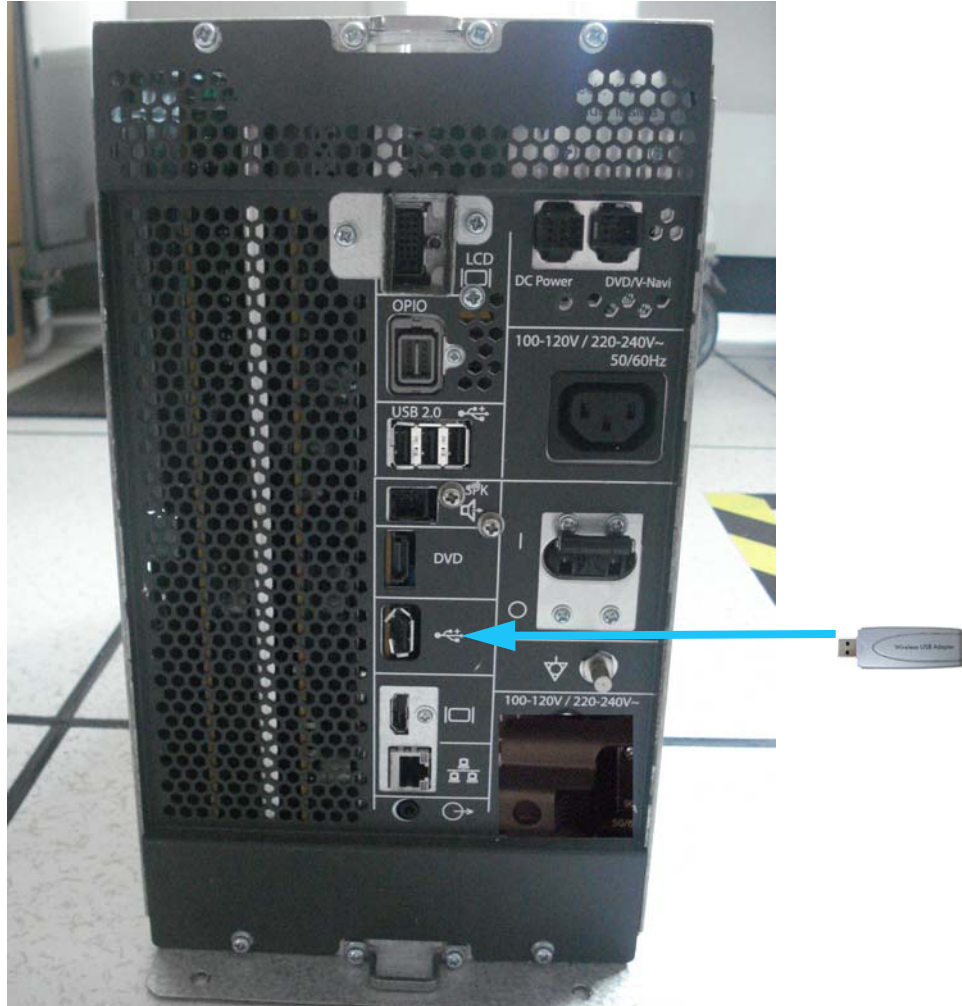
Figure 3-9 Connection Scheme - Wireless (USB) Network Adapter
