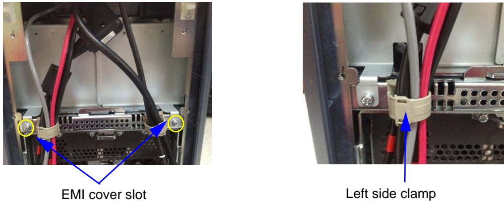
Figure 8-114 Route the printer cables
