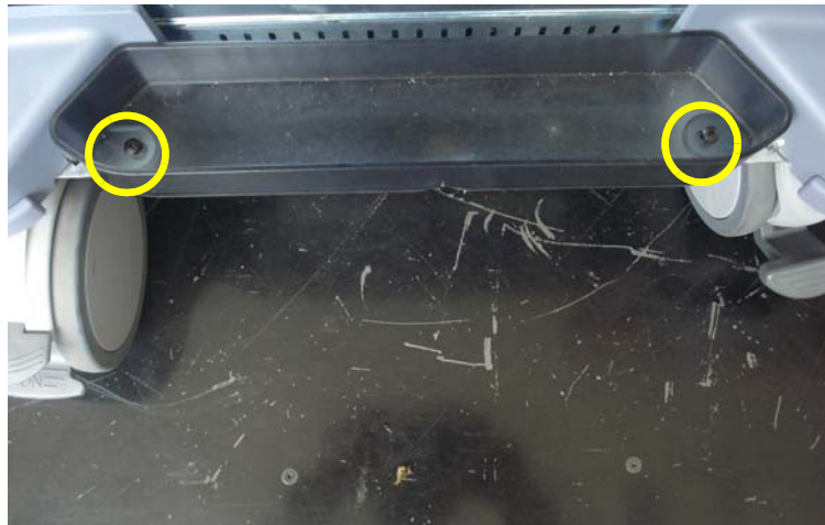
Figure 8-65 Unscrewing 2 screws and remove SIDE TRAY ASSY
