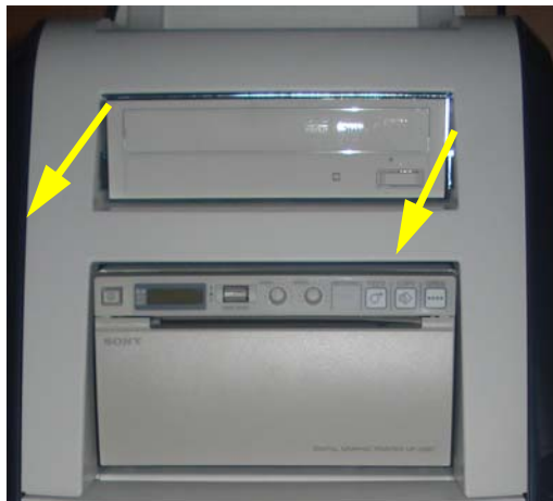
Figure 8-94 Removing FRONT PLASTIC COVER
