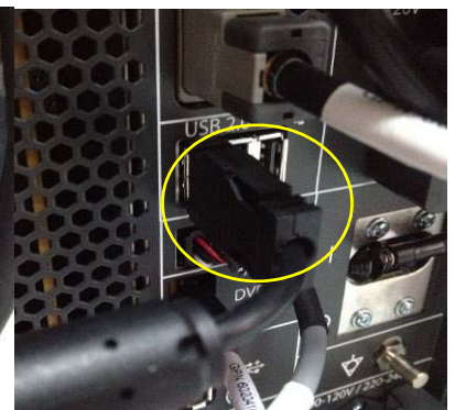
Inserting Printer USB cable into the Nest box
