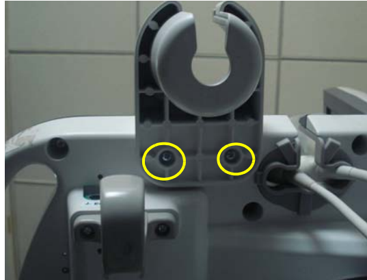
Figure 8-131 Assemble TV PROBE HOLDER BASE with 2 screws (2159634, BH M4x10)
