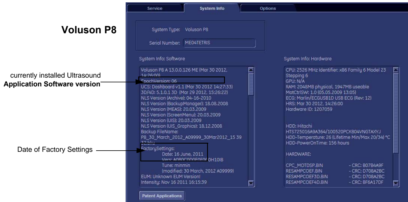
Figure 8-8 Version check (System Setup - Administration - SYSTEM INFO page)
