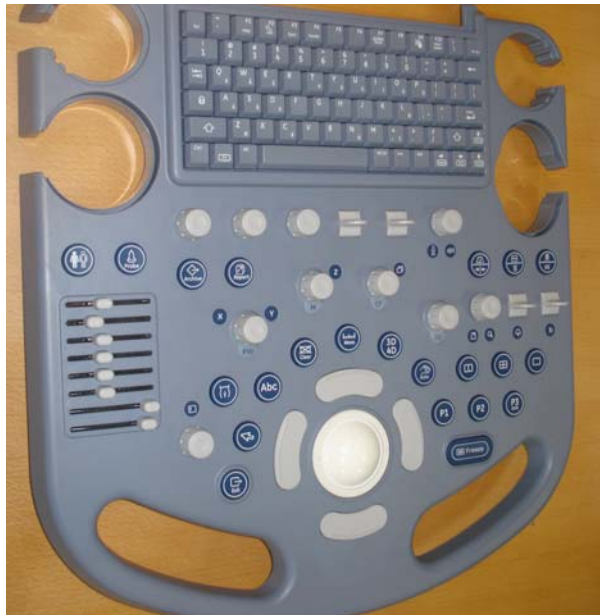
Figure 8-57 Removing 8 TGC KNOBS
