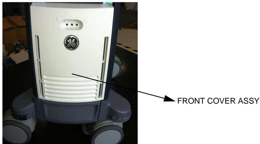
Figure 8-50 Removing the FRONT COVER ASSY
