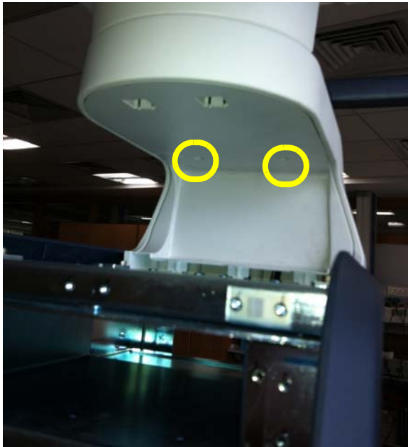
Figure 8-66 Remove REAR COVER ASSY
