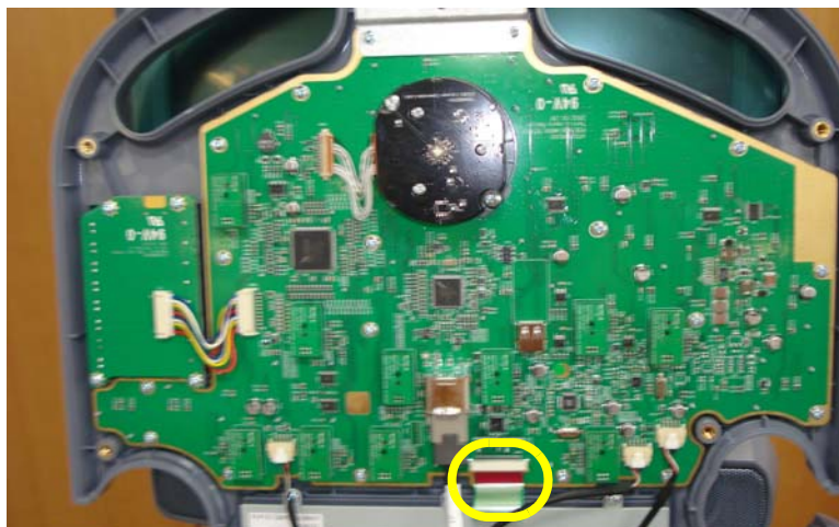
Figure 8-101 Disconnecting 3 cables from OPIO ASSY
