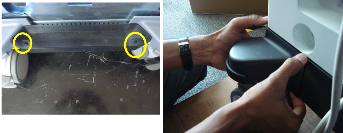
Figure 8-62 Removeing the CASTER CAP
