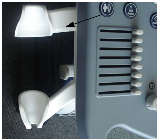
Figure 8-130 HORIZONTAL TV PROBE HOLDER is installed on Left Side only
