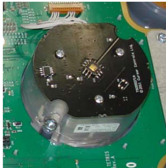
Figure 8-56 Unscrewing 2 screws and pulling out the TRACKBALL
