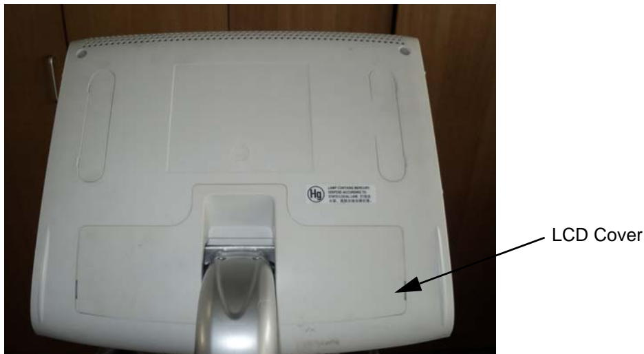
Figure 8-22 Removing the LCD COVER
