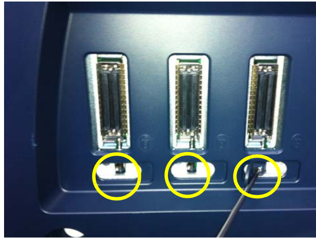
Figure 8-40 Removing the 3 RS KNOBS
