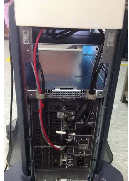
Rear side view after removing the EMI covers 1 and 2
