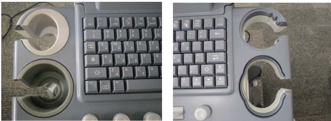
Figure 8-25 Removing the 4 PROBE HOLDERS
