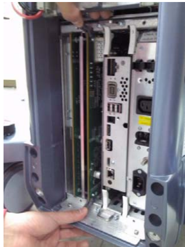
Figure 8-87 Drawing the BF/PIR
