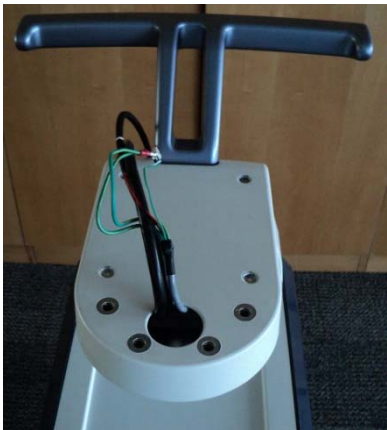
Figure 4-52 Lift the base and pull the cables
