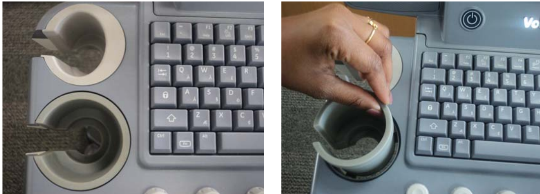
Figure 8-46 Removing the PROBE HOLDER
