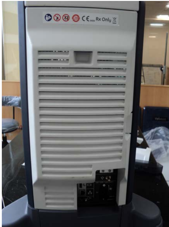
Figure 8-33 Unscrewing 5 screws and Remove REAR COVER ASSY
