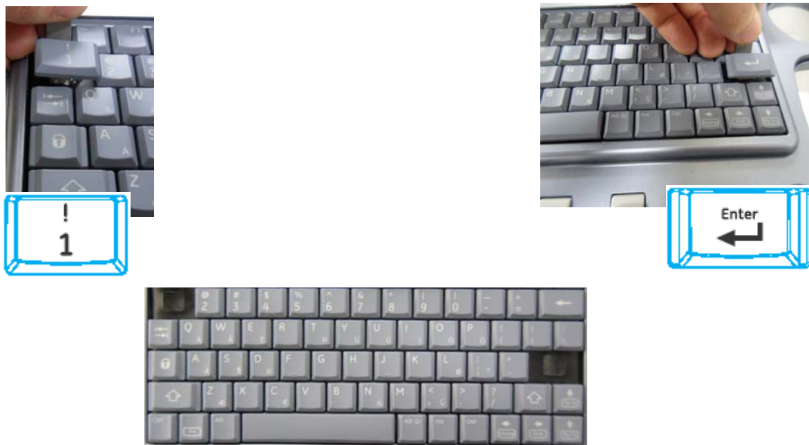
Figure 8-99 removing “1” key and “Enter” key
