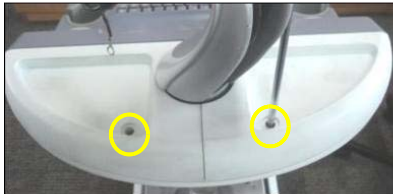
Figure 8-69 Removing the OPIO COVER L, R
