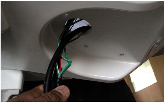
Lift the base and pull the LCD cable, OPIO cable and Speaker cables through the keyboard base hole
