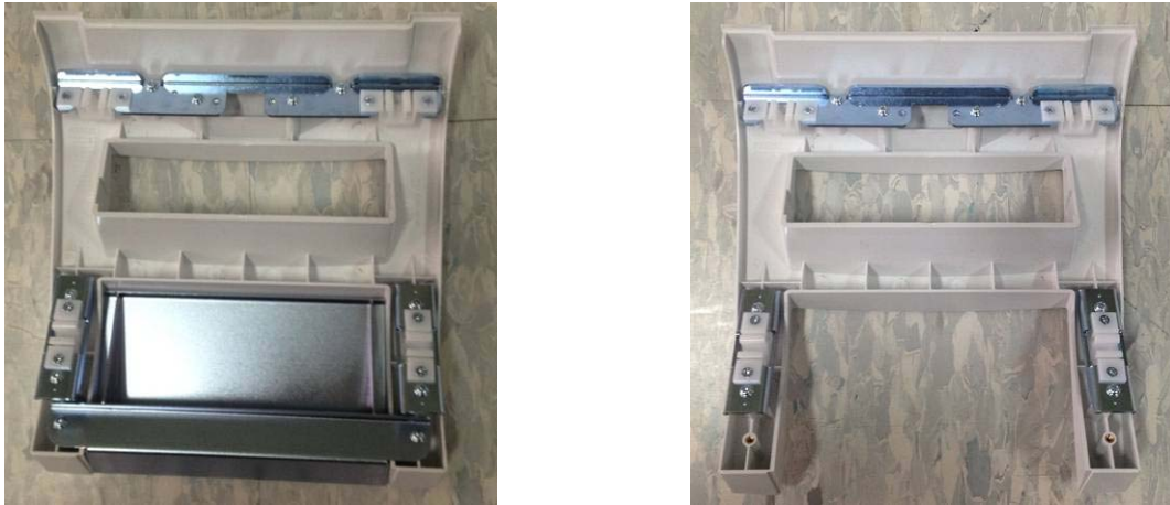
Figure 8-106 Disassemble printer cover
