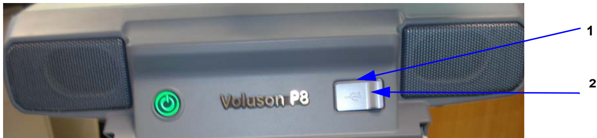
Figure 5-17 External I/O Connectors - on the TOP OPIO
