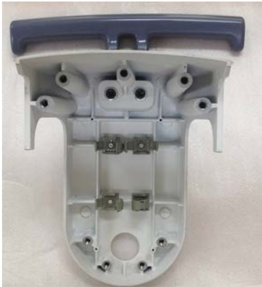
Figure 8-67 Unscrewing 2 screws and remove REAR HANDLE
