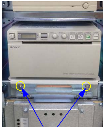
Assemble printer base plate with two screws
