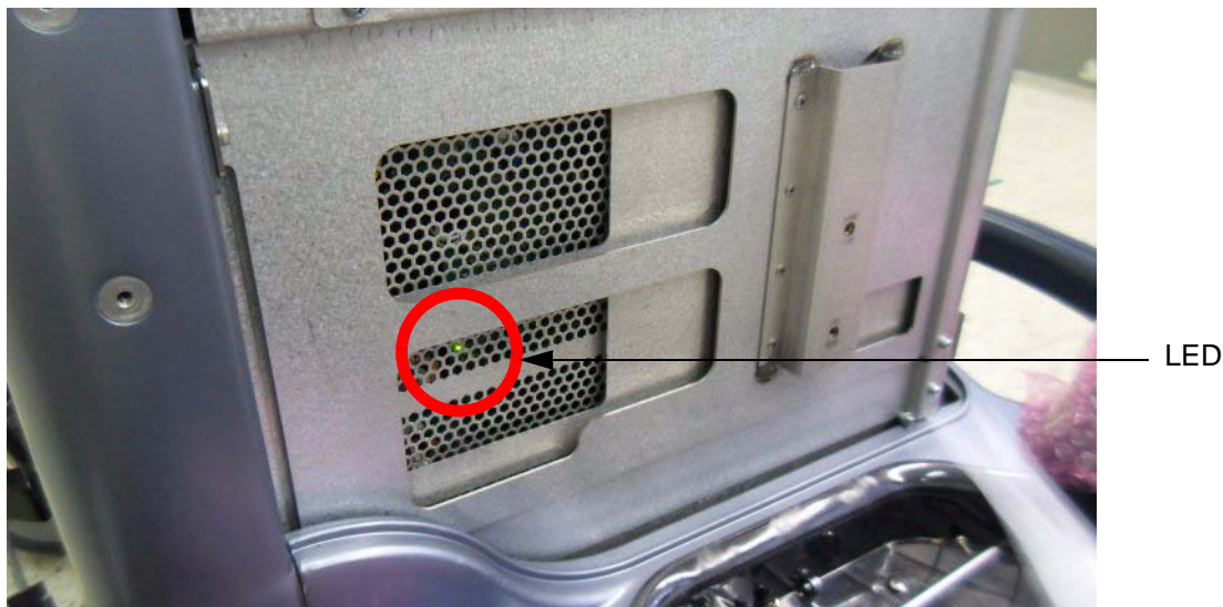
Figure 7-6 Check green LED inside CPS
