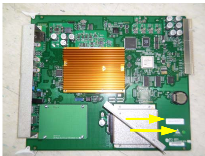
Figure 8-79 Pulling the HDD
