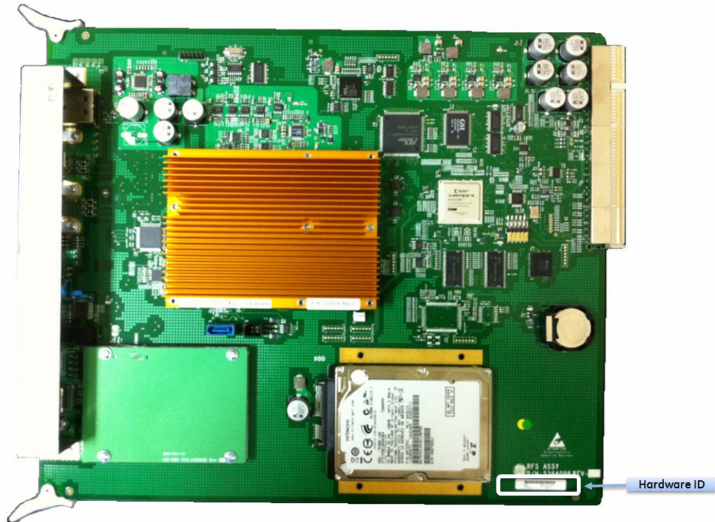
Figure 8-75 Hardware ID on label RFS-board
