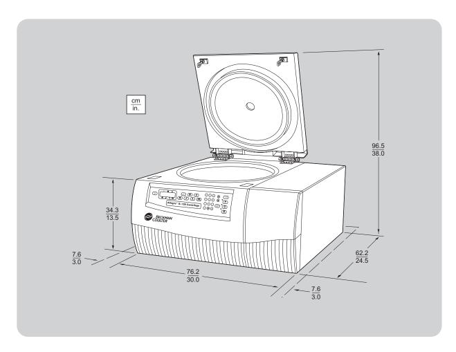
Figure 2-1. Centrifuge Dimensions
