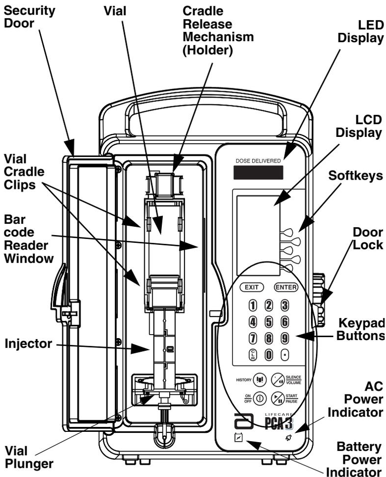
Basic Layout of Front Panel and Keypad
