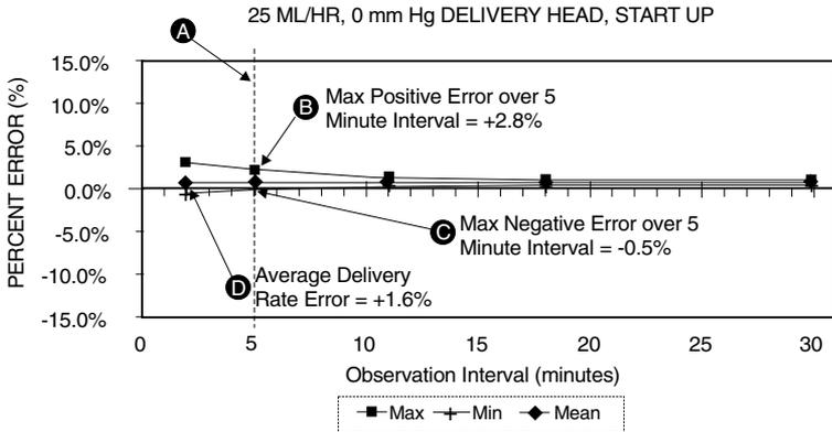
**A trained professional can use the resulting graphs to select a pump with the appropriate startup and flow characteristics to suit the clinical application.**
