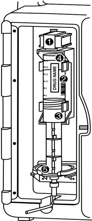
**1. Squeeze Cradle Release Mechanism together at the top of the holder and move to the uppermost position.**
