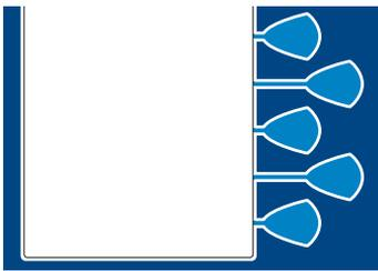
Keys (or Softkeys) are touchkeys which are located to the right of the main display. They perform a variety of functions correlating to the description displayed on the screen.
