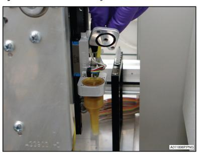
**5** Remove the O-ring (1) from the holding plate.
