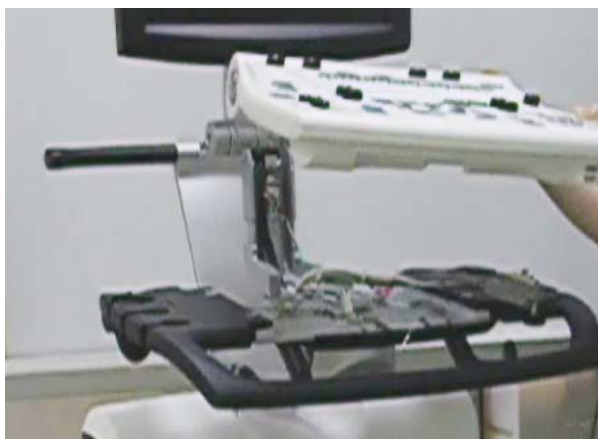
Figure 8-52 Removing the Keyboard Assembly from the System
