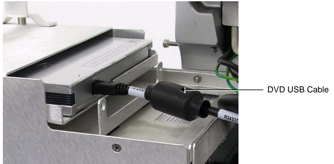
Figure 8-270 Mini USB Cable Connected at Rear of DVD/CD-RW Drive
