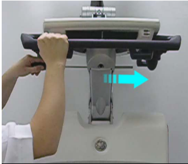
Figure 8-243 Removing Securing Pin from Base of Operator Panel
