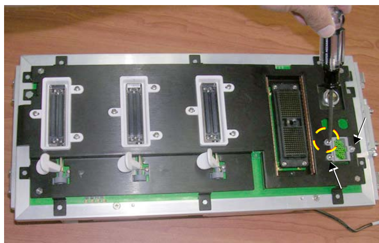
Figure 8-181 Screws Securing ECG Connector to the PSB Board
