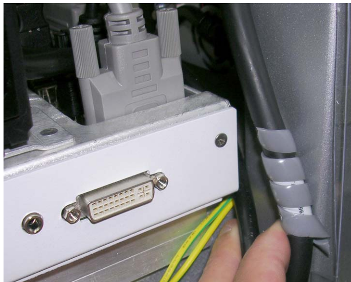
Figure 8-212 Easing Out the Cable from Behind the DIB
