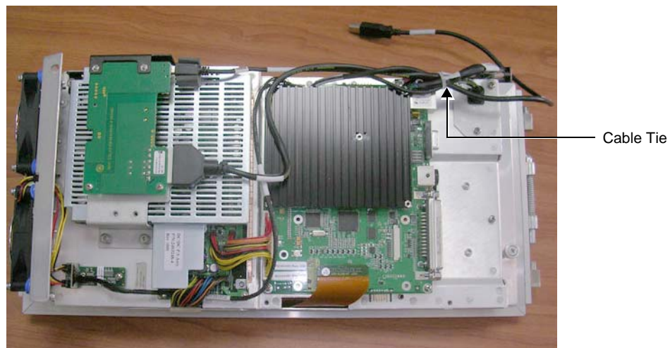
Figure 8-165 Location of Cable Tie
