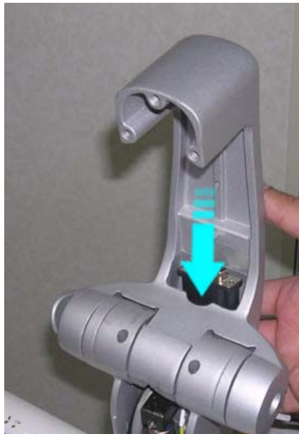
Figure 8-129 Cables Threaded Past Monitor Arm Axis towards LCD
