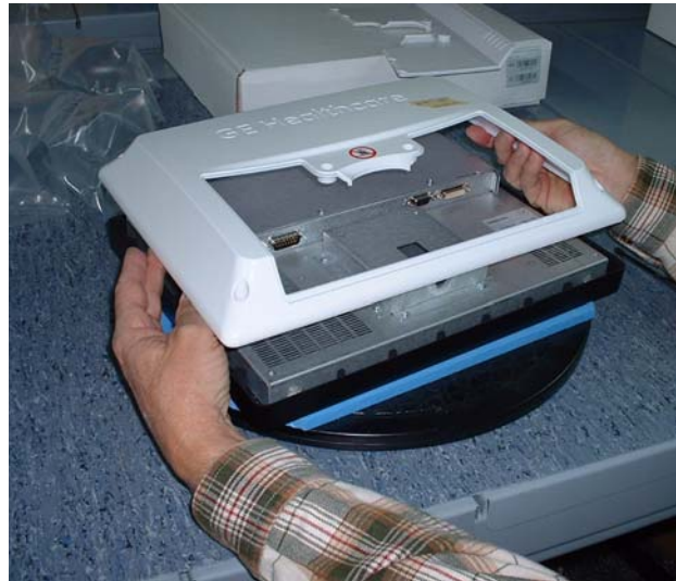
Figure 8-61 Keyboard Interface Assembly Positioned on Joint
