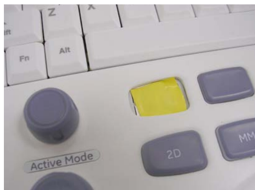
Figure 8-99 Key Hole Covered with Plastic Tape
