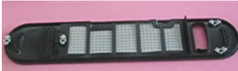
Figure 8-9 Air Filter Fastened in Position on the Left Cover
