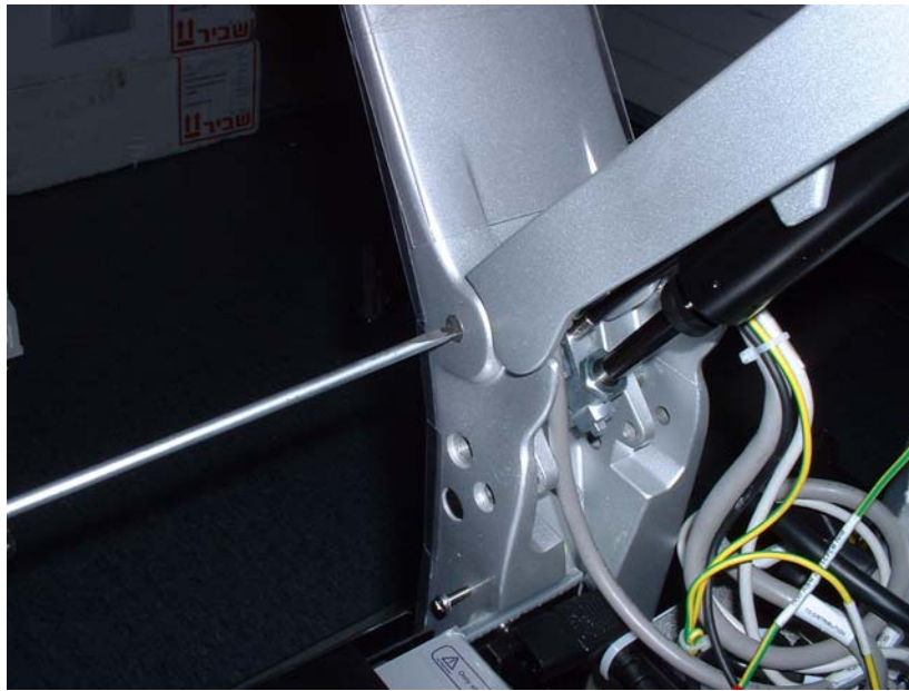
Figure 8-76 Tapping Out the Upper Arm Support Pin
