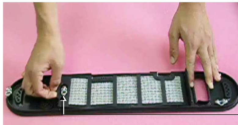
Figure 8-6 Releasing Air Filter Securing Clip
