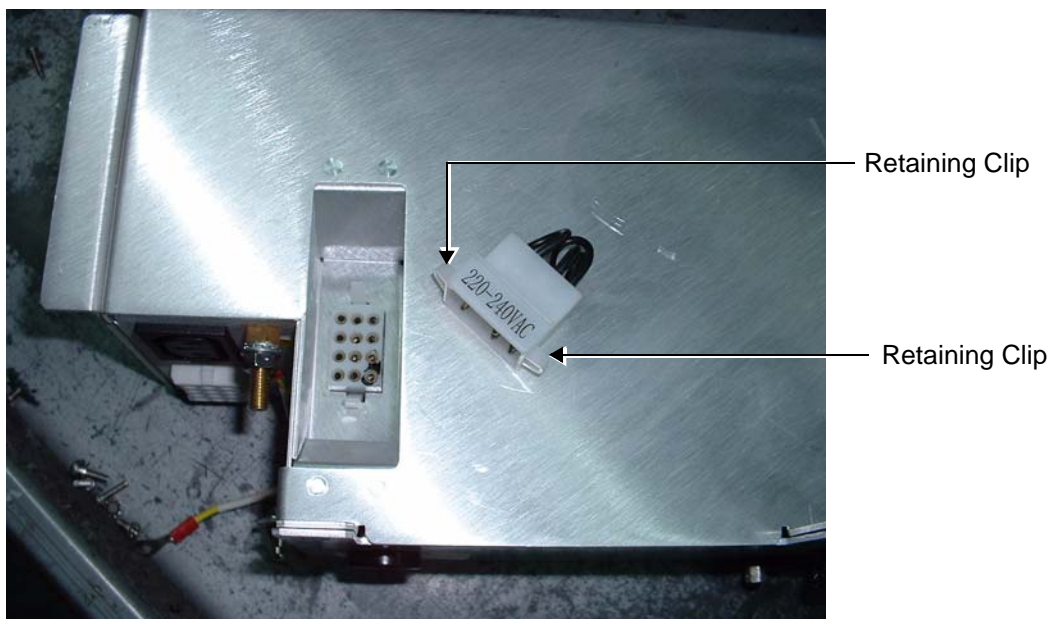
Figure 8-236 AC Box Showing Jumper with Two Retaining Clips
