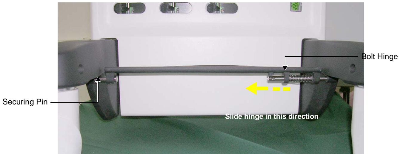
Figure 8-239 Bolt Hinge Securing Foot Rest to Wheelbase
