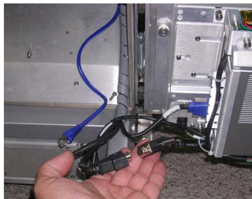
Figure 8-136 Releasing Connectors on the KB Data Cable
