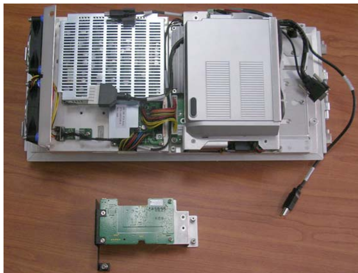
Figure 8-174 ECG Module Assembly Removed
