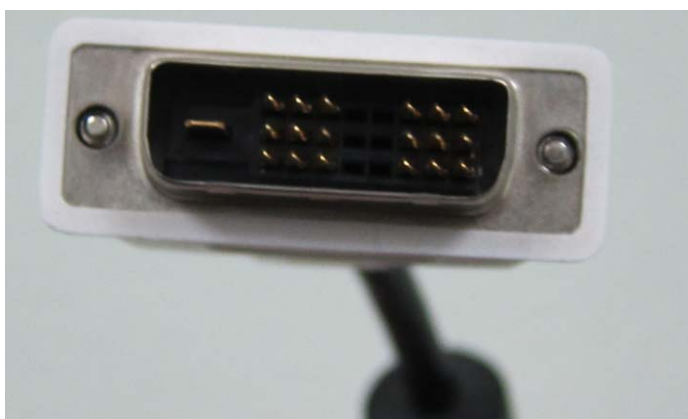
Figure 8-32 Checking DVI Cable Pins
