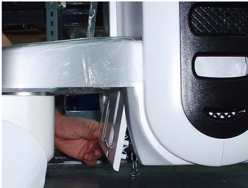
Figure 8-232 Bottom Rear Cover - View from Side
