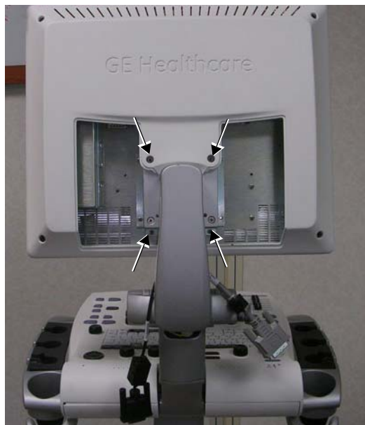
Figure 8-31 Removing the Securing Screws
