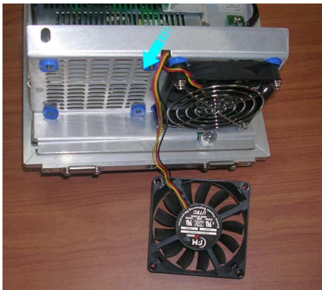
Figure 8-207 Disconnecting the Fan Cable and Removing the Fan
