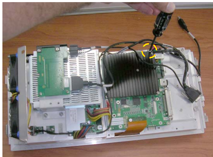
Figure 8-166 Keyboard Cable Fastened with Screw
