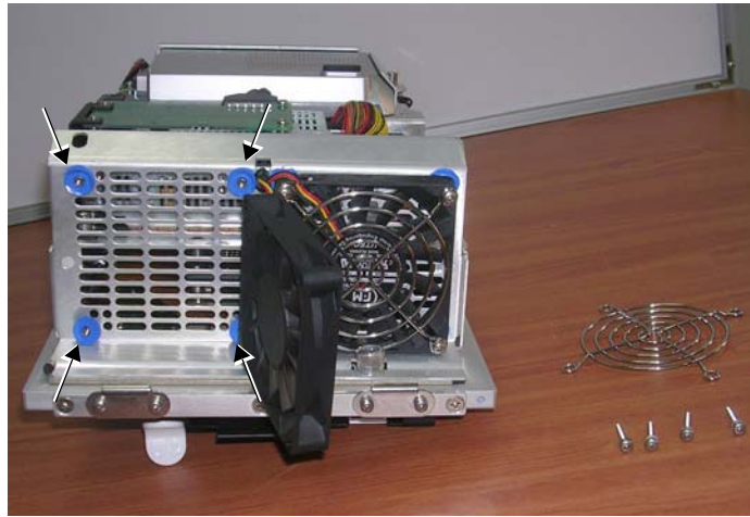
Figure 8-206 Location of Shock Absorbers on Mounting Pins
