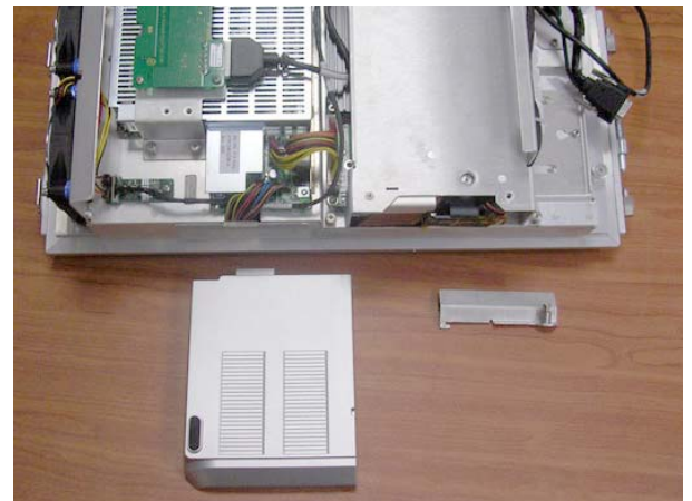
Figure 8-146 Sliding the Vivid S6 N Battery out of the Battery Compartment
