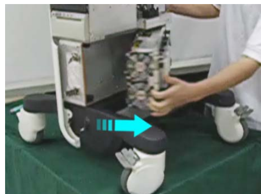
Figure 8-130 Unfastening the Latches and Opening the Cage
