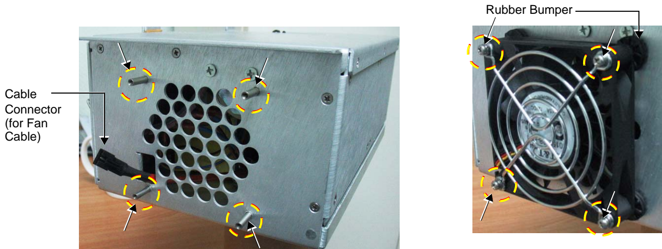
Figure 8-235 AC Distribution Box showing Retaining Pins and Protecting Grid
