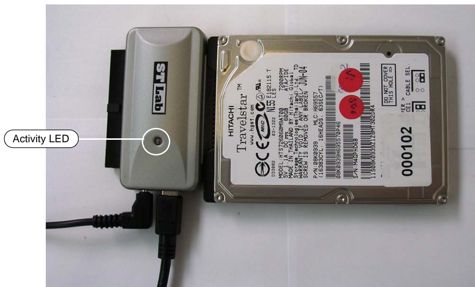
Figure 8-158 PATA Hard Disk Connected to the USB-to-SATA/PATA Adaptor
