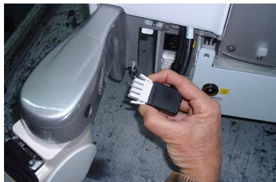
Figure 8-230 Plastic Securing Clips on Power Cables
