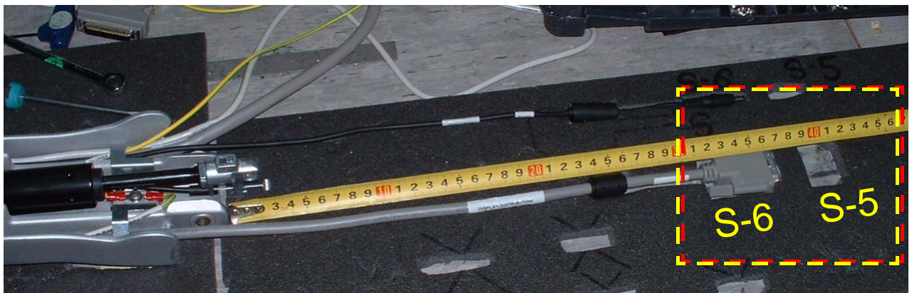
Figure 8-78 Protrusion of Vivid S5 N and Vivid S6 N Cables (42 cm and 37 cm, respectively)
