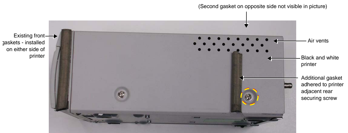
Figure 8-288 B&W Printer showing the Additional Gasket Adhered
