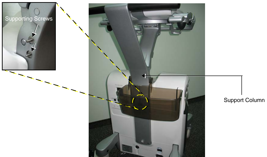
Figure 8-22 Folder Box Installed on Vivid S5 N / Vivid S6 N Support Column
