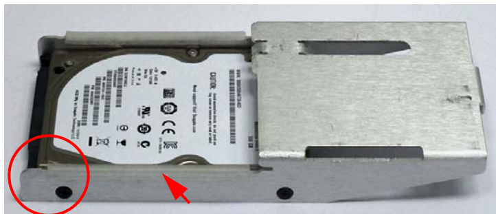
Vivid S5/S6 hard disk showing plastic buffer (indicated by arrow) position
