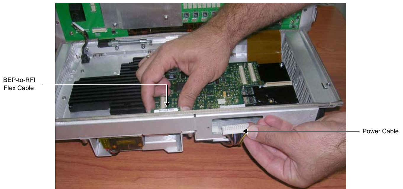
Figure 8-193 Disconnecting the Cables from the RFI Board
