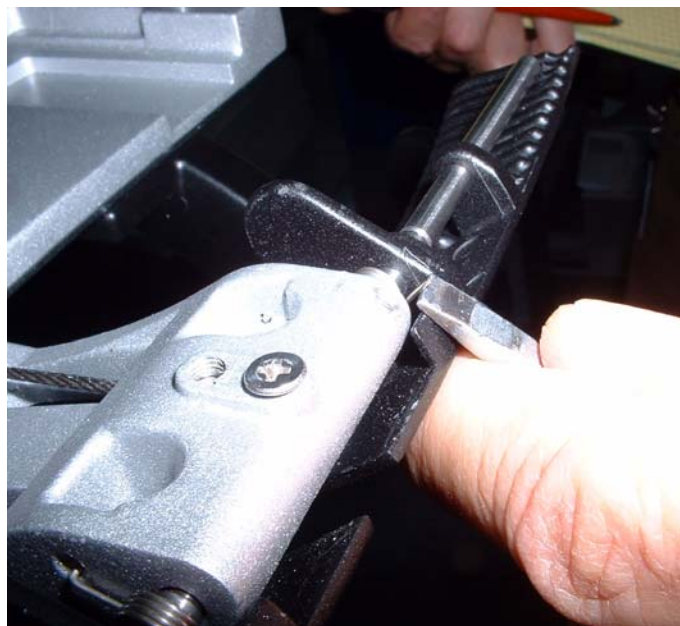
Figure 8-68 Releasing Spring that Presses on the Handle
