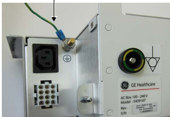
Figure 8-231 Ground Lead Showing Spring Washers and Cable Holder
