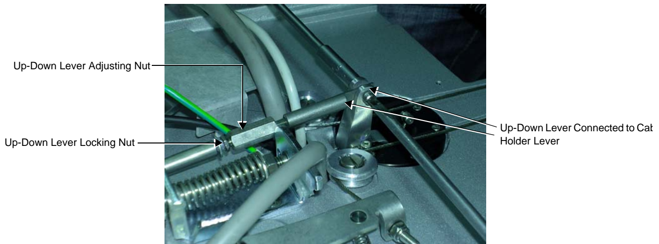
Figure 8-64 Up-Down Lever Connected to Cable Holder Lever
