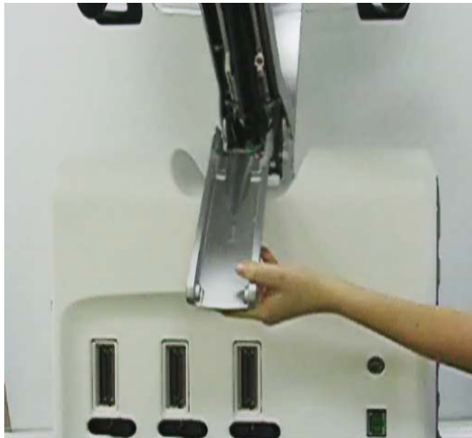
Figure 8-247 Removing the Lower Arm
