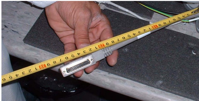
Figure 8-77 Vivid S5 N Monitor Cable Protrudes 27.5 cm from End of Upper Arm
