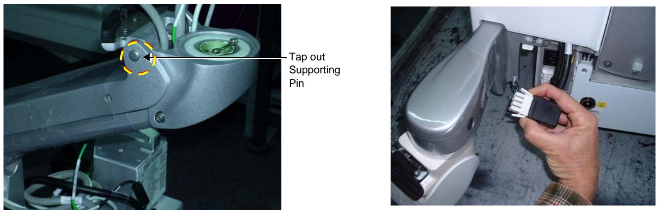
Figure 8-83 Removing the Joint Assembly
