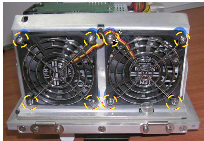
Figure 8-205 Fan Assembly Securing Screws
