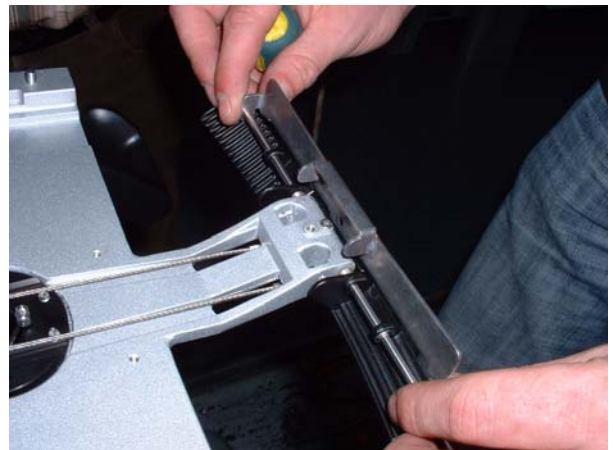
Figure 8-66 Protective Metal Plate Rotated 90 Degrees
