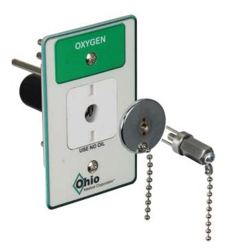
the internal primary check valve, located in the latch valve assembly. The locking kit consists of a chrome plated locking cap which plugs into the Ohmeda outlet. Inserting and turning the key will pop off the lock and allow flow of the gas. Part Numbers: 261639 Ohmeda Locking Kit (all gases) 261640 Key for Ohmeda Locking Kit
