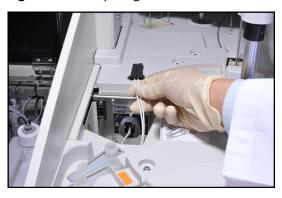
**6** Remove the lamp by turning the lamp holder counterclockwise, then pulling the lamp from the lamp receptacle. Handle the lamp by the lead wires.
