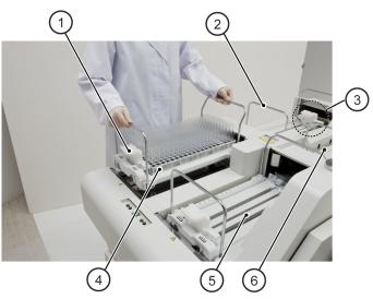
Figure 4.10 Placing a Rack Input Tray or Rack Output Tray
