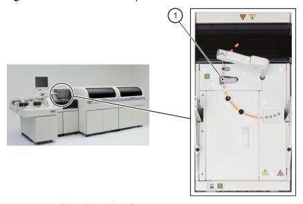
1. ISE sample probe wash solution set position
