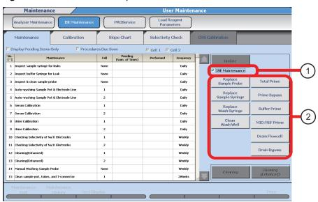
Figure 6.7 ISE Maintenance Operation Buttons
