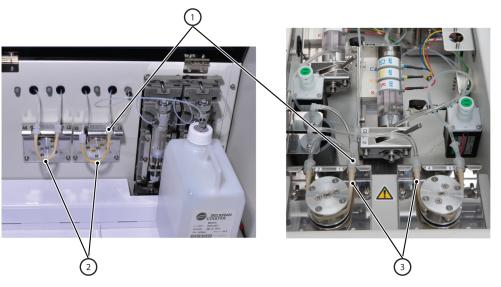
Figure 6.113 Mixture Aspiration and MID Standard Roller Pump Tubing
