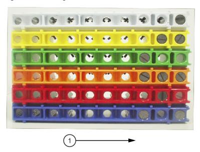
1. Magnets in rack positions 1, 2, or 3 (to the right of the arrow)
