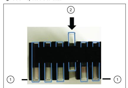
Figure 6.84 Replace the Cuvettes
