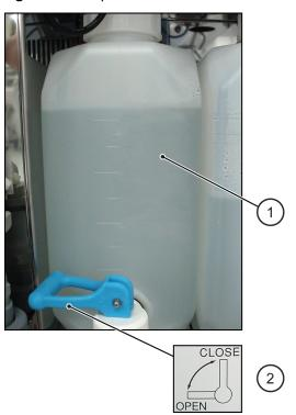
Figure 2.16 Inspect the Handle on the Diluted Wash Solution Tank in the Analyzer Unit
