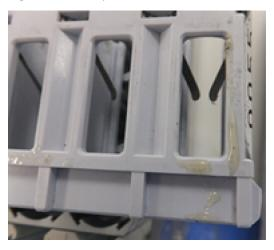
If the rack ID label is peeling, it can also cause a rack jam. Replace the rack ID label. Refer to Replace Rack ID Labels.
