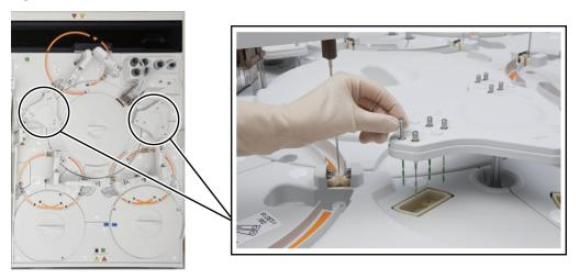
**4** Insert a new mix bar into the mix bar component.
