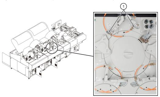
1. Sample probe wash solution set position
