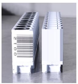
**2** Attach a new rack ID label on the rack. Place the label on the beveled edge of the rack with the numbers on the left (when looking at the rack).
