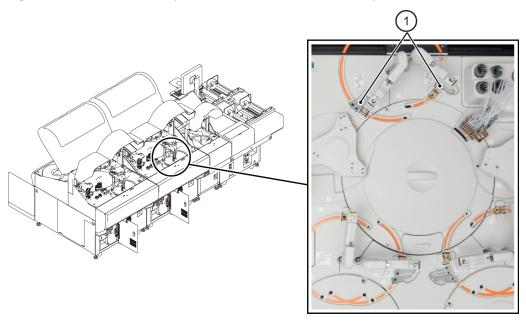
1. Sample probe wash solution set position
