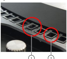
Figure 9.4 Incorrect and Correct Cuvette Placement
