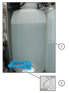
Figure 6.19 Inspect the Handle on the Diluted Wash Solution Tank in the Analyzer Unit
