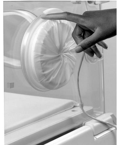
4. Check the access door latches and gaskets.
