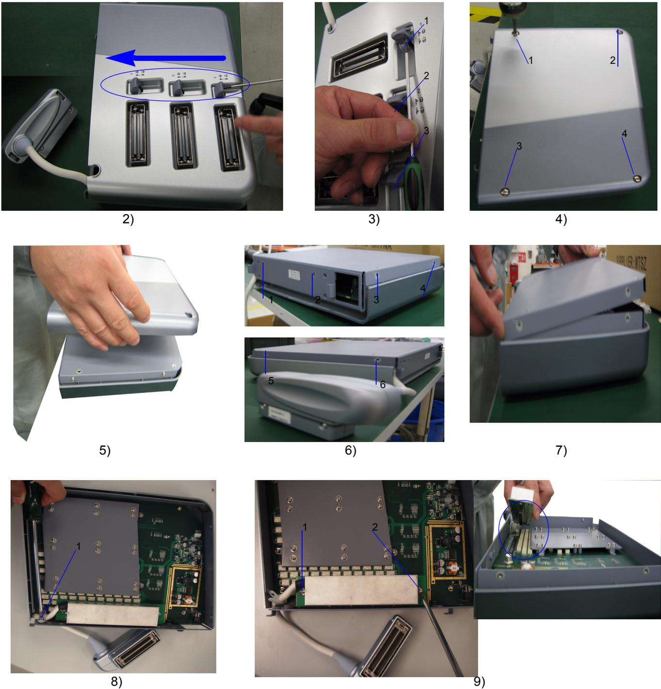
Figure 8-12 Three-probe PWA Disassembly
