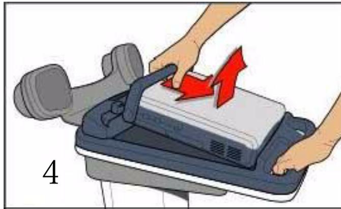
**Figure 4-58** Lift up the system from cart
