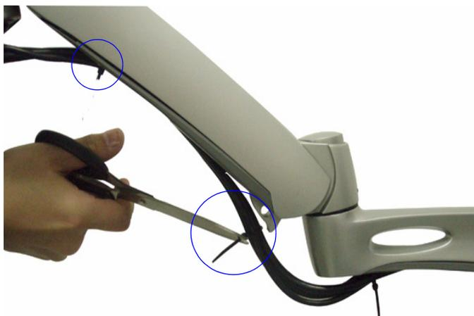
Figure 3-14 Cut the cable tie
