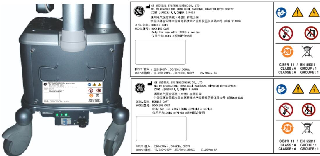
Figure 1-4 Docking Cart Identification and Rating Plate (for 220V-240V AC)
