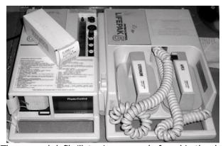
The manual defibrillator is commonly found in the developing world. The unit on the left includes an ECG monitor. The device delivers a potentially lethal shock and should be worked on with great care.
