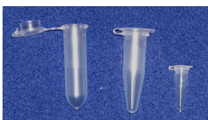
Three microcentrifuge tubes: 2 mL, 1.5 mL and 200 µL (for PCR).
