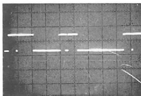
Deflection Board U1C, Pin 8, 2 msec, 20 Volts/Div.
