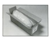
c. Stretch the resin pack over your arm to elongate the pack, and feed it into the Silex column allowing the pack to slide out of the plastic sleeve.
