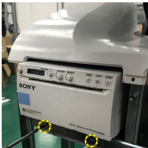
Figure 3-27. Push the printer assembly
