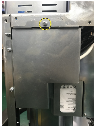
Figure 3-39. Remove the metal sheet
