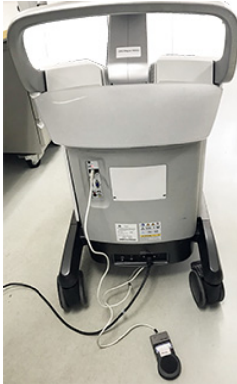
Figure 3-30. Connect Footswitch to the system (2)
