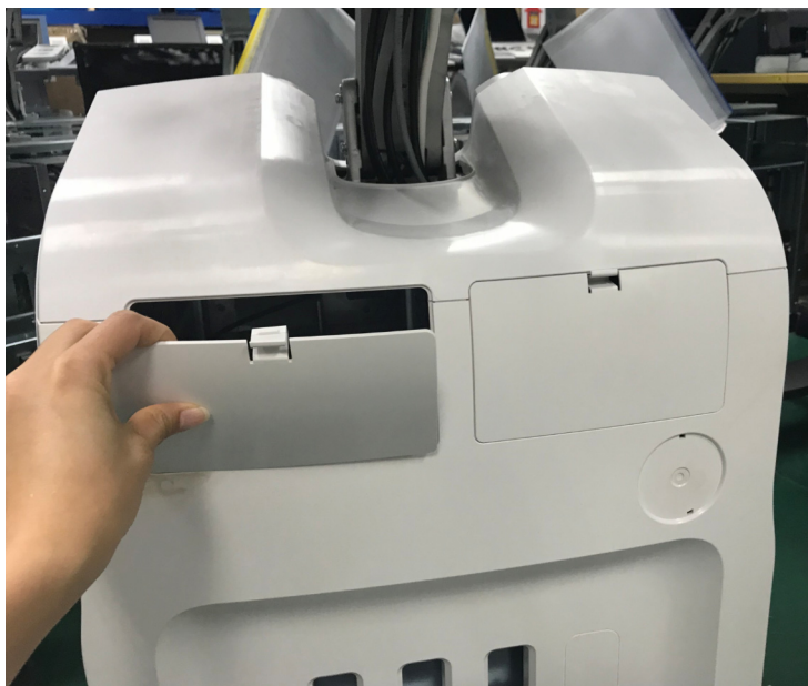
Figure 3-9. Remove printer and ECG cover
