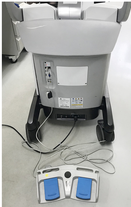
Figure 3-29. Connect Footswitch to the system (1)
