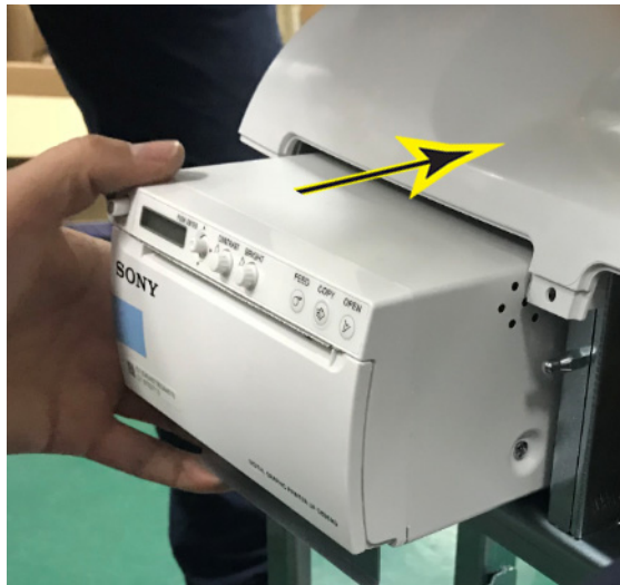
Figure 3-12. Insert AC printer
