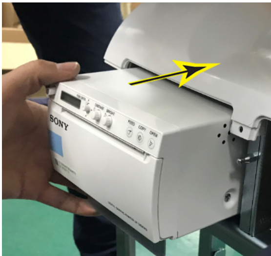
Figure 3-26. Insert DC printer
