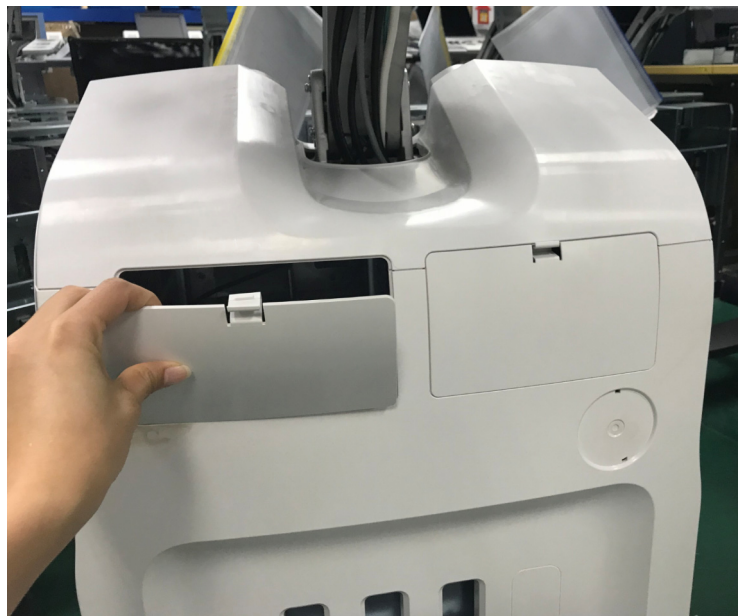
Figure 3-36. Remove printer and ECG cover
