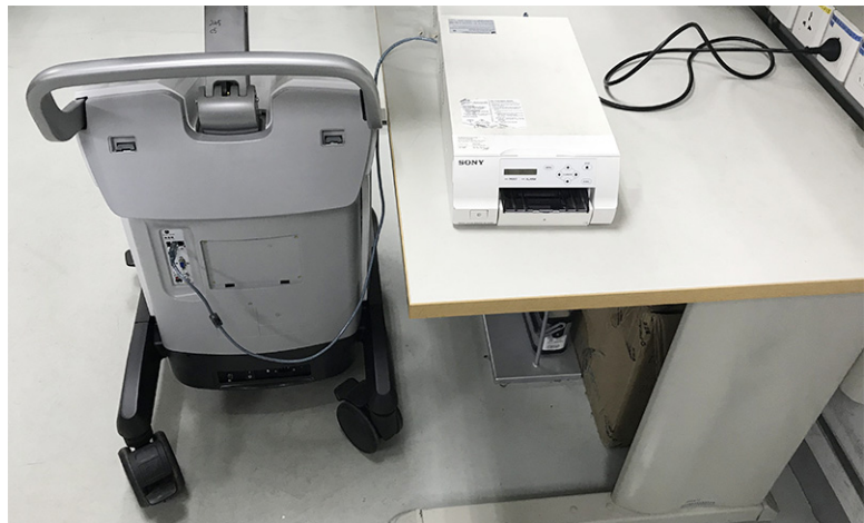
Figure 3-28. Color Printer connection
