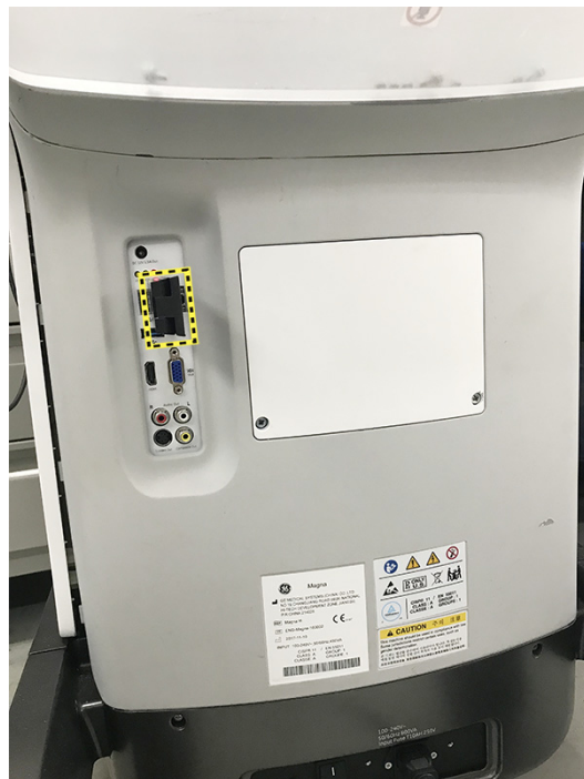
Figure 3-41. Connect Wireless Adapter
