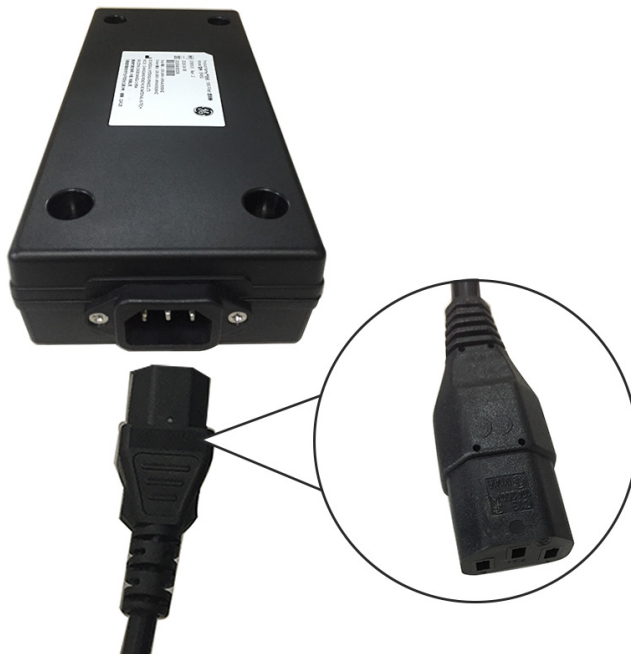
Figure 3-52. Insert the system power cord into the EMI filter input side
