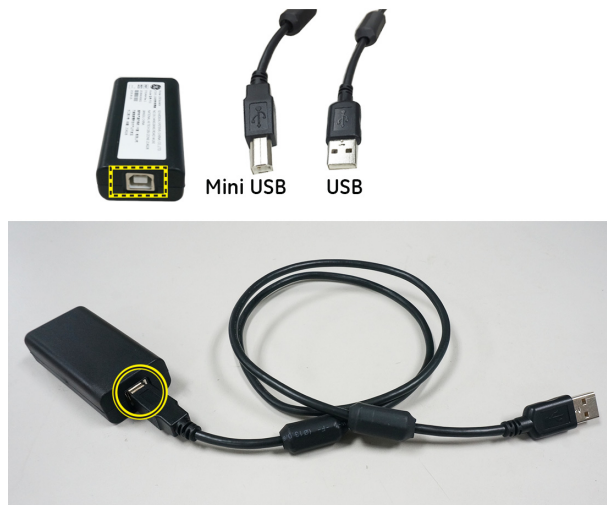
Figure 3-48. Insert the USB connector into Printer USB Isolator
