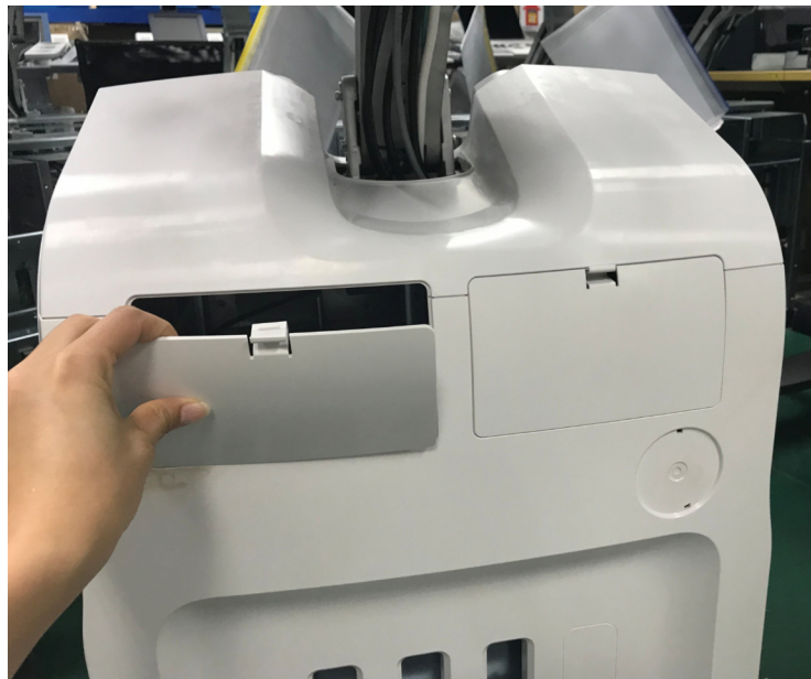
Figure 3-22. Remove printer and ECG cover
