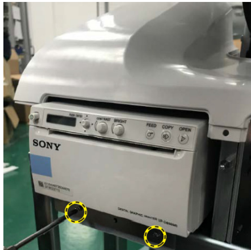
Figure 3-13. Push the printer assembly
