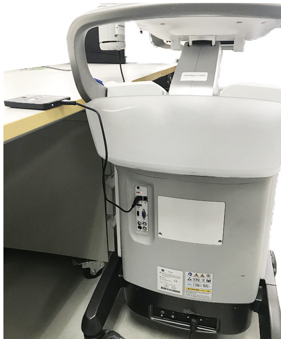
Figure 3-32. Connect HDD to the system
