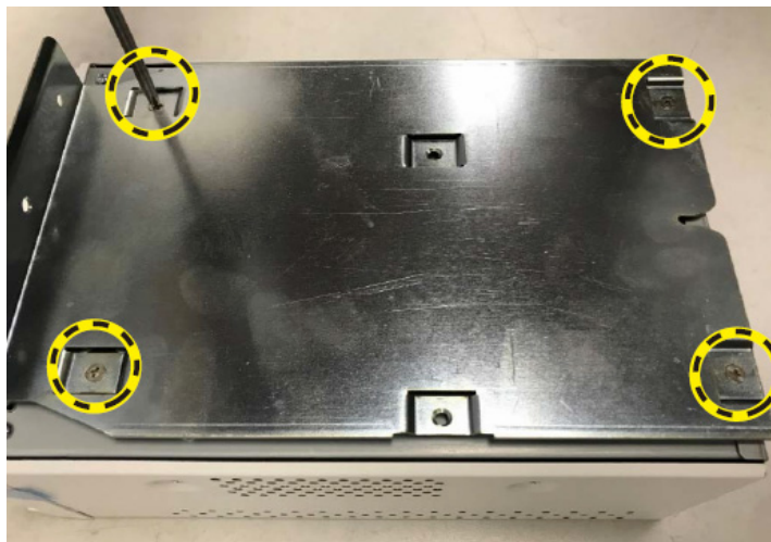
Figure 3-7. Install printer to printer shelf
