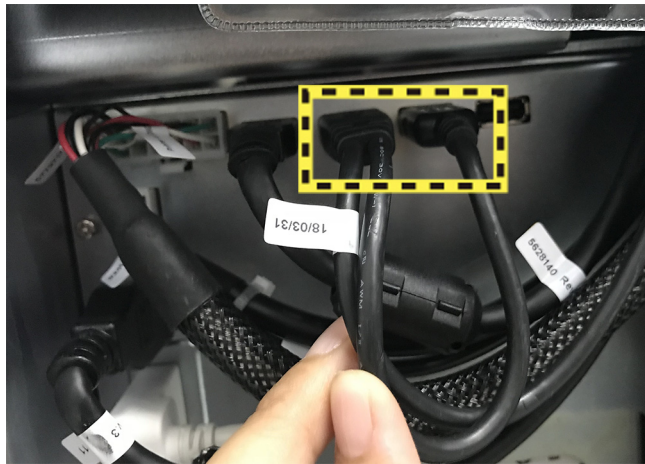
Figure 3-40. Connect both of the DVD USB cables
