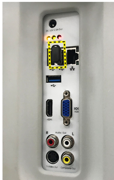
Figure 3-42. Connect Bluetooth Adapter
